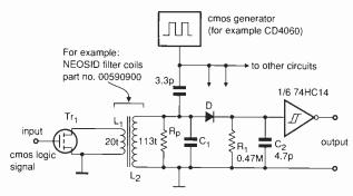
Fig. 1. While providing effective logic isolation, this inductive circuit consumes about 2000× less power than an opto-isolator.
