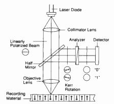
In a magneto-optical rewritable disk, polarity of the magnetic bit region can only be changed while the area is heated by a laser.
