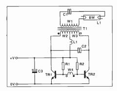
Fig. 5. Emergency fluorescent lamp controller runs from 2.4 or 4V. Low operating voltage results in fewer power cells, reduced volume and lower cost.
