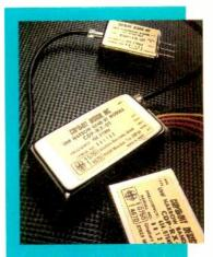
Narrowband radio modules. A matched transmitter/receiver pair by Circuit Design for the pan-European ETS-300-220 frequency of 434MHz is a now available. CDP-TX-01 is a narrowband transmitter using a crystal oscillator with a ±4ppm stability and direct fsk modulation to allow 12.5kHz channel spacing.The CDP-RX-01 receiver is a crystal-controlled double superhet with 120dBm sensitivity and ±5kHz selectivity. Low Power Radio Solutions Ltd. Tel., 0993 709418; fax 0993 708575.
