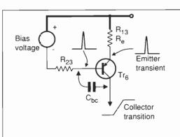
Fig. 6. One reason why simple theory fails. Fast positive edges on the collector of the voltage amplifier source  $Tr_6$  couple through the internal  $C_{bc}$  to momentarily reduce standing current.
