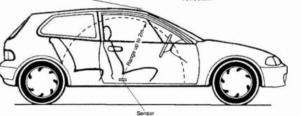
Adequate gain is available by adjusting a sensitivity control potentiometer to give a minimum of two metres coverage range when the sensor is mounted as described. Metal objects in close proximity to the sensor may distort the beam pattern and lead to areas of poor coverage. Moving the sensor slightly can overcome this.
