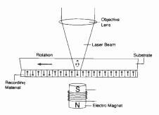
temperature however, polarity of a magnetic domain can be easily changed by an external magnetic field. Wherever a data bit is to be recorded, a high powered laser beam is used to heat the material above this temperature, allowing this reversal to take place.
