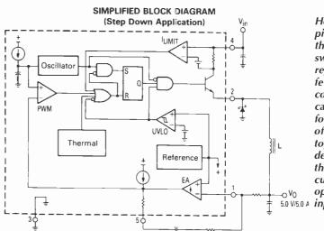
Housed in a fivepinned flat pack, the MC34167 switching regulator needs few external components yet can be configured for a wide range of DC converter topologies. It delivers more than 5A switch current and operates from 5.0 V/5.0 A inputs to 40V.
