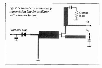
in fact, shunted by the junction resistance but, as this is very large  $(10M\Omega)$  under reverse bias, it has little effect. When designing an oscillator, if  $C_j$  is made to be all or part of the tuned circuit, then changing the reverse bias voltage will change the resonant frequency of operation.
