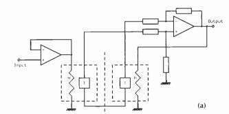
Fig. 1a). Deriving the rms value of a signal using two heatersensor combinations. A DC voltage applied to a resistor produces exactly the same amount of heat as its equivalent in rms. b). Dynamic range of the thermal converter is improved by adding analogue divider.
