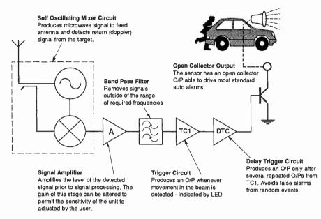
This Doppler radar module, built into a bolt-on box, provides an output compatible with existing alarm systems and is easily retrofitted.
