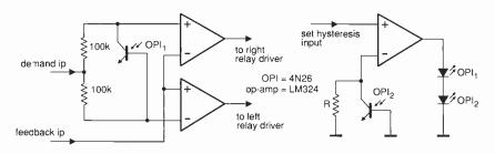
Servo, originally used to control steering on a small vehicle, uses opto-isolators to provide a floating hysteresis voltage to define dead zone.
