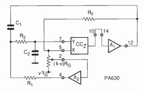
Fig. 1. Current-feedback amplifier circuit allows independent control of amplitude and frequency.
