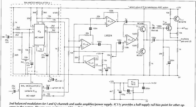
amps in the system. The pre-amp sections would benefit from a lower noise device in place of the LM324 used in the prototype.
