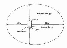
Because it is unlikely that the Doppler radar module will be mounted exactly in the middle of the car, its effective area is asymmetrical. Although proportions of the area covered are fixed, the size of the area is adjustable by simply turning a screw.
