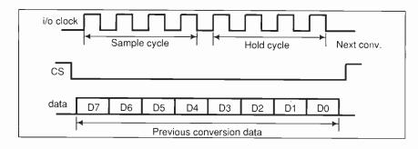
procedure eight times. Finally the chip-select line is brought high and the converted data returned in the AL register.
