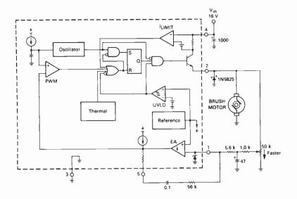
current limiting, undervoltage lockout, and thermal shutdown. Also included is a low power standby mode that reduces power supply current to  $36\mu$  A.
