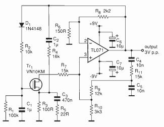
Spot-frequency Wien-bridge oscillator uses a mosfet instead of a thermistor for amplitude control, while retaining a THD of about 0.02%. A common method of stabilising a Wien-bridge oscillator is to use a thermistor, which is expensive. This 1kHz spot-frequency oscillator uses a mosfet to do the same job, with low distortion.
