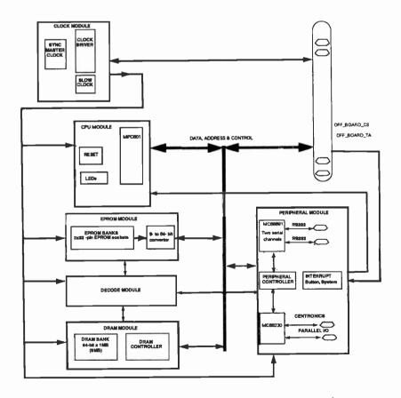
Elements of an evaluation system for Motorola's new PowerPC chip. Within the note describing this system are full details including software drivers and pcb layouts.
