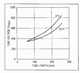
Fig. 9. Running voltage against lamp length at two temperatures. Start-up voltages are usually 50 to 200% higher over temperature.
