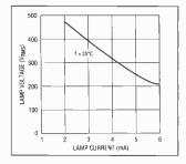
Fig. 8. Current versus voltage for a lamp in its operating region.
