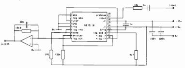
Fig. 9. Versatile converter chip configured for log of rms conversion. This configuration is useful for audio decibel metering.
