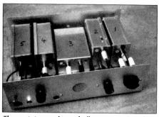
The prototype unit was built up as a series of modules wired together. This achieves a high level of screening, important even to basic direct conversion equipment.
