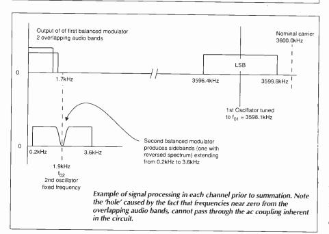
the middle of any subsequent reconstitution of the original modulation frequency range. Also, one of the signals has a reversed frequency spectrum compared to the original modulation.
