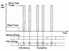
Unrecorded, the active layer in worm media is amorphous and absorbs light. Recording involves changing the phase of a data area by crystallising it using heat from a laser. This results in light absorbing and reflecting areas: each represents a logic level. amorphous areas of the active layer, data is easily detected by the variation in intensity of a reflected low-power laser beam.
