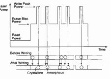
Similar to worm disks, phase-change rewritable types have amorphous and crystalline areas but the crystalline areas formed by melting can be reversed by heating to just below their melting point.
