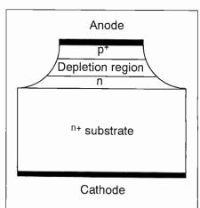
Fig. 6. Varactor mesa doping profile and the approximate equivalent circuit of the packaged chip. Cp and Lp are parasitics while Rj and Cj are the junction resistance and capacitance.
