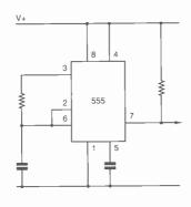
July) can be more simply realised by reversing the roles of pins three and seven. Pin three is normally the output and has active pull-down and active pullup. Pin seven is normally the discharge route, and has only active pull-down (being open-collector).
