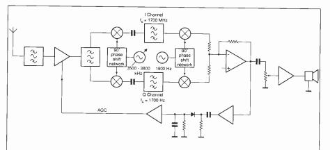
Receiver block diagram. Most of the circuitry is divided between five separate modules: rf amplifier and dual first mixers; 2-phase rf oscillator; dual 7-pole low-pass filters; dual second mixers, audio amplifier and agc circuit; two-phase second oscillator.
