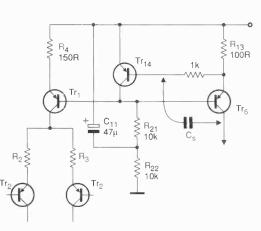
Fig. 7. A modified biasing system that makes  $Tr_6$  current the controlled variable, and reduces the feedthrough effect.
