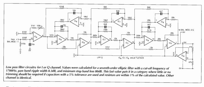
The low pass filter design is detailed in Ref.4. Values were calculated for a seventhorder elliptic filter with a cut-off frequency of 1700Hz, pass band ripple width 0.3dB, and minimum stop band loss 80dB. This last value puts it in a category where little or no trimming should be required if capacitors with a 5% tolerance are used and resistors are within 1% of the calculated value.
