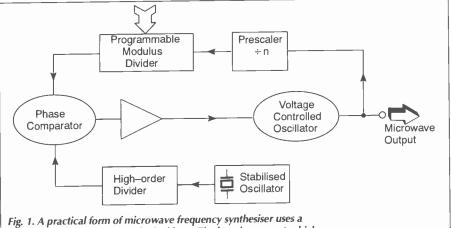
Fig. 1. A practical form of microwave frequency synthesiser uses a fundamental VCO in a phase locked loop. The loop incorporates high frequency dividers, one having a programmable modulus.
