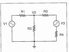
Fig. 3. Simplified model of a negative feedback network which can be used to determine the loop parameters with sufficient accuracy. Design of this model is based on a series RLC loop.
