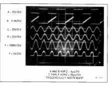
Fig. 2. Waveforms for the cold-cathode fluorescent lamp supply. Triggering is independent on traces A and B, and C through F.
