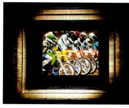
Microscopic rotatable mirrors fabricated on conventional static ram cells could result in a technology to compete with CRTs. This picture was formed by reflection from the micromirrors.
