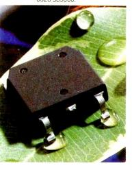
162/262/165/265 SF/FT/TR x16organised memories. Access times are 60ns at 5V or 80ns at 3.3V. By using the pipe-lined fast page mode. cycle times can be reduced from 115ns to 40ns. A 512 by 16 serial memory is included. 2Mb types are also offered. Toshiba Electronics (UK) Ltd, 0276 694600.
