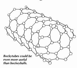
high intensity of the electron beam destroyed any trace of them. But as he began to examine the negative electrode of the arc under the electron microscope, Lijima soon discovered something far more interesting: tiny needles of carbon about a micron long and between 4 and 30 nanometres in diameter
