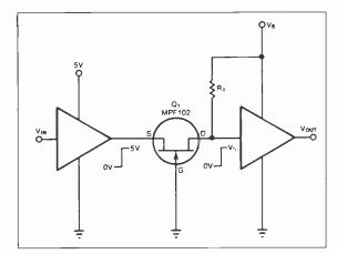
The jfet, operating in the commongate mode, provides lowpower translation of a 5V logic signal to higher-voltage levels,
