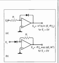
(a) Logarithmic amplifier with junction connected into negative feedback loop; (b) antilog amplifier.
