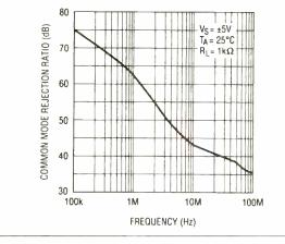
Fig. 4a. Common mode rejection ratio vs frequency for the LT1193.
