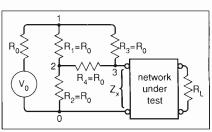
Modelling a return-loss bridge at the relevant port allows plot of insertion loss and, without further computation, return-loss plot simultaneously.
