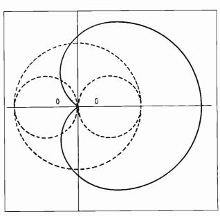
Combined omni and loop polar diagram, showing heart-shaped field. Cardioid null is not quite as sharp as from loop alone and is usually used merely to show which way to turn loop for correct null. This is unnecessary in Lipschutz's design. Signal from omni must be exactly the same in magnitude and phase as that from the loop.
