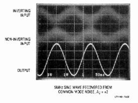
Fig. 3b. Recovered signal from common mode noise.
