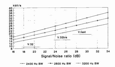
modems will establish initial line speed conditions and so transmission speed by sending a probing signal at the beginning of the handshaking sequence. The modem will then categorise the line into one of several pre-ordained categories before resorting to more traditional training methods.
