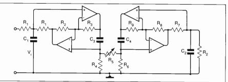
Fig. 4 Gyrator realisation of bandpass filter from Fig.1b.
