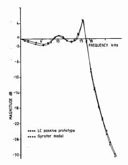
Fig. 7. Magnitude characteristics and Fig. 8 (below) phase characteristics, of a simulated filter derived from the simulation of the circuits in Figs. 5 and 6. 15kHz has been taken as the cut-off frequency.
