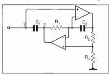
Fig. 2 FDNR circuit model realised by substituting a capacitor for  $R_1$  in Fig.1b and by interchanging the component locations of C and  $R_3$ .
