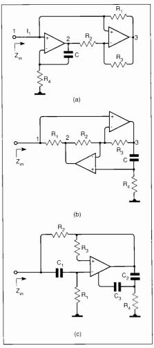
Fig. 1. Three realisations of a gyrator circuit using an op amp.
