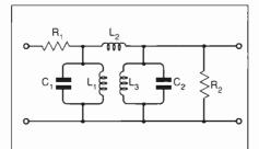
Fig. 3 Prototype of a coupled resonator bandpass filter.
