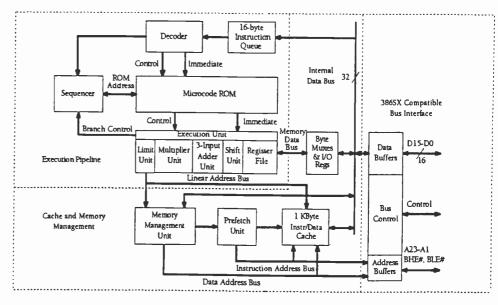
386 pin-compatible Cyrix architecture speeds up a PC by a factor of two over a 386 powered machine run at the same clock speed. Extensive use of pipelining accounts for the boost.
