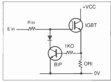
Fig.2. Latch-up protection. Input n-p-n transistor turns on if output current exceeds set limit.
