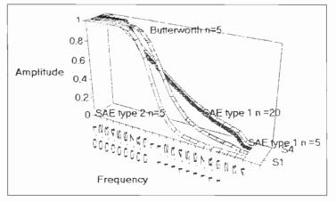
the techniques are equally applicable to high pass, band pass, notch or indeed any configuration which can be mathematically described. First of all a very general form of low pass filter (now referred to as type 1) can be expressed as:
