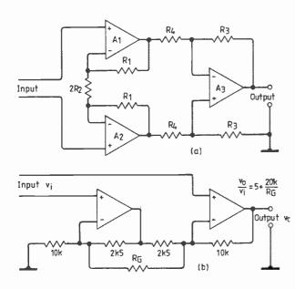
Fig. 1. Instrumentation amplifiers, floating high-impedance input. Circuits using (a) three op-amps or (b) two op amps.
