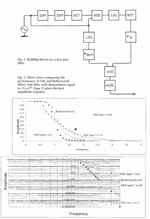
This signal is of course our original signal but is now multiplied by  $\omega^2$  and is suitable for input to the SAE equation. An important point to note is that for real life signals containing many such sinewayes, there is no relative phase shift amongst them in passing through this procedure: all frequencies rotate through one full circle of 360°.
