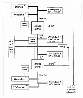
The board has three banks of zero wait-state sram (banks 2, 3 and 4) and one bank of dynamic ram (dram), Processors have exclusive use of one bank each (bank-3 for DSPA and bank-4 for DSPB) and access is through the respective processor's outer port. Each outer port is also linked to the processor's respective HyperBus port.
