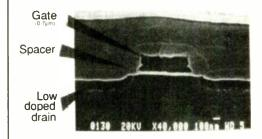
The ECPD07 0.7µm process resulted from a joint venture
