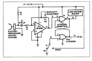
Fig. 7. Ambient sound above a user-determined threshold activates this intrusion detector. Once triggered, the alarm will sound until you momentarily press the switch (S<sub>1</sub>).
