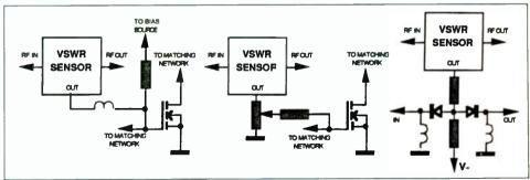
Fig. 2. Three possible methods of using VSWR sensor to control RF gain of amplifier. First two vary bias on mosfet and are useful for complete, fast shutdowns. Third method gives gain reduction for linear amplifier.
