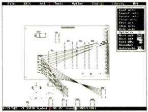
Optimized placement by displaying ratsnest per component. Lines indicate the unrouted nets.
