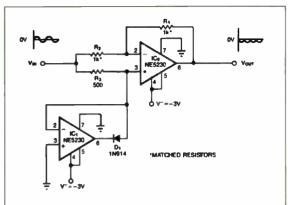
Fig. 4. This circuit (obtained by reversing the power supply connections in Fig. 3) performs negative full-wave rectification using a single supply voltage.
