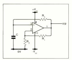
Fig. 1. Common form of op-amp oscillator, providing 50:50 mark:space ratio with equal supplies. Feedback resistors determine reference voltage.
