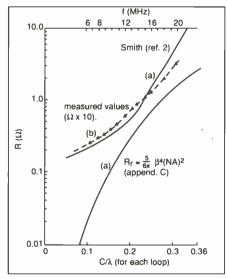
Fig. 5. Comparisons between expected and measured radiation resistance.
