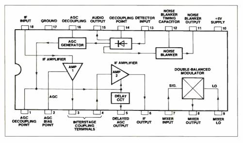
Fig. 3. Use of SL6700 in broadcast receiver takes advantage of detector linearity. Low supply needs are convenient in portables.
