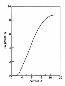
Fig. 1. Light output as a function of input current for 8mm monolithic array of 50µm emitters on 500µm centres.
