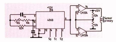
Fig. 1. The driver circuit used in all version
