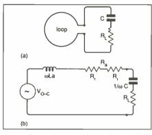
Fig. 3. Electrical circuit of a single tuned loop with resonating components.
