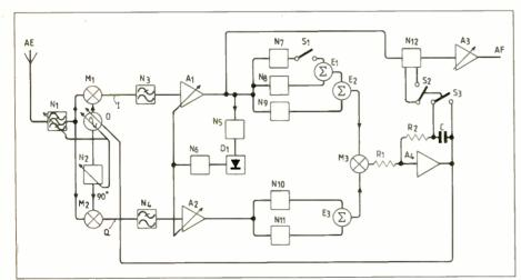
EC Forster's direct-conversion synchronous receiver for AM or reduced-carrier SSB broadcast
