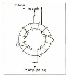
Fig. 6. Balancing/matching transformer.
