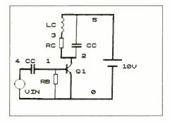
Fig. 3a (top) Transistor tripler model.
