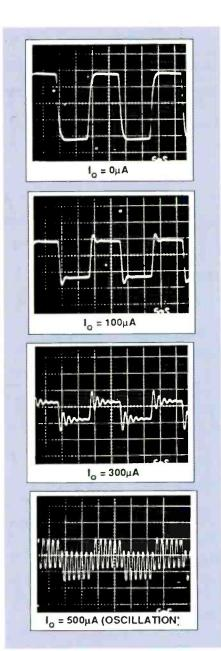
Fig. 3. Effect of applying a square wave to the circuit for different values of  $I_{O}$ .
