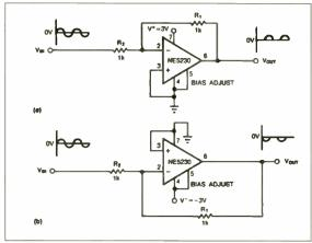
Fig. 2. Requiring no external components, these op amp circuits perform (a) positive and (b) negative half-wave rectification for ground referenced AC signals.
