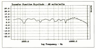
FFT of first of impulse with all room reflections removed. Frequency resolution is 330Hz, so low frequencies have been excluded from graph, printed as zoomed by cursors. This is the pseudo-anechoic response and is not smoothed in any way.
