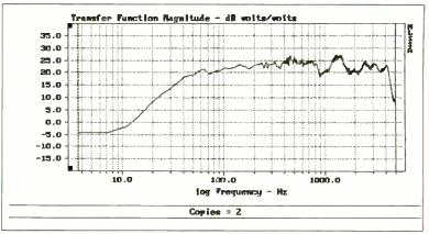
Low-frequency resposne taken with 5kHz bandwidth and 4096 points acquisition, giving a resolution of 3.66Hz. This was taken with the microphone at 12cm from the woofer and shows the response clearly down to about 10Hz.
