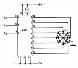
Fig. 7. A simple octant compass display
