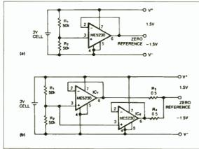
Fig. 9. This bridge transducer interface circuit conditions the bridge's output signal for ratiometric operation and eliminates the need for a reference voltage and an instrumentation amplifier.
