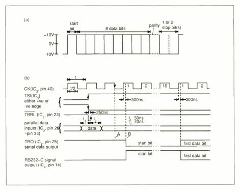
Fig. 2. Serial data format and levels at output of RS232-C driver (a). Number of stop bits is optional, as is inclusion of odd or even parity bit. Timing of circuit is at (b). Point A is first negative edge of clock, at least T/2+175ns after positive edge of TBRL; B is start bit time, T/2+300ns after A.
