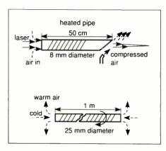
Top, Air passes through a heated pipe so that air nearest the pipe wall becomes hotter than that near the middle, has a lower refractive index and so produces a "rolled up mirage".
