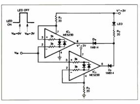
Fig. 5. This window detector's rail-to-rail input range allows the circuit to detect faults in which the input signal becomes shorted to either rail.
