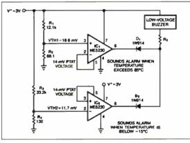
Fig. 6. The op amp's bias-adjust pin (pin 5) is the PTAT (proportional to absolute temperature) voltage, which lets you use the amplifier as a temperature sensor. This circuit activates the buzzer when the temperature exceeds a user-specified limit.
