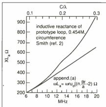
Fig. 4. Inductive reactance of prototype 0.454m loop
