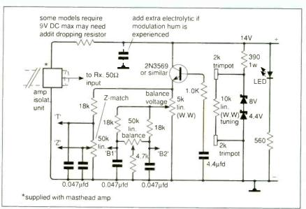
Fig. 8. Tuning and control circuitry. 8(a) (left) masthead tuner; 8(b) above) control box.
