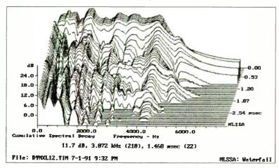
Cumulative decay spectra of loudspeaker in sealed box, showing the decay in sound output after the "stimulus" has stopped. Plotted with a linear frequency axis.
