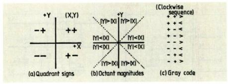
Fig. 6. Mapping out the octants with translation to Gray code equivalent
