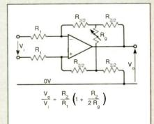
Fig. 3. Another way, giving adjustment from  $R_2/R_1$  to a high value.
