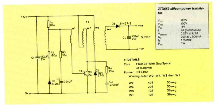
Fig. 1. Self-oscillating inverter for NiCd battery charging.
