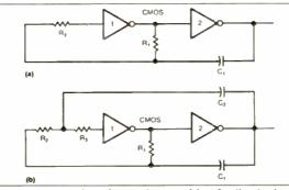
its transition region,  $C_2$  provides positive feedback, thus rapidly moving Gate 1 out of its transition region.
