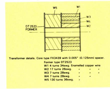
40 turn winding is needed to obtain the correct inductance for  $W_2$ .
