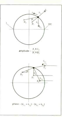
amplitude, they can be placed anywhere. Poles cause an increase in amplitude and can only be placed inside the circle; put them on the circle, or outside it, and the filter is unstable.
