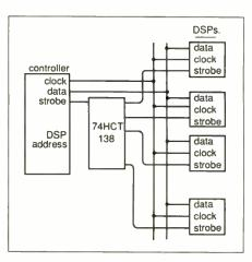
Fig. 8. Passing control data to the DSPs.
