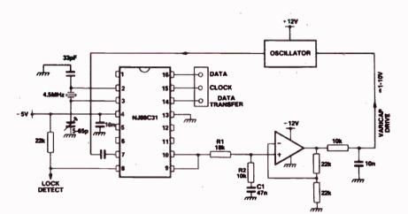
One application of the Plessey chip, in this case for a VHF-only receiver. Control is by means of the three lines on pins 14-16.
