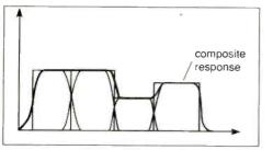
Fig. 3b. Response with bands at differing levels.
