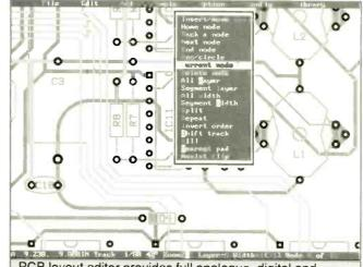
PCB layout editor provides full analogue, digital and surface mount support - ground and power planes (hatched or solid)- 45 degree, arced and any angle tracks.
