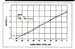
Fig. 2. The dotted line indicates the response of Fig. 1's circuit for the 100Hz to 10kHz audio range; solid line indicates an ideal response. Full scale (0dB) equals 300mV pk-pk.
