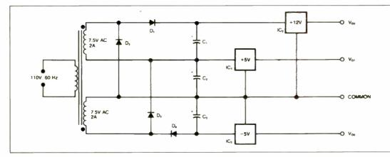
Fig. 1. Simple power supply generating three regulated voltages using a minimum of components.
