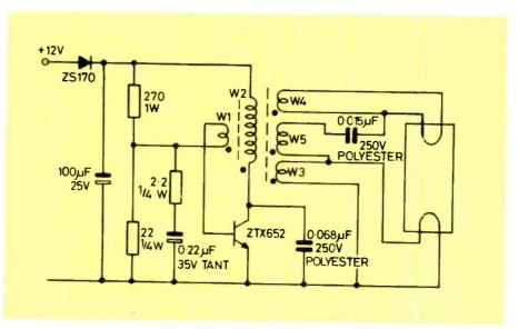
Fig. 3. Driver for an 8W fluorescent tube running at 20kHz. Only one transistor is needed since the ZTX653 supplies energy to the tube in both forward and flyback modes.
