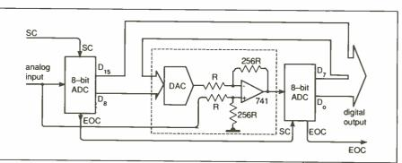
Two low-resolution A-to-D converters perform the function of one high-resolution type, the principle being capable of extension to an increase of n times.
