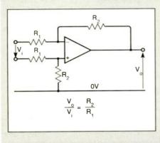
Fig. 1. Ordinary differential amp for fixedgain operation.
