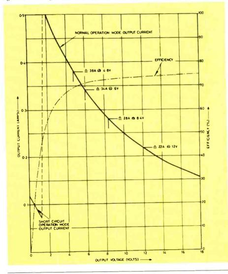
in the range of 4.8 to 15.6V from a supply of 12V. It provides a charging current of 220mA at an output voltage of 12V.
