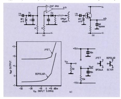
added if the absolute detected DC level is important. When comparing the performance of a jfet with a bipolar infinite impedance detector, the more abrupt cut-off of the latter results in a higher dynamic range, **Fig. 1c**.
