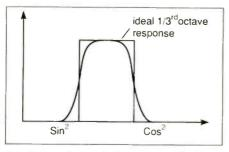
Fig. 3a. Filter's practical response with sin<sup>2</sup> cos<sup>2</sup> transitions.
