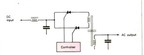
Fig. 3. The ferroresonant inverter is an SCR bridge with a tuned resonant transformer in its output.
