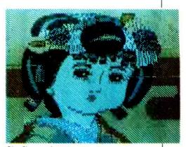
Sin diagonal, 256×85 colour activematrix displays from GEC. Notice the line faults in the lower picture.
