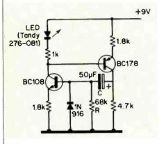
the led is high, so the circuit may be triggered by the photovoltage generated by a light shone on it, the led then illuminating. No power is consumed during the off state. W. Gray
