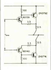
3.3  $\Omega$  will suffice. The voltage lost at peak drive current is still acceptably small: only 0.66V at 200 mA, for example. As before, higher resistor values will increase the compensation.
