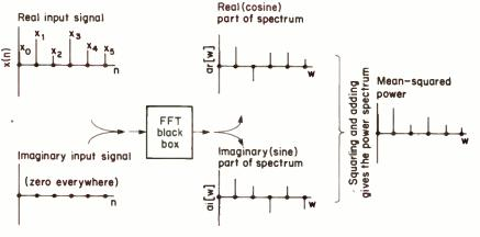
Fig.6.15. Graphical description of fast Fourier transform
