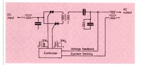
cycle of the square waves, additional control circuitry is added.
