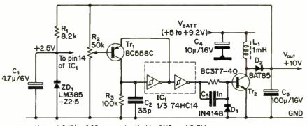
Unused I/P's of IC; must be tied to GND or +2.5V
