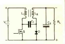
Fig. 3. The Cúk circuit allows the integration of separate inductors into a single, close coupled transformer. DC currents in the core cancel out minimising the problems of core saturation.
