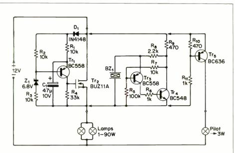
Transistors  $Tr_3$  and  $Tr_4$  act as another multivibrator, using two bipolar types, to provide an audible signal. The piezoelectric buzzer (Murata PZKM 4201 EPP) does not operate at its resonant frequency, but must be capacitive to act as the timing capacitor.
