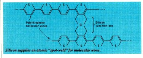
an arrangement that allows a totally flexible configuration. The difficulty, however, has been to do this without creating unwanted bonds or losing the conductive pathway.
