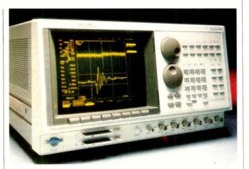
DL2100A 200Msample/s oscilloscope from Yokogawa, distributed by Marton Instruments.
