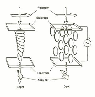
temperatures it is an isotropic liquid. But, unlike other materials, it goes through a phase in which it is a semiordered liquid. By applying an electric field you can control the way the molecules in this liquid line up.
