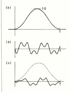
Fig. 6.19. Hanning window. At (a) raised-cosine function is generated using window[z]=0.5\*(I-cos(2\*PI\*z/N)), where z is sample point number and N number of samples. In (b) is truncated data set to be transformed and (c) shows effect of multiplying data set by Hanning window.
