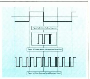
Fig. 3. Generating direct-sequence spread-spectrum signals by modulating the data with a pseudo-random code.
