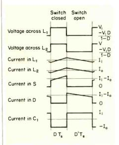
Fig. 2. Voltages and currents during the Cúk cycle
