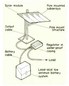
Typical solar generator system (up to 200w load) as supplied by Solapak Ltd.
