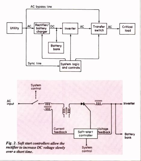
Soft start (Fig. 2) is simply a circuit that allows the rectifier/battery charger to increase the DC bus voltage slowly, over about 15 seconds.
