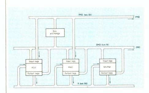
Fig. 4. Analog Devices ADSP2100 has dedicated MAC and straightforward arithmetic section.
