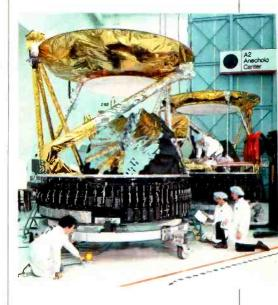
Building satellites: the communications section of Intelsat VI. The completed satellite, launched on March 14, can carry 120 000 telephone calls and three TV channels. There will be five Instelsat VI spacecraft in orbit by the end of 1991.
