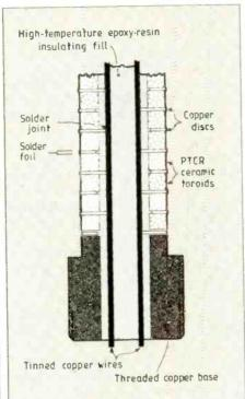
current drop, stabilizing the ceramic at a particular temperature. Any alteration in surface cooling will produce a sharp change in current as the ceramic naturally regains its equilibrium. So the material is effectively a self stabilizing measure of any external changing cooling rate.
