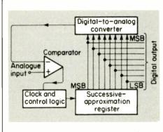
Fig. 2.3 System diagram of successive approximation A-to-D converter
