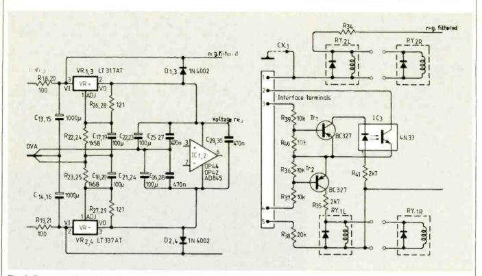
Fig. 3. Power supply and interfacing circuit for muting and de-emphasis relays.
