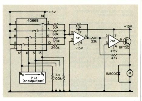
Fig. 1.9 Hardware for computerised speed control is simple: most of the work is done by software.
