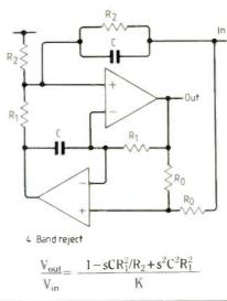
four digitally-selectable filter functions, namely band-pass, high-pass, all-pass and band-reject.
