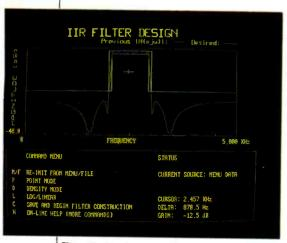
Fig. 5. Design envelope of an infinite impulse-response filter.
