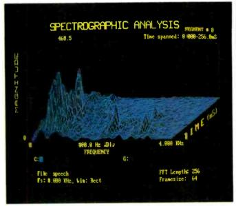
Fig. 3. Three-dimensional spectral display for showing develoment of a signal.
