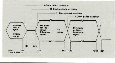
or inverted form on alternate lines to allow the decoder to recover correct colour after an interference burst. There is also a 64-bit vertical sync. word at the start of line 625.
