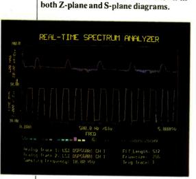
Fig. 7. Displays from spectrum analyser and oscilloscope can be combined in one frame.
