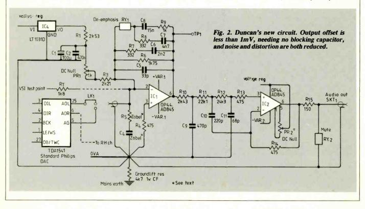
is beginning to fall off, at mid to high audio frequencies. Power supply noise measured across  $C_1$  is now many orders better than the original, as well as being below 16-bit audio's best SNR. The significance of measuring across  $C_1$  is that the voltage present here appears more or less unchanged at the output of  $IC_1$ . The trimmer PR<sub>1</sub> trims the current supplied to match the standing current of individual DACs for complete DC cancellation.
