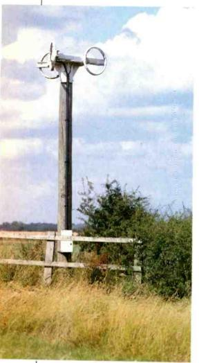
is the desired bearing of GW with respect to the orthogonal loop pair A and B. Component H<sub>a</sub>, being normal to the Poynting vector of AW, has a component x in line with GW at the earth surface. This is shown in plan view in **Fig. 1b.** The addition of H<sub>g</sub> and x produces R which, acting in loops A and B, gives an erroneous bearing  $\beta^*$ .
