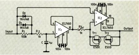
13 and a new output taken from pin 12 which is the amplifier's clock output. Because the oscillator has a divide-by-two counter the output will be one-half the input frequency.
