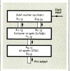
the most significant bit of the counter (13th bit onwards) are Exor-ed with the corresponding least significant bits and given as the address to the rom. This way the 4K PRN data is read out in many combinations and output as a different sequence for each possible combination of the most significant bits of the counter; as a result the sequence length is increased. This circuit has a maximum sequence length of  $2^{24}$  clocks. A. Dhurkadas Naval Physical & Oceanographic Laboratory Cochin India
