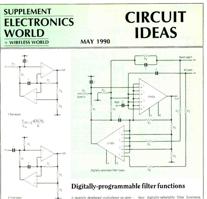
A recently developed multiplexer op-amp – the LM604 – can be configured to provide
