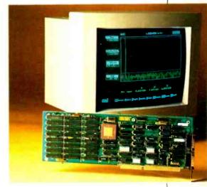
AT&T's newest 32bit DSP chip, the 50MHz DSP32C, calculates at 25 million floating-point operations a second, can evaluate a single-tap, finite-impulseresponse filter in 80ns and perform a complex 1024-point FFT in 3.2ms.
