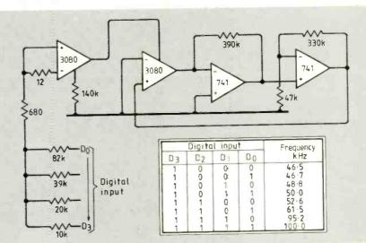
The circuit has been tested using the 741 op-amp, the CA3080 operational transconductance amp and a passive Dto-A converter. For a digital input from 1000 to 1111, the frequency of oscillation varied as shown in the table. Muhammad Taher Abuelma'atti University of Bahrain
