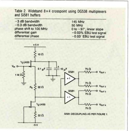
Fig. 3. Multiple-output high-performance buffer
