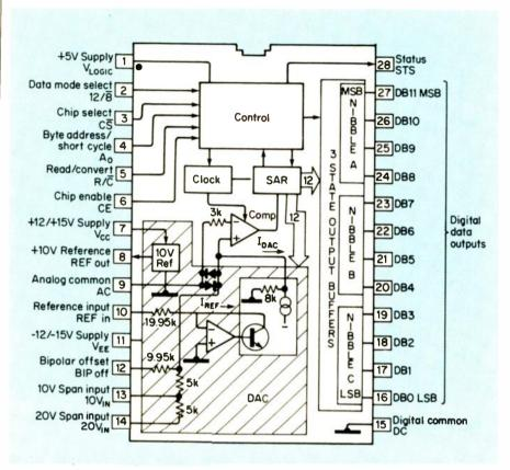
Fig. 2.9 AD574A block diagram and pin configuration
