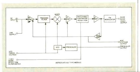
Satellite mini-receiver. Astec's receive-only module covers 950 to 17750MHz, the downcoverted European satellite TV band, and provides positive sync, raw video derived from a demodulated IF of 479.5MHz. Quoted noise figure is 12dB. An internal prescaler can be set to either 256 or 512 for use with an external synthesised tuning system.
