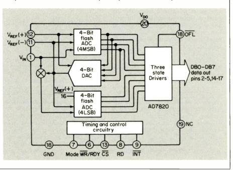
While the output from the A-to-D is latched, the digital signal is reconverted to analogue form for a second conversion with a 1/16 weighted network to make up the least significant bits of the 8-bit output word.
