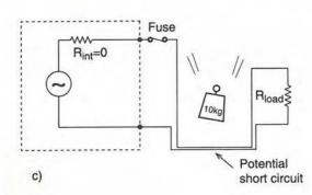
The other main characteristic to be considered is the  $I^2t$ rating of the fuse. This represents the current pulse needed to open the fuse 'immediately', in the event of a gross overload, such as a short circuit. Immediately, here, means in less than half a cycle of the mains, typically
