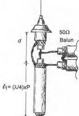
$\ell_2 = \lambda x 0.27 (50 \Omega \text{ line})$  $\ell_2 = \lambda x 0.24 (75\Omega \text{ line})$
