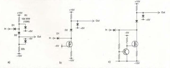
Fig. 8a). Given suitably rated diodes, this frequency-counter input-stage provides protection up to 316V dc, 612V rms continuous, 1kV rms short term.
