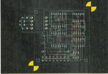
Fig. 4. The rat's nest of Fig. 3 autorouted in Specctra and returned to WinBoard format. Note the nonmitred corners. See the text for an explanation of this.
