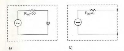
Fig. 1a). An rf signal generator typically has a source resistance (internal resistance) of 50Ω. b) An ideal constant voltage generator has an internal resistance of zero. c) Consequently, if its output is short circuited, a very large fault current will flow, unless fuse protection is provided.
