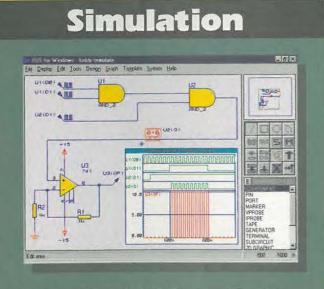
●Non-Linear & Linear Analogue Simulation. ●Event driven Digital Simulation with modelling language. ●Partitioned simulation of large designs with multiple analogue & digital sections. ●Graphs displayed directly on the schematic.
