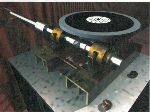
Fig. 6. The author's modelling of Baird's Phonovision recording studio of 1927/28 shows the drive-shaft from the scanning disc connected through a 3:1 worm gear to the record platter.
