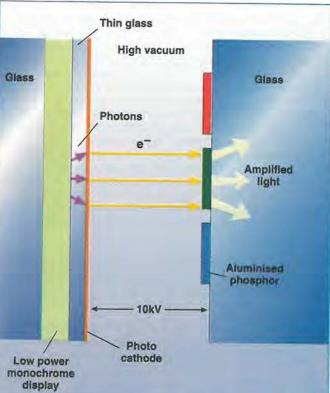
established image intensifier, or 'night-sight,' technology where light striking a photocathode is used to produce electrons.
