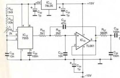
Fig. 6. 3150Hz reference oscillator. A divided-down crystal reference is often used here, but this circuit was found to give adequate stability, as you will see from Table 2. The circuitry conditioning the 555 output turns the rectangular wave into a sinusoidal one.
