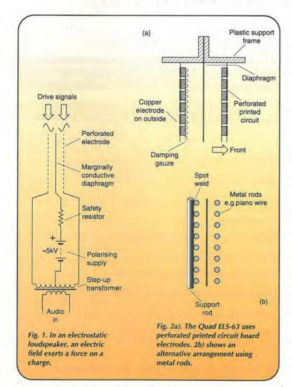
which are perforated to let the sound out. The electrodes are connected to a balanced high voltage audio signal. Several kilovolts may be used. Enthusiasts may build direct drive amplifiers using transmitter valves, but commercially available units employ step-up transformers so that a fairly conventional amplifier may be used.
