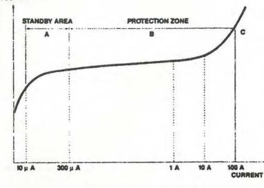
Fig. 11. Current through a zinc-oxide varistor is negligible in the standby area A, but increases rapidly with voltage in the protection zone B. Reproduced courtesy of Philips.
