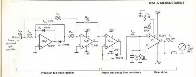
Fig. 5. Quasi-peak indicating full-wave rectifier with meter-drive and the circuitry determining attack/decay time constants.
