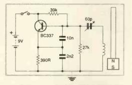
Fig. 4. A basic oscillator detects the Earth's magnetic lines once a magnet is glued to one end of the ferrite. The beat frequency with a medium-wave transmitting station falls in the audio range and can be heard on a radio and measured. Even tiny movements of the rod or the impinging magnetic lines causes an audible change of the beat note. If high stability is required it is advised to build a second identical oscillator instead of using a commercial station.
