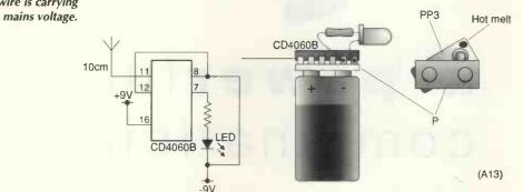
the led flashes at about 3Hz; if the wire is not connected to the mains, the led is either lit or unlit, but does not flash regularly.
