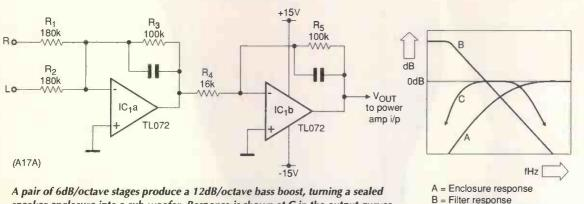
speaker enclosure into a sub-woofer. Response is shown at C in the output curves.
