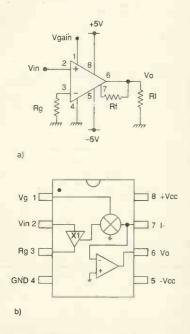
Fig. 5a). The CLC5523 conected as a noninverting amplifier.
