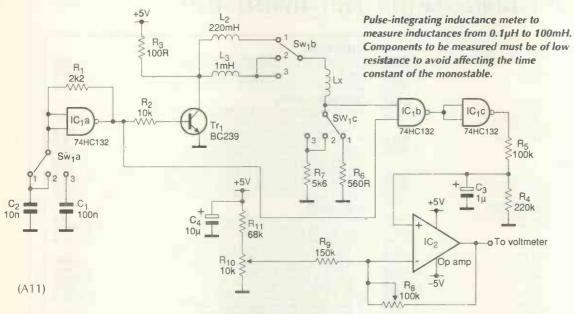
the transistor. When the transistor is cut off by the monostable, the unknown inductor takes current through  $R_6$  or  $R_7$  and  $R_3$ . On the next half-cycle, the transistor conducts and
