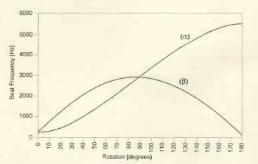
Fig. 5. Curve (a) refers to the north-south orientation of the ferrite rod and curve (b) to the east-west. Rotation takes place on an horizontal plane. If the rotation plane changes, the frequency range of the beat frequency will also change since the magnetic lines are parallel to ground only at the equator. Consequently, an accurate measurement must take in account the latitude, 45° in this case, and the plane.
