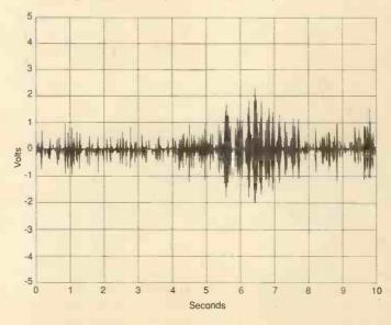
Fig. 9. Seismogram of a lorry, barely heard in the silence of the night, passing in the area and measured over 10s. The frequency range of the signal is mostly between 10 and 50Hz and is bound to interfere with a real seismic wave. This demonstrates that careful choice of the installation site is important if you want to record natural phenomena.
