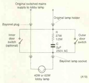
A lobby light left on permanently will cost less and last longer with this switching circuit.
