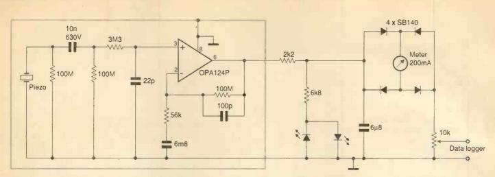
Fig. 8. There are no settings or adjustments in this seismic detector. The screened portion is placed together with the piezoelectric detector and connected to the remaining part of the circuit with a three-core shielded cable. Piezoelectric gas lighters are economical and readily available. The element from any such lighter should be suitable for the detector.
