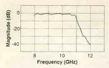
Fig. 5. Actual measured filter performance for gain, S21.
