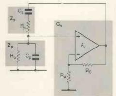
Fig. 1. Wien-Bridge oscillator using an opamp with gain  $A_v$  as the gain block.
