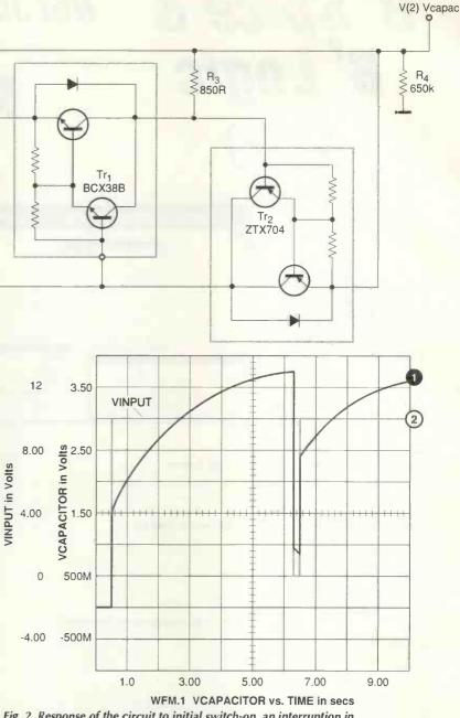
Fig. 2. Response of the circuit to initial switch-on, an interruption in supply and delay after the interruption.
