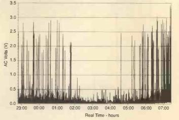
Fig. 10. Printout of data logged from 11pm to 8am the following day. Readings where taken at 1sample/s and shown as an alternating voltage. The  $10k\Omega$ potentiometer was adjusted to accommodate the peak readings of the local tramway. Also in this case there is quiet period around 3-4 am underlining the need to install the detector away from cities, roads and railways.
