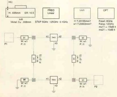
Fig. 9. Schematic for a two-stage distributed amplifier
