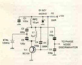
Fig. 1. The LC oscillator of Ref. 1 modified for crystal control.
