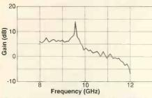
Fig. 8. Measured performance for amplifier gain (S21)
