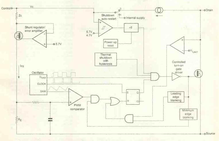
Fig. 1. Functional block diagram of the TOP209 standby power supply chip for output power to 4W.
