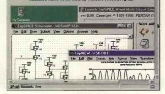
Fig. 4. TopSpice, the affordable Spice based analogue simulator. Unusually, TopSpice provides Smithchart and can use 'S' Parameters.
