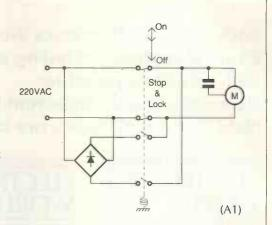
Simpler than usual circuit to stop dead and lock an induction motor by applying dc to it.
