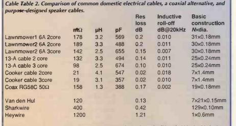
All data are for 5m round-trip, measured at 1kHz. Inductive roll-off is ref 1kHz, ie this is the *extra* attenuation due to inductance. Data for the last three commercial speaker cables are from Eric Ford<sup>6</sup>; no inductance values were given.
