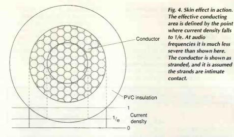
Taking 13A copper mains cable as an example, equation 2 shows that below 13kHz, the skin depth is greater than the cable radius, and there is no significant effect. At 20kHz, the skin depth is 0.47mm, and the conductor radius 0.6mm. The cross-sectional area is 1.08mm<sup>2</sup>, of which only the central 0.06mm<sup>2</sup> is unused. Therefore resistance per metre only increases from  $152m\Omega$  to  $160m\Omega$ , and this can have no appreciable consequences.
