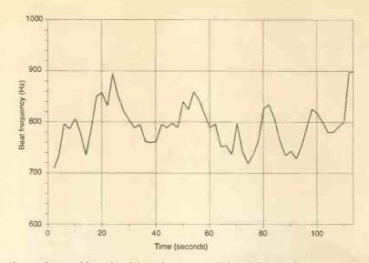
Fig. 6. Printout of from data logger shows the variation of the beat frequency over a period of 113 seconds. Samples where taken at 1s intervals at 6pm in a built-up area. In open country the response is much quieter with several minutes without appreciable changes.
