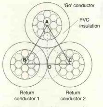
Fig. 3. The geometry of three-core cable usage, showing how inductance reduction works by reducing the effective conductor spacing.
