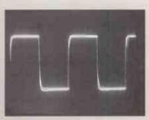
Photo 4. Square-wave response (2kHz) at  $R_1=8\Omega$ .
