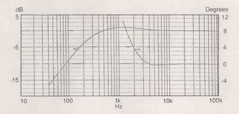
Fig. 5. Bode plot for the circuit of Fig. 4, where all Cs are 1nF and all Rs=100 $k\Omega$ . Gain peaks at +0.9dB at 1.2kHz, but is still in excess of unity at the zero phase-shift frequency of 3.9kHz.
