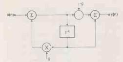
Fig. 8(a) All-pass filter flow diagram.
