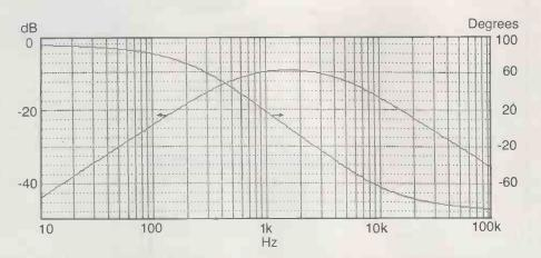
b) Phase and amplitude response (Bode plot) for a). Note the much more rapid change of phase with frequency in the region of maximum output, compared with Fig. 5.
