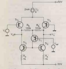
Fig. 3b. Improved solid-state phase splitter reduces distiortion and reduced influence on outpout gain.
