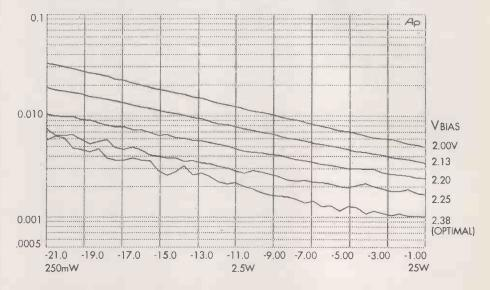
Fig 2. Showing how crossover distortion rises slowly as output power is reduced from 25W to 250mW (8 $\Omega$ ) for optimal bias and increasingly severe underbias (upper lines) This is an emitter-follower type output stage. Measurement bandwidth 22kHz.
