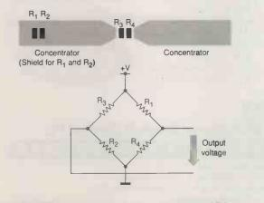
Fig. 5. Giant magnetoresistive sensor layout. In addition to screening  $R_{1,2}$ , the shield concentrates flux through  $R_{3,4}$ .
