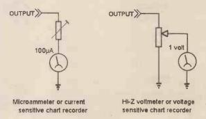
Fig. 5. Additional circuitry needed to connect output of the magnetometer to a chart recorder or voltmeter.
