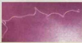
A molecular wire of molybdenum selenide embedded in a polymeric matrix. The thickness of a single wire is approximately three atoms in diameter, with the length about 110 atoms. Approximate magnification is 1 million times.
