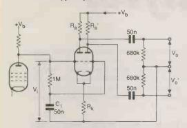
Fig. 2. Conventional phase splitter,  $R_k=68k$ ,  $R_a=100k$ ,  $A=V_o/V_i=25$ , thd=1.8%,  $V_o=25V_{rms}$ .
