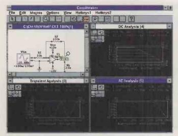
Fig. 16. Typical analogue simulation of a circuit imported into Circuitmaker from Propak using SPICE netlist transfer. Note how the sig gen is connected and the test probe location.
