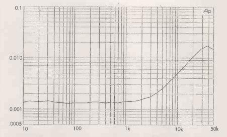
Fig 1. Distortion performance, percentage thd, of a typical Blameless Class-B amplifier at  $25W/8\Omega$ ; the noise floor is at the 0.0008% level. Bandwidth is 80kHz.
