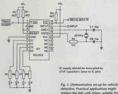
Fig. 1. Demonstration set-up for venicle detection. Practical applications might replace the leds with relays, suitable for alarms, or connection to a data-collecting computer.
