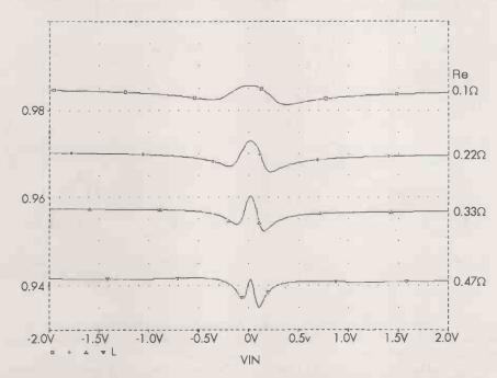
Fig 8. Output linearity of the cfp output stage for emitter-resistance  $R_e$  between 0.1 and 0.47 $\Omega$ .
