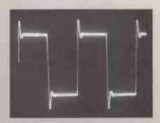
Photo 5. Square-wave response (2kHz) at  $C_L=1\mu F$ .
