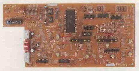
Fig. 2. Microprocessor-based dc controller of Japanese manufacture illustrates that it may wise to consider single-sided designs even for fairly complex
