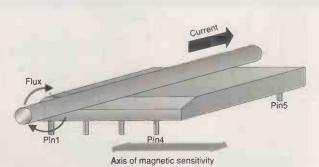
Fig. 6. Placing a conductor a precise distance from the gmr sensor allows current to be measured without calibration.
