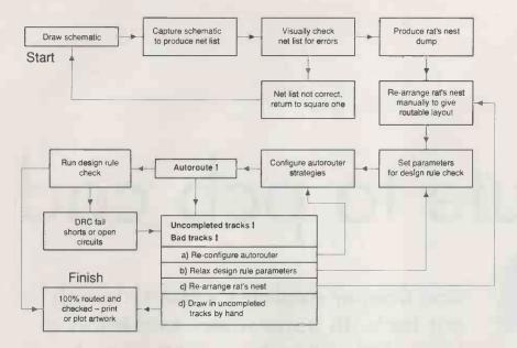
This chart shows the typical steps from start to finish for a schematic capture and autorouter system.
