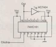
Fig. 1. The '161, shown here dividing by 7, has four program inputs for division to 16.
