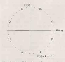
*Fig. 7(a) Visualising the performance of a phase flanging processor using a pole-zero diagram.*
