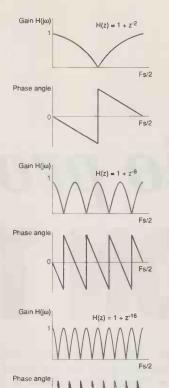
Fig. 2. Frequency response caused by phasing for different time delays. Reconsider this performance with the assistance of zeros on the circumference of unit circle.
