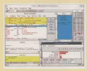
Part of the package is dScope for Windows – an integrated software simulator and debugger for the 8051 family.
