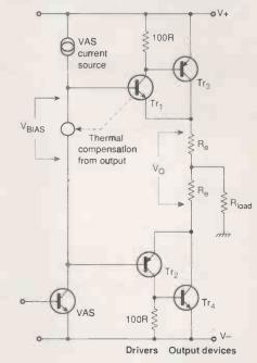
in the transistors; this may appear to be a blindingly obvious, but it was worth checking as there is no inherent reason why the optimal  $V_q$  should not be a function of device temperature. Fortunately it isn't, for thermal com-
