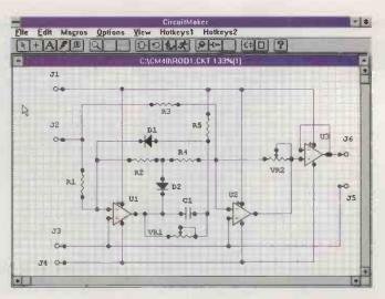
or 95. A well-written and comprehensive manual is provided and there is good on-line help and a separate help directory, plus a very Fig. 14. Schematic in CircuitMaker. Note the lattice grid and pin-out on 741.
