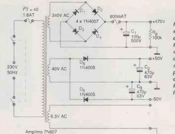
Fig. 6. Power supply circuit comprising ht at the top for the valves – lethal don't forget – ±50V for the phase splitting circuit and 6.3V for the valve heaters.
