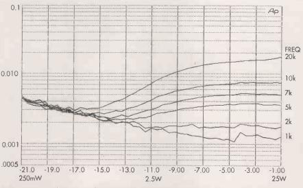
Fig 3. Variation of crossover distortion with output level for higher frequencies. Optimally biased emitter-follower output stage. Bandwidth 80kHz.
