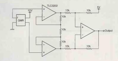
Fig. 7. Giant magnetoresistive device amplifier. Current of 500mA though the sensing wire causes a field of 1 oersted, increasing the differential amplifier output by 666mV. Power supply is 10V.
