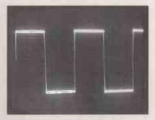
Photo 3. Square-wave response (2kHz) with open output.
