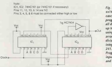
Fig. 3. Two xx161 parts cascaded allow programming of all division ratios up to 256 or, using this arrangement, division of all integers ratio to 241. Programming inputs are A, B, C and D.
