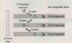
Fig. 3. Giant magnetoresistive devices comprise alternating sheets of magnetic and non-magnetic thin films. This diagram shows conditions when no magnetic field is present.
