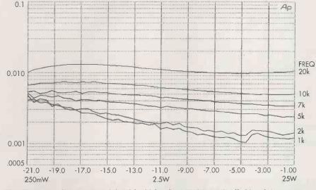
Fig 4. Variation of distortion with level for higher frequencies. Optimally biased CFP output stage. Bandwidth 80kHz.
