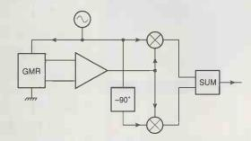
Fig. 8. Giant magnetoresistive sensors suffer form noise. Modulation could be used to remove this.
