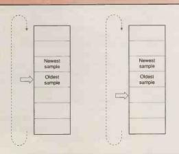
Fig. 3. Circular buffer both before (a) and after (b) a sampling interval. The oldest sample is T.N seconds old.
