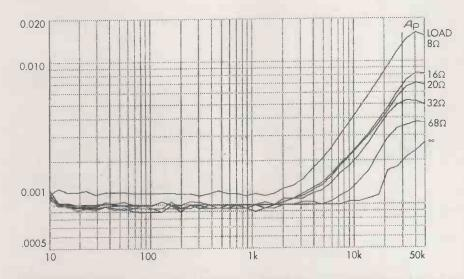
Fig 5. How crossover distortion is reduced with increasing load resistance. Power is 20W into  $\delta\Omega$  and bandwidth is 80kHz.
