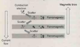
Fig. 4. Resistance of a giant magnetoresistive device reduces when magnetic field is applied.
