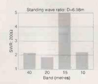
Fig. 2.Standing-wave ratio at the antenna terminals for a standard 1/3-feed dipole.
