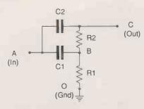
Fig. 2a) Network with two capacitors and two resistors. b) In this case, the circle diagram looks something like this (with provisos, see text). Note that output vector OC can exceed the input OA.
