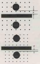
Fig. 1. Finer grids are not always better. In a) a coarse grid allows the design clearance between the track and pad to be achieved, but b), using a fine grid, does not. One of the claims for gridless autorouters is that, by using alternative methods like the geometric-shape technique, the load on the pc's memory is lower. But this does not necessarily mean the router will be quicker. A lot depends on the routeing strategies being used.
