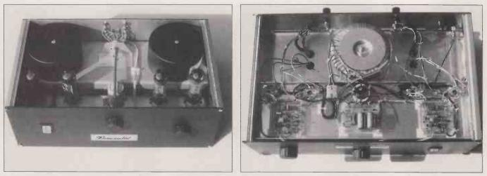
Photos 1, 2. Top and bottom views of the prototype power amplifier. Mounting the valves directly on the chassis offers benefits.
