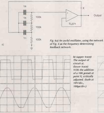
about this amount, and the amplitude of oscillation builds up until there is heavy clipping, Fig. 6b), upper trace.
