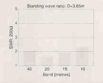
Fig. 4. A further example of how moving the feed point affects standing-wave ratio.
