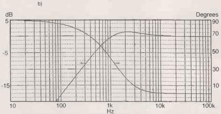
Fig. 3. Bode plot for the circuit of Fig. 2a), for the case where  $R_1=100\Omega$ ,  $C_1=1\mu F$ ,  $R_2=100k\Omega$ ,  $C_2=1nF$ . Thus the loading of  $C_2R_2$  on the  $C_1R_1$  circuit is negligible. Note: if  $R_1=R_2$  and  $C_1=C_2$ , the plot is almost the same except that the peak gain falls from +1.25dB to +0.65dB.
