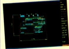
Fig.4. EE Designer III: layout for a two-sided printed circuit board. It can be displayed with trace widths to scale, as here, or with uniform thin lines. Components, except the connectors, and the traces were all placed automatically by the programme.
