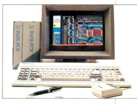
Typical PC-based cad station with PCB design in progress, using PADS-PCB from Microtel which is to be described in a future issue.
