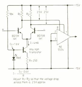
Fig.9. NE5534 op-amp with substituted differential transistor pair for optimum source resistance matching.
