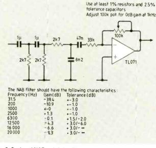
Fig.6. Optional NAB weighting filter for the circuit of Fig.6.
