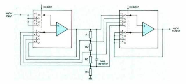
Fig.3. Inserting a single capacitor in the feedback loop of the left-hand op-amp stage makes it possible to control the low-frequencies. Low-frequency gain is determined by the resistors and the effective frequency range by the resistor and capacitor values.
