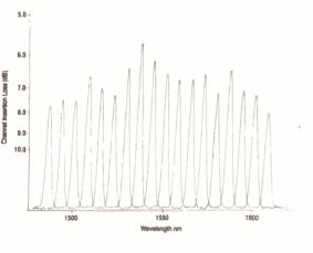
Fig.6. Passband characteristics for 18 channels of the component shown in Fig.5.
