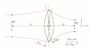
Fig.2: Re-imaging with a quasi-optical lens. Note that the radii of curvature R of the incoming and outgoing beams are not necessarily equal to the distances of the beam-waists from the lens.
