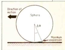
possible to see that the force contributed by the thermal expansion will supplement the momentum of the sphere and, assuming that the friction is extremely small, would ultimately move it randomly across the surface of the plate.
