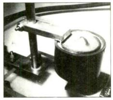
Fig.4. Above, cross-section through mercury fountain and (lower) photograph of it.
