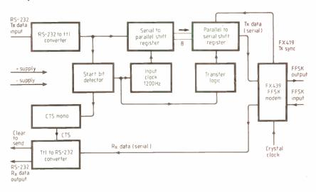
Fig. 1. Block diagram of the link, which provides hidirectional asynchronous communication at up to 1200bit/s.
