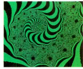
A Hercules Monochrome Graphics display. Part of a Julia set associated with the Mandelbrot set. The resolution is 720 horizontally by 348 vertically, with an aspect ratio of 1.45.
