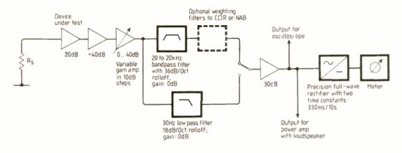
Fig.3. Block diagram of a noise measurement circuit for white noise and flicker noise.
