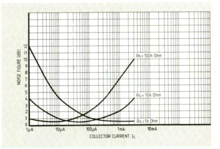
Fig.8. Noise figure and optimum source resistance  $R_{\rm s}$  as a function of collector current  $I_{\rm c}$  for an LM394 transistor.
