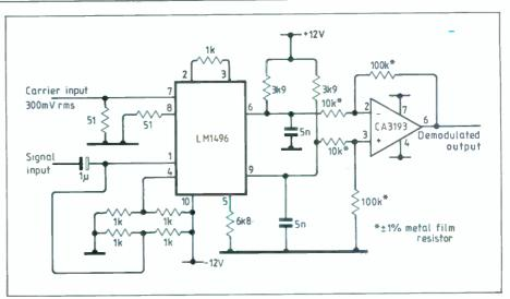
Attenuation of  $2f_c + 2f_s$  products is greater than 60dB. As shown, the circuit is suitable only for low frequencies but if the op-amp is replaced by a CA3450 for example, bandwidth is greatly increased; note that the 3450 and 1496 in this case would both be powered from  $\pm 6V$  rails. The 1496 operates at up to 100MHz.
