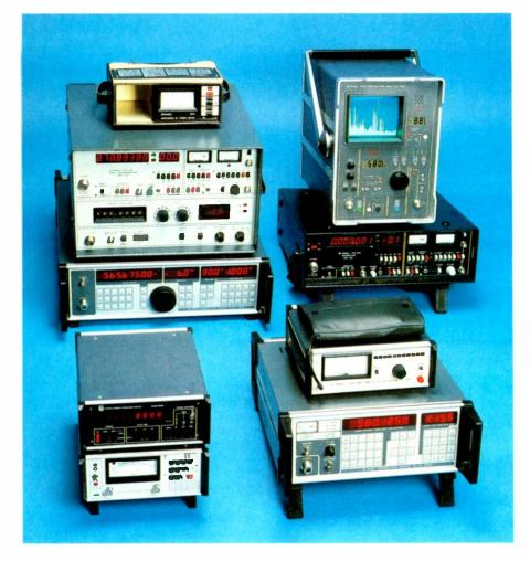
Farnell Instruments Limited manufacture a wide range of test and measuring instruments for use with mobile radios, pocket pagers and other communications equipment. Instruments include synthesized signal generators, transmitter test sets, communications test sets, power meters, automatic modulation meters, frequency meters, etc.
