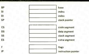
These are common to the 8088/8086, 80286 and 80386. The latter have further registers in addition, used for addressing memory beyond the 1 megabyte memory and in multitasking.
