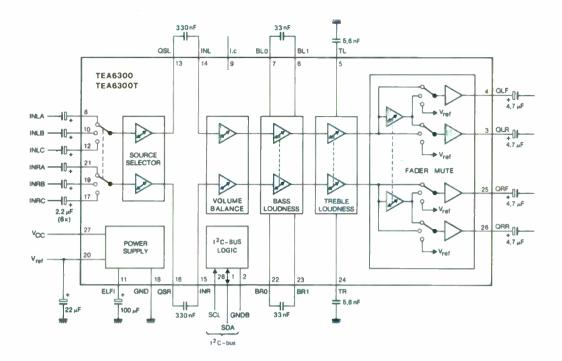
Fig.7. Car radio preamplifier based on the TEA6300. The volume/balance control consists entirely of linear op-amp stages.
