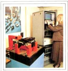
One company within the Institute is devoted to research into precision mechanical engineering. This company, CPE, has produced a machine-tool guidance system consisting of modules for everything from bed positioning to user interfacing.
