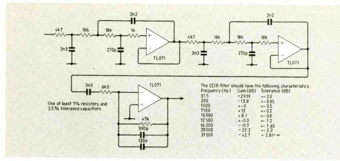
Fig.5. Optional CCIR weighting filter for the circuit of Fig.6.
