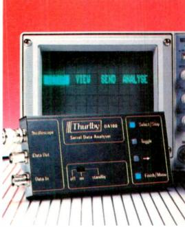
Thurlby's DA100 protocol analyser uses an oscilloscope at its display, showing bit rate, word format and the data.
