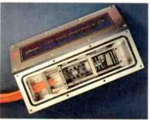
Fig.5. Packaged 16-channel single-mode fibre WDM component. The device features a grating as wavelength dispersive element and a lithium-niobate concentrator.
