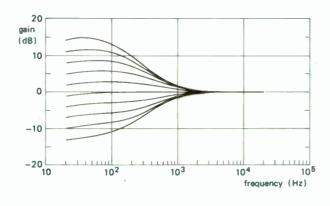
Fig.4. Example frequency response characteristic. Gain control range is +15dB to -12dB in 3dB steps.
