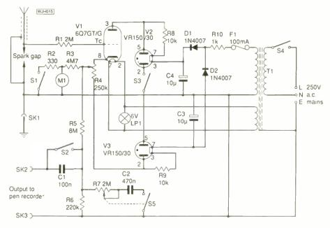
Fig.3. Circuit of the electrometer. It can accurately log atmospheric potentials in the range  $\pm 350V$  (by courtesy of the editor of *Practical Wireless*).
