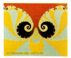
A Video Graphics Array 256-colour display. The large number allows subtle graduations in a display, though the limited resolution of 320 horizontally by 200 vertically loses fine detail.
