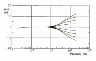
Fig.6. Example frequency response. Gain control range is +12dB to -12dB in 3dB steps.
