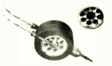
Fig.4. The cavity magnetron, devised by Randall and Boot, contains small, interconnected Hertz resonators, excited directly across the capacitive gaps.
