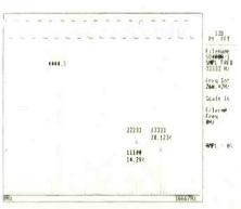
Fig. 2. 40kHz square wave harmonics when sampled at 33.33kHz.
