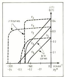
Fig.19. The B-H and J-H curves for various grades of ferrite material all show the characteristics mentioned in Fig.19.
