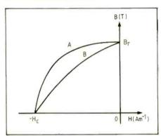
Fig.16. Although the two hypothetical materials shown here possess the same coercivity and remanence, the BH product differs. Material A has a larger "fullness factor" than B.
