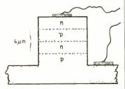
This device, which has characteristics similar to those of a conventional silicon p-n-p-n stack, shows considerable promise especially in its switching speed.
