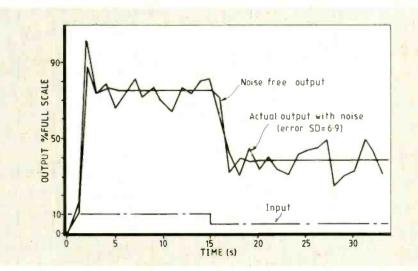
Fig.2. Model representing ideal and noisy behaviour of airflow, providing an input to the Kalman filter.
