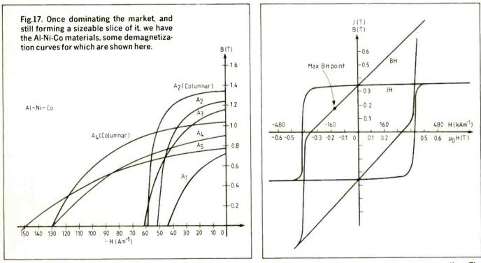
Fig.18 (right). The enormous coercivity, but considerably lower remanence of the ferrite materials produce an interesting effect. The axes can now be plotted to the same scale, as I have done here. The B-H curve now has a maximum slope of minus unity, whereas the J-H curve has a large horizontal section. B can reverse, even while J is still near the saturation value.
