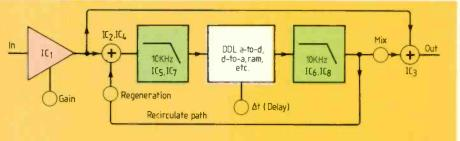
by a four pole low-pass filter IC<sub>57,7</sub>. Output from the delay line is also passed through an identical filter to remove the quantitization step noise. Recovered audio is recirculated through mixer amps IC<sub>1,4</sub> to give a variable reverberation time. Treated audio and the original signal are mixed in  $IC_3$  to provide control over the depth of echo. In spite of there being no companding and no sample-and-hold circuit the audio output is remarkably good. A G Birkett, London.
