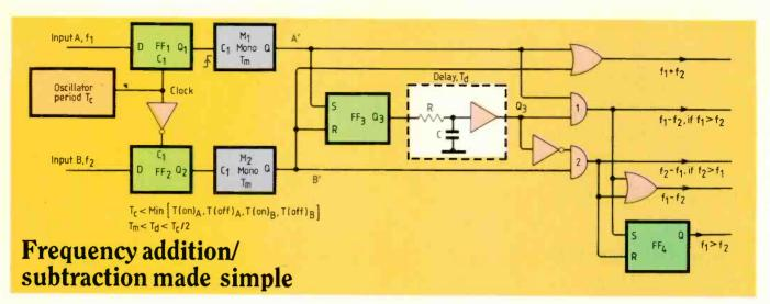
Pulse-cancellation is applied in this design to produce a simple sum and difference circuit that operates over a wide range of frequencies. From input frequencies  $f_1$  and  $f_2$ it produces signals of  $f_1-f_2$  and  $f_1+f_2$  and detects  $f_1 > f_2$ .
