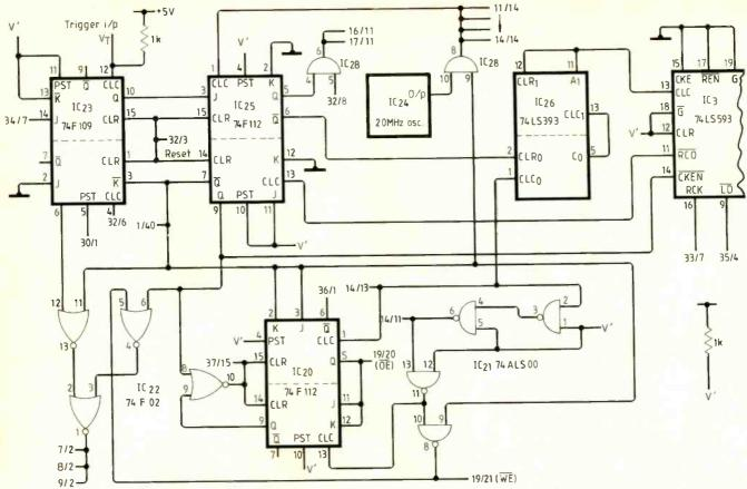
Fig.3. Oscillator and trigger circuitry.
