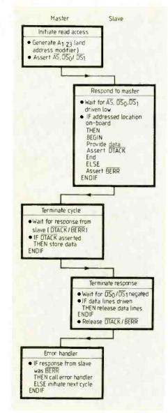
Fig. 3. Protocol flowchart for a VMEbus access.
