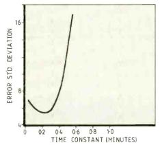
Fig.5. Plot of estimate error against timeconstant of first-order filter, showing that its best performance is poorer than that of Fig.4.
