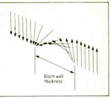
Fig.6. The Bloch Walls mark a region where the direction of magnetization has to change by 180°.
