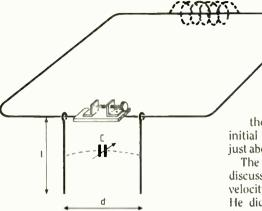
Fig.3. Hertz reports on his experiments with "tuning". "The easiest way of adjusting the capacity of the secondary circuit was by hanging over its two ends two parallel bits of wire and altering the length of these and their distance apart". "Exactly similar results followed when the poles of the secondary circuit were connected with the plates of a Kohlrausch condenser".
