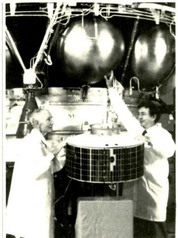
Pioneer Dr Harold Rosen (left) with the prototype of his Syncom. the first geostationary communications satellite. A colleague, Tom Hudspeth, points to one of the fuel tanks of the new Intelsat VI which stands behind in the Hughes plant at El Segundo, California. Syncom, weighing only 35kg, would fit inside this tank. Intelsat VI is 120 times heavier at 4240kg.
