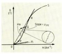
Fig.1. The relation between B and H in ferromagnetic materials is very non-linear. The various slopes from the origin give the permeabilities under different conditions. One of them, the incremental permeability, arises from the shallow slope Q-T as H oscillates along this path.
