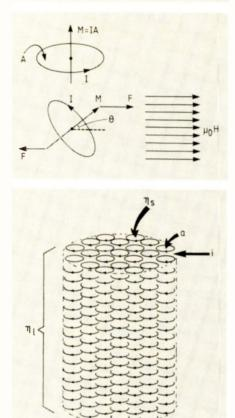
Fig.3. Magnets in an external field experience a torque or turning moment trying to align them a long the direction of the field lines. Hence the function of the magnetic compass. You can see the two ways of looking at this in (a) and (b). The relation between the elementary loop moments and the total moment should become clear from (c).
