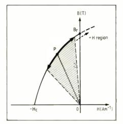
Fig.14. Very rarely do magnets possess a single operating point such as that on Fig.12. Different parts of the material operate on different sections of the demagnetization curve as shown here.
