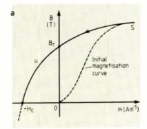
Fig.2. Looking at (a), moving back from saturation near S, a negative value of H eventually reduces the flux density to zero. The path from  $B_r$  to  $-H_c$  carries the title demagnetization curve. The full curve in (b), obtained by going right through a complete magnetization cycle, shows the familiar hysteresis curve of a ferromagnetic material.
