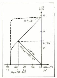
Fig. 20. This curve applies to the largest energy product achieved in a sample of permanent magnet material. The picture also illustrates that the optimum operating point yields a load line slope of 45° in these materials.
