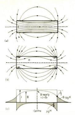
Fig.13. The continuous flux lines shown in (a), concentrate towards the remanent value in the centre of a bar, while the H field strength drops off towards zero at the same position. The field lines proceed in different directions to the flux lines. In general they go in opposite directions inside the material. The graph shows qualitatively how the field strength and the flux density varies from point to point in the material and nearby space.
