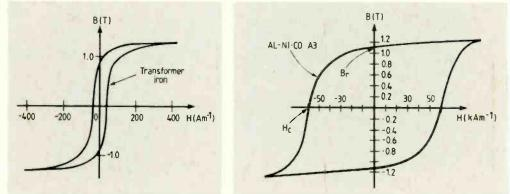
Fig.10. This illustrates the narrow hysteresis curve characteristic of a "soft" magnetic material. Notice the small magnetizing force required for a rapid rise in flux density. Fig.11 (right). A "hard" material has a wide hysteresis loop with a large coercivity,  $H_e$ .
