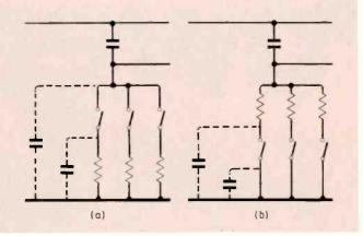
Fig.15. Switching capacitance effects for either switching method.
