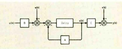
Fig.1. System diagram of a Kalman state estimator.
