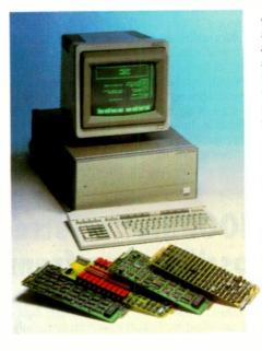
seventies, the 6954A has eight slots, expandable in 16-socket frames to 120, a 300 series computer, 1Mbyte of ram and a 20Mbyte disc, whilst running Basic 5.0 and maintaining compatibility with the previous series software. The computer, actually a 310 series with 68010 c.p.u., replaces the 68000 series 300, which in turn supersedes the series 200 introduced six years ago.
