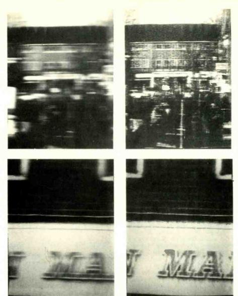
There is little that can be done to improve a blurred image by optical means but when the image is represented in digital form, the information can be manipulated mathematically. These blurred images, produced by a rotating camera, were deblurred using a convolution filter developed by Smith Associates of Guildford. The convolution filter is part of a high-speed image processing computer.
