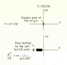
Fig.5 The Laplace transform of the ramp function  $t \rightarrow \frac{1}{s^2}$  gives rise to a double pole at the origin of the s plane. The frequency shifting rule has the effect of moving the poles to the left by  $\frac{1}{\sqrt{cR}}$  units.
