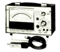
LEVELL BROADBAND VOLTMETERS TM6B 16 LF ranges as TM3B + 8 HF ranges 1mVts/3Vts accuracy 4% + 1% fs at 30MHz. ±3dB 300kHz-400MHz
