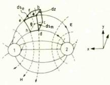
Fig. 3. The key to handling the field approach to lines means constructing a small volume in the space around the line, bounded by the E field lines, the H field lines and direction of propagation, z.
