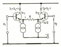
Fig.1. The basic circuit of the long-tailed pair.
