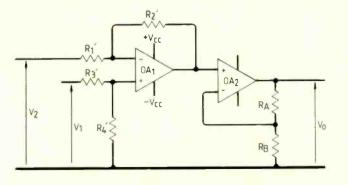
Fig.4. One way of obtaining a high gain, which can only provide a c.m.r.r. equal to that of the first stage.
