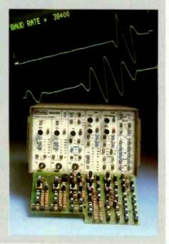
O Increasingly complicated nature of multiprocessor systems makes analysis by conventional logic analysers extremely difficult, if not impossible, according to Dolch Logic Instruments. Their latest model M128 incorporates a twin-slot capability that allows two cards to be linked together and analyse data on two independently clocked and synchronized processors.
