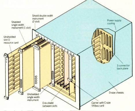
Shown here is a VXIbus mainframe used for internal product development at Hewlett Packard Co. Also shown is a prototype instrument module and a carrier assembly that allows standard B size VME modules to be integrated into C size mainframes.
