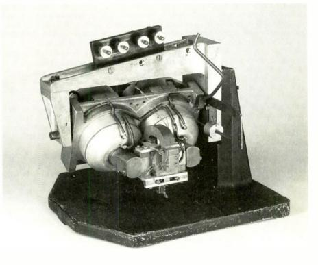
Moving-coil recording head, 1930/31 (Thorn EMI Central Research Laboratories).
