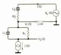
Fig.2. Equivalent circuit of the sine-wave oscillator of Fig.1. With the link closed, the circuit assumes inverters having infinite gain: practical devices have a finite gain (link open).
