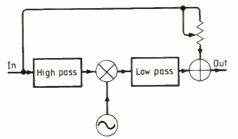
Fig.1. Transposer-type hearing aid. Sound components above 4kHz are superimposed on the 0-4kHz components. This treatment improves intelligibility by adding emphasis to speech consonants and other sounds.
