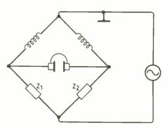
Tightly-coupled inductive ratio-arm bridge circuit, 1928: Blumlein's first invention. The coils were bifilar-wound.
