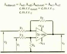
Fig.1. Standard differential amplifier, in which common-mode rejection is heavily dependent on resistor matching.
