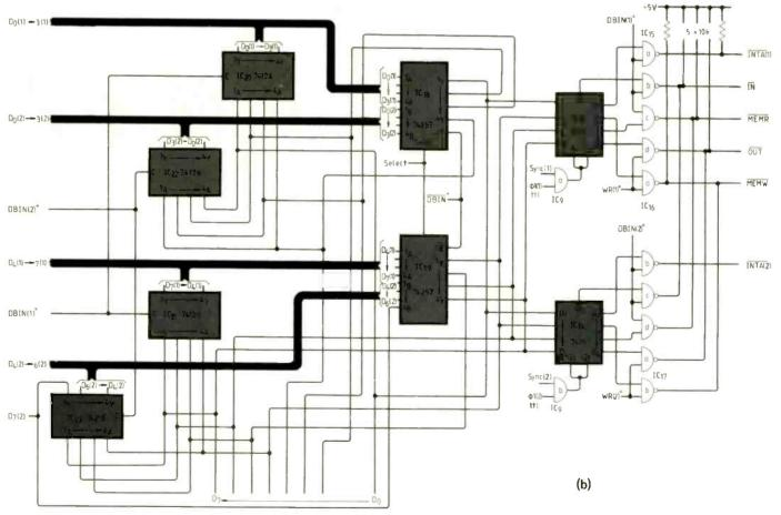
Fig.1. Processor control signals modified to allow two processors to operate together. In this synchronous system,  $\phi 1$ and  $\phi 2$  clocks of each microprocessor are shifted in relation to each other so that the processors access the bus alternately.
