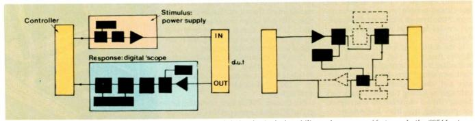
Simple stimulus response test using standard instrumentation (left) has limited adaptability and an excess of features. In the 6954A setup (right) the relationship between cards is not fixed and is determined by the test designer. Features can be adapted by 'rewiring' the blocks, and as the selection of i/o cards is determined by the test designer unnecessary functions can be omitted.
