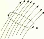
Fig. 5. A journey round the H loop gives the total current through the loop, by Ampère's Theorem.
