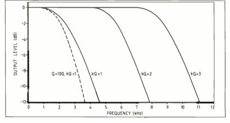
Substituting gives a loss of 10.8 dB, relative to that at  $f_o$ , at  $\pm 6$ kHz. For three i.f.ts, the response will be -32.5 dB at  $\pm 6$ kHz, which agrees well with the chart.
