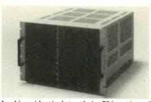
Looking identical to their 53A series of card-based instruments, this 73A series prototyping system is Colorado Data Systems first VXI product. (CDS is represented in the UK by Instrumatic UK Ltd of Marlow, tel. 06284 76741.)
