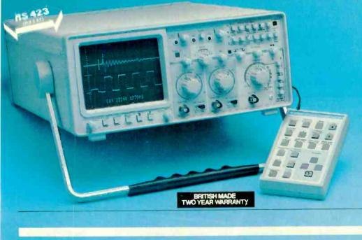
The Gould 1425 Digitising Storage Oscilloscope allows detailed comparison of active with stored waveforms, up to a frequency of 20MHz. Five reference waveforms can be held in the non-voltage memory.
