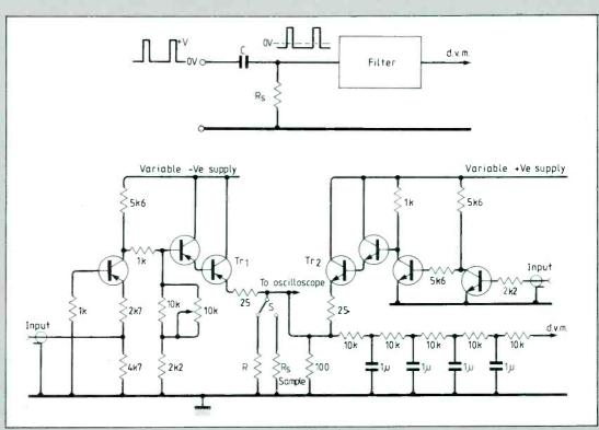
simulates the action of the blocking capacitor, irrespective of period length or duty cycle. Essentially, the circuit consists of two current sources, one positive, the other negative, and so generates a base-line shifted waveform of the type shown in the small diagram.
