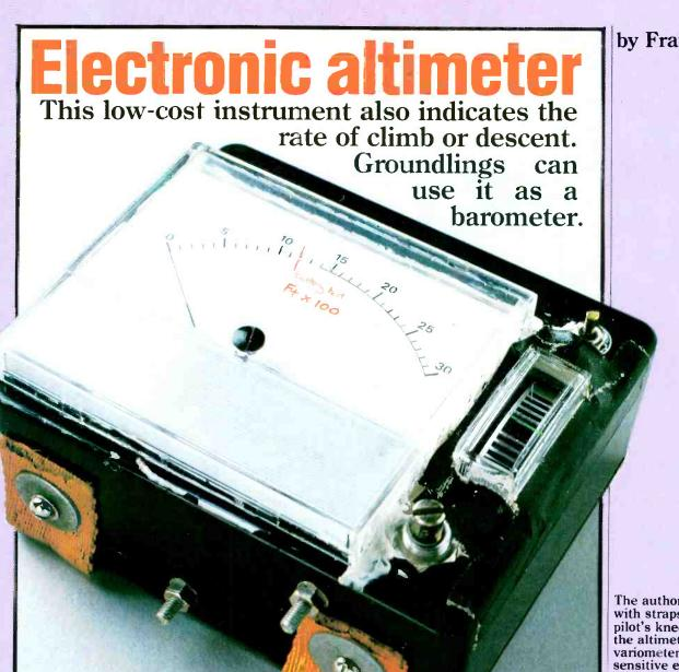
The author's version is fitted with straps for fixing to the pilot's knee. To the right of the altimeter display is the variometer, which is sensitive enough to reach almost to full-scale deflection in the lifts at Quadrant House. The black insulating tape is for vibration-proofing.
