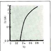
Fig. 4. Graph of  $I_f$  versus  $V_f$  for wire-ended Schottky rated at 1 amp.
