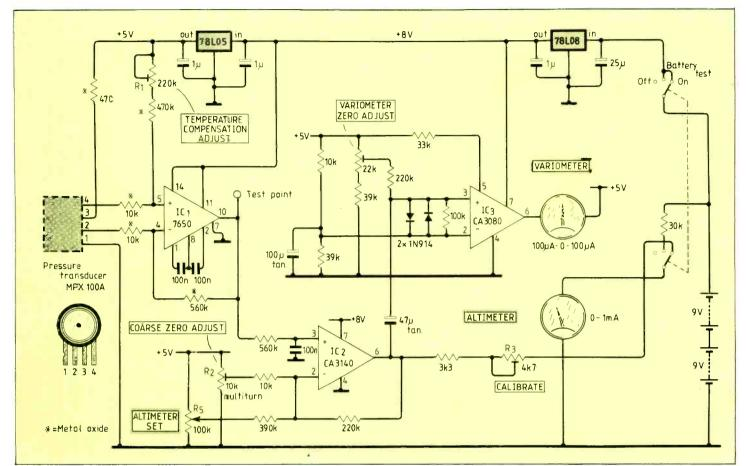
Pressure transducer is a low-cost device intended for the motor industry. Temperature compensation is achieved by the 7650 chopping op-amp and a Wheatstone bridge circuit. 1V/1000ft, which is available to drive a meter movement for altitude indication. The resistor and preset associated with the meter movement are for altimeter calibration purposes. The original design used a 1mA instrument; other movements could be used provided that a suitable scaling resistor chain is provided.
