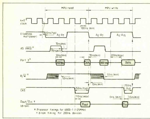
Fig. 5. Printer buffer timing required for dynamic rams. An address must be multiplexed into the rams in two halves on eight lines. Half of the address is latched by the row-address strobe, RAS, and the second half by the column-address strobe, CAS
