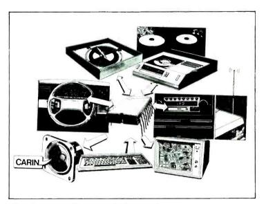
The elements, CD player, dashboard data, electronic compass and computer, that go together to make the Carin route information system, under development by Philips.
