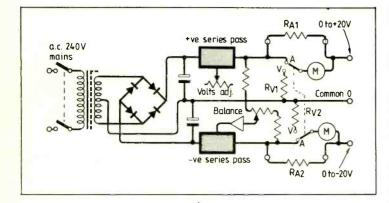
Fig. 1. The diagram shows how positive and negative lines can be obtained from a centre tapped transformer secondary in conjunction with a bridge rectifier. The negative line is referenced to the stabilised positive supply. Simple volt-amp meter switching to monitor the output is illustrated.
