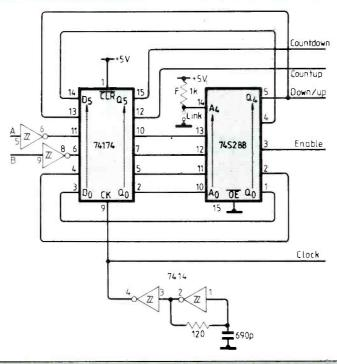
counters are taken through latches since the rom outputs are strictly speaking only valid on the clock edge. For 190/191 counters, the clock input must be connected to the system clock. The two outputs from the shaft encoder (must be t.t.l. compatible) are connected to the A and B inputs of the interface. A further input, F, allows the circuit to
