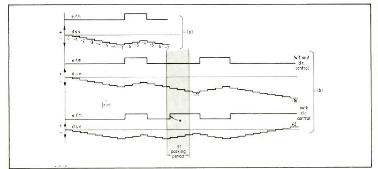
Fig. 3. Digital sum value example calculated from e.f.m. waveform (a). Two successive 14T symbols without d.c. control (upper) give d.s.v. of -16, (b). Additional transition (\*) results in d.s.v. of +2.
