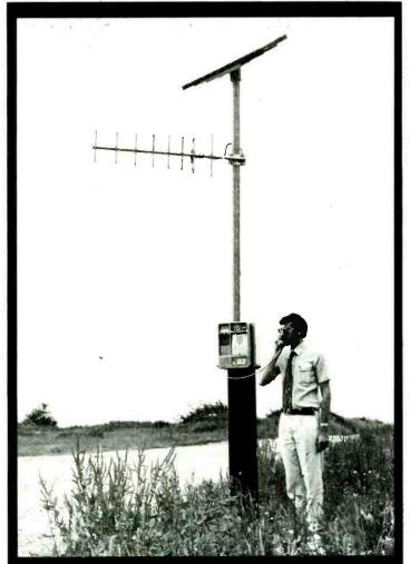
A telephone designed for use in the third world. It is solar powered and communicates by radio, with battery back-up. The equipment can also act as a relay to act as a local link so that remote villages can communicate with each other. Designed by Plessey Radio Systems.
