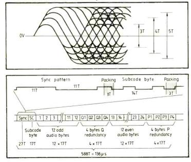
increase and decrease about some average value, which superposes a d.c. level on the readout signal, in addition to a component at the rotational frequency of the disc (3.3 to 9.5Hz) and harmonics thereof. Because the code is d.c.-free, a simple coupling capacitor can be used to remove these effects.
