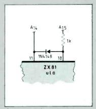
On an issue three computer, the most convenient position for these components is in the u.l.a. socket under the i.c.
