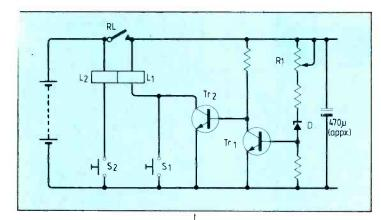
Fig. 2. Low-voltage cut-out circuit is turned on by pressing push-button PB<sub>2</sub>. Relay closes, but  $Tr_1$  clamps base of  $Tr_2$  and holds off the coil L<sub>1</sub> of the relay. If voltage falls below that set by pre-set pot R<sub>1</sub> and zener,  $Tr_1$  releases  $Tr_2$ , the turn-off coil L<sub>1</sub> opens the relay and the load and circuit are switched off. Alternatively, the load may be turned off by pressing push-button PB<sub>1</sub>.
