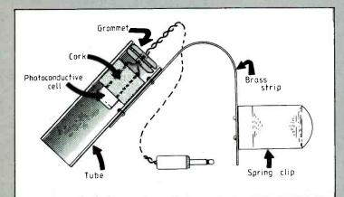
Fig. 5. Tubular holder for photosensitive cell giving a 30 degree viewing angle. Terry clip fixes to enlarger column. have chosen to employ a circuit which is adequate for the purpose in hand, and with no greater complexity or cost than is demanded by its specification, and I have shown the final circuit employed in Fig. 3.
