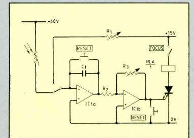
Fig. 2. Basic circuit of timer paper in the correct situation, and press the 'on' button. The enlarger then switches on for a suitable period, and when the photoelectric sensor judges that an adequate exposure has been given, switches the lamp off again. I have had such a system in use in my own darkroom for very may years, since I tend to use a 35mm
