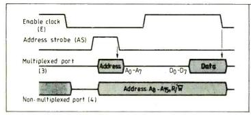
Fig. 3. Multiplexed data/ address signal timings for the 6803 microprocessor. Lines are usually multiplexed in this way to make the most of pins on the i.c. package.
