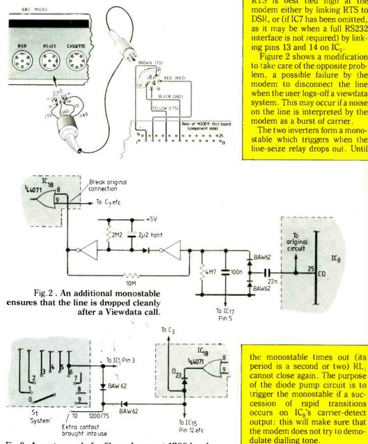
Fig.3. An extra mode for file exchange at 1200 baud.
