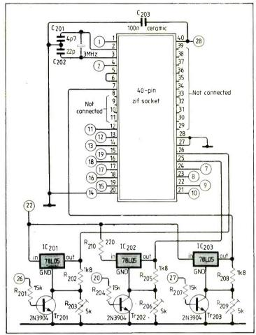
Fig.5. 8741/8/9 microcomputer programming adaptor. Numbers in circles refer to pins on the eprom programmer slave socket into which this adaptor is plugged. These extra components are needed to drive the processor clock and switch voltage levels.
