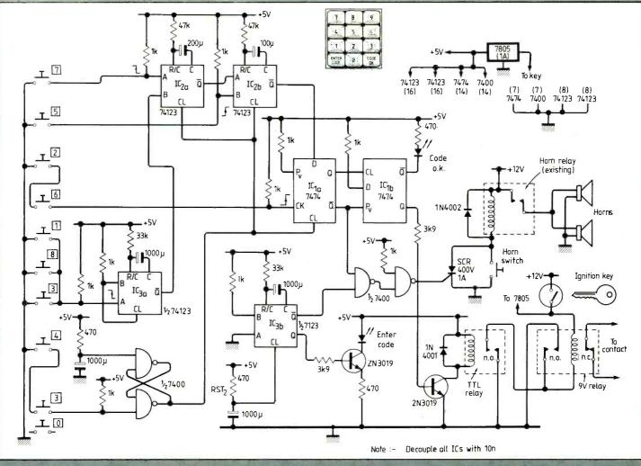
s ort across the ignition contact breaker and the normally-open contact offers a holding path for the 9V relay, even during reset.
