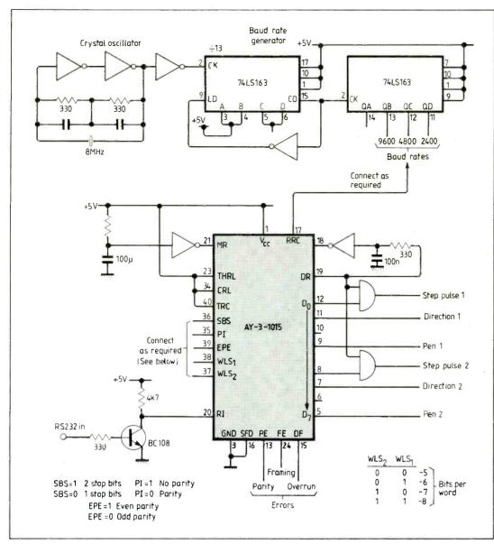
Fig.5. Serial interface for graphics plotter.
