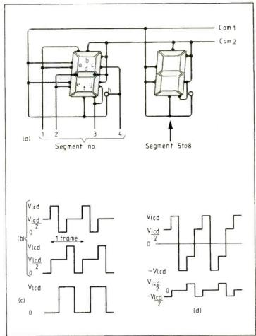
line. Note that this waveform is 180 degrees out of phase with each of the peaks in the common waveforms, resulting in a large polarizing voltage across the four segments, as at (d). If segments 'b' and 'c' must be lit, while 'g' and
