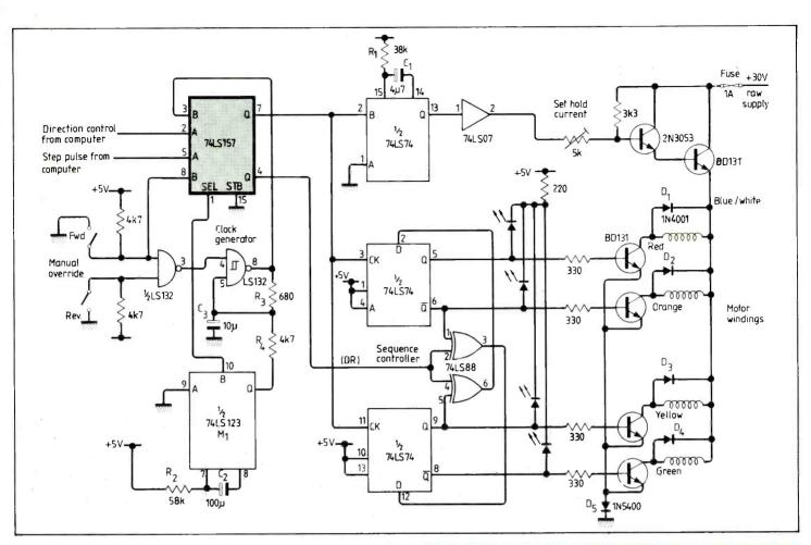
rent of approx 40 mA is found suitable for the 12/24V motors obtained from Stewarts of Reading. These figures are not critical and optimum choice will depend on the mechanical construction of the plotter.
