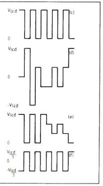
numeric displays. The number of common lines used can get as high as 8, 16 or 32: the limiting factors are how closely the thresholds on the displays can be determind and how well the reference voltages for the steps can be defined. For example, when 16 common lines are used, the voltage across a selected segment is  $1/4 V_{\rm l.c.d}$  and the voltage across a non-selected segment is 11/80
