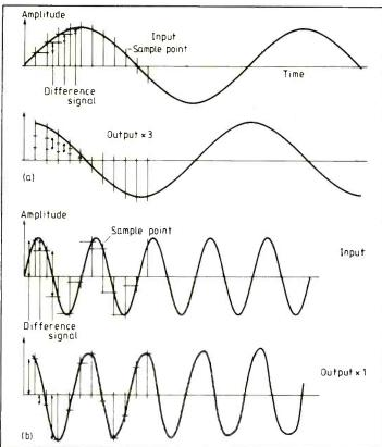
Fig. 4. Effect of differentiation network at higher input frequencies. At (a), input is one-twentieth of clock frequency, giving little distortion. Higher input frequency at (b) increases distortion.
