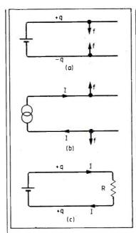
that if a line has  $Z_0 = 100\Omega$ then to establish a current of 1A in the line we need a supply of 100V and the electrostatic attraction because of that cannot be ignored.
