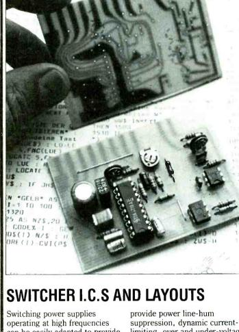
Switching power supplies operating at high frequencies can be easily adapted to provide power at specific current and voltage values. Siemens produce four control i.cs for such supplies and have now made it even easier to design them by the provision of card layouts with the position of all components marked. The four circuits, TDA4700/14/16/18,
