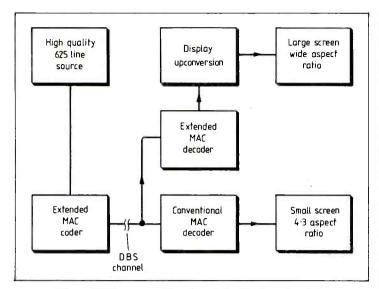
Fig.1. IBA's compatible approach to higher definition television using extended MAC in a C-MAC/packets DBS channel. Other researchers think there is further benefit to be obtained by starting with a high linenumber HDTV picture source and down-converting to 625 lines for transmission.
