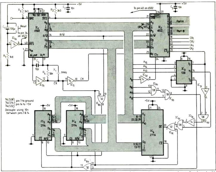
Mimicontroller is designed to emulate BBC microcomputer i/o in control applications. Software is developed and tested using the computer's assembly-language and i/o facilities then transferred to a 2716 eprom for use in Mimicontroller. Ports A and B and control lines of the 6522 v.i.a., top left, act as those on the BBC microcomputer. code control using a computer that they are already familiar with.
