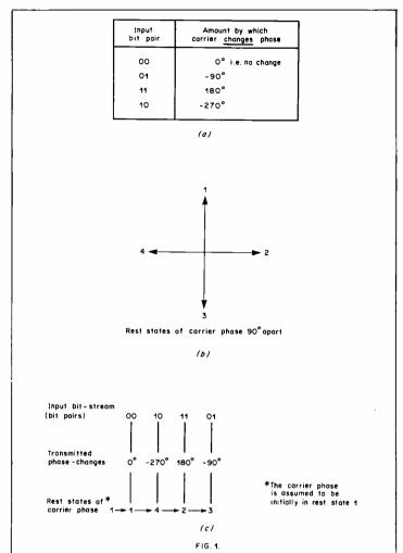
Fig.1. In the differential coding process four bit-pair combinations which modulate the carrier cause it to change phase by the amount shown in the table (a). Carrier has four possible rests state 90 apart (b). An example of carrier rest states adopted for the input bit-pair sequence 00, 10, 11 and 01 is shown in (c).
