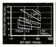
Fig. 2. Longer wavelength laser systems offer the best combination of repeater spacing and data rate, but shorter wavelength l.e.d. systems are less costly.
