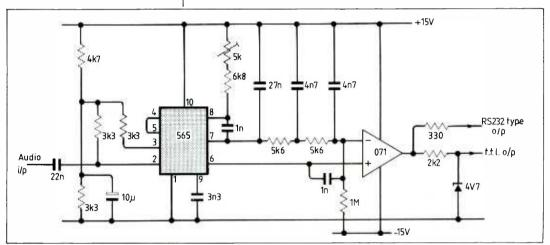
Fig. 7. F.s.k. demodulator, using Signetics 565 phase-locked loop.
