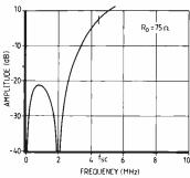
Fig. 94. Amplitude performance of the chroma path filter.
