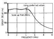
Errors caused by rounding components of Fig.87 (bottom circuit) to preferred values are shown by the group delay response above (Fig.88).
