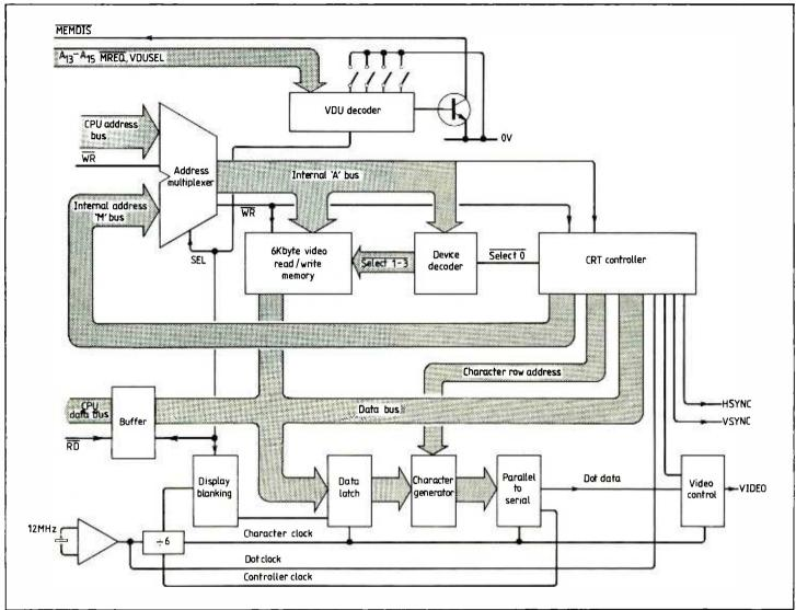
Designed chiefly for fast clear high-density text display, the monochrome v.d.u. section of SC84 is memory mapped and uses the pipelining technique. Output is separete video and sync. signals in either polarity.
