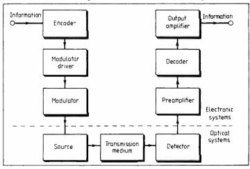
Fig. 1. Principal components of an optical communications system.
