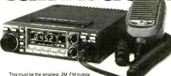
available today, measuring only 38mm H x 144mm W × 177mm D. It has all the features that you probably require included in this microprocessor controlled unit. In addition, if you feel lonely and can't find anybody on the band, just press "speech" and the optional built in speech synthesizer will tell you the frequency you are tuned to. This is a boon to the blind operator or to those that tuck their rigs out of sight.
