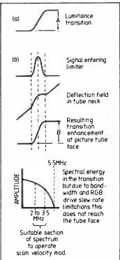
Fig. 99. Example of waveforms occurring in a scan-velocity modulation circuit.
