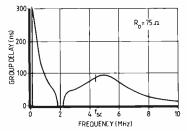
Fig. 95. Group delay response of the high-pass chromafilter.
