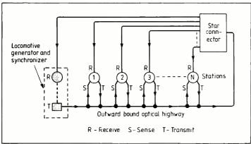
Fig. 6. D-Net optical lan | municate with each other. combines a data highway and a star return, making it more like an open ring.
