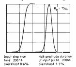
Group delay ripple and other losses in performance caused by using preferred capicitor values are shown in these pulse-and-step test results (Fig.89).
