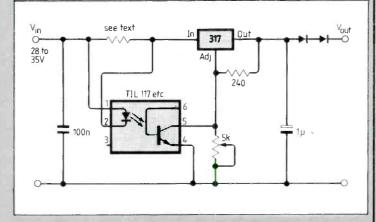
1.5V above control voltage to limit output current under a dead short. Power and resistance ratings of the series resistor are chosen to suit the required current limit and the diodes must
