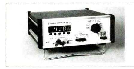
This 4½ digit autoranging digital multimeter measures a.c. and d.c. volts and current, resistance and dBm. A.C. measurements and dBm are true r.m.s. with a frequency response of 45Hz to 20kHz.
