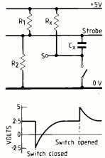
Fig. 1. Outline of the keyboard's interrupt generator. Closing or opening the switch causes the voltage on the strobe rail to act as shown. Each pulse causes an interrupt.
