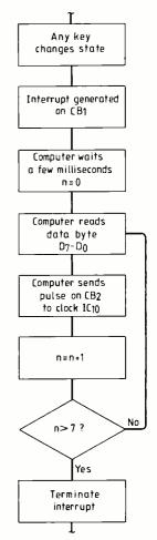
At switch on, the counter is set to zero and its synchronism is checked each time the keyboard is read. The delay allows for key bounce and for the fact that is impossible to play all the notes of a chord simultaneously.
