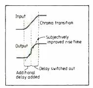
Fig. 102. Waveforms showing chroma edge enhancement by delay switching.
