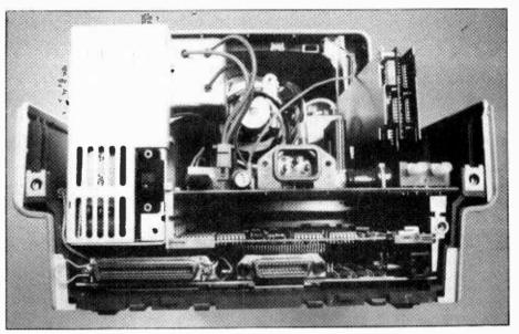
A 68000-based computer with half a megabyte of ram surrounds the c.r.t. in Hewlett Packard's Series 200 Model 16. Basic for this engineering system takes up 277K of memory, but is fast as some compilation takes place when the program is entered.
