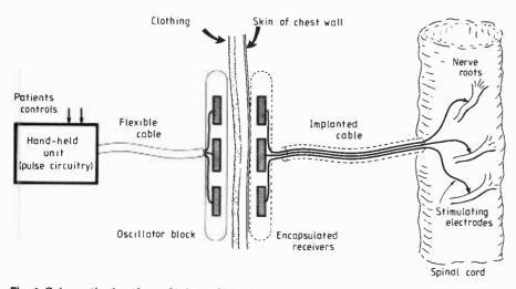
**Fig. 1.** Schematic showing principle of bladder control prosthesis. The implanted part of the stimulator comprises a receiver unit, a flexible cable and an assembly of stimulating electrodes.
