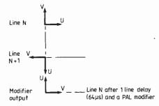
**Fig. 15.** PAL modifier chroma phase relationships (above) for line N+1 and line N emerging (at time of N+1) from line delay and modifier. Phase of  $2f_{sc}$  feed sets output phase of modifier. (b) shows improved methods of decoding PAL signals using a modifier in the comb (right).
