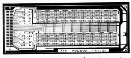
Fig. 21. Artwork for a memory board. All bus interconnections were drawn by the plotter.
