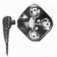
**Fig. 3.** (a) Complete three-receiver implant after encapsulation in silicone rubber. The three plugs mate with sockets on the implanted cable. (b) The corresponding oscillator block as used by the patient.
