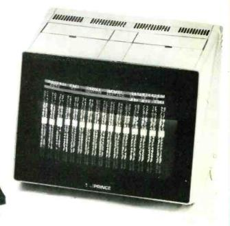
The new microprocessor controlled EP8000 Emulator Programmer will program and emulate all EPROMs up to 8k x 8 sizes, and can be extended to program other devices such as 16k x 8 EPROMs, Bipolar PROMs, single chip microprocessors with external modules.
