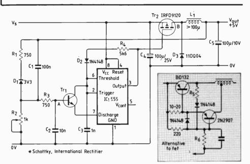
of 0.5mm wire wound on a Neosid 14mm powdered-iron toroid was used for the prototype output choke. Copper on the top surface of the p.c.b. is soldered to the fet drain terminals to act as a heat sink.
