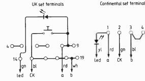
Modifications for connection of UK or Connection to public network for UK (left) and Continental sets. For UK sets, remove straps 5, 6, 17 and 18 in telephone. Change around green/white strap in terminal block and connect blue wire to tag five in telephone. In Continental telephones, change green wire from point two to point five and connect 'a' to the socket ground strap.
