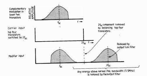
top of a letter T will bring the notch on, and if the tops of Os and other rounded letters appear on the same tv line, the notch will still be on and dot crawl will not occur around these edges although the amount of energy associated with a rounded top surface would not have been Fig. 19. Modifier chrominance signal envelopes show reversing of the sidebands as the carrier input is high w.r.t. the video signal.
