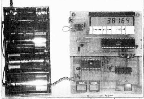
**Fig. 1.** Microprocessor-based sampling frequency meter. If the number of pulses counted in the ten-second measuring interval is greater than 65,535 "HI ----" is displayed. The i.c. to the left of the display (not included in the circuit diagram) is a small test oscillator, feeding pulses to the input of the circuit.
