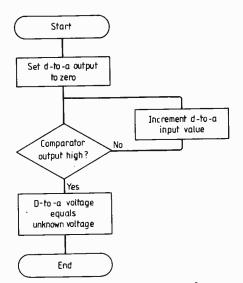
**Fig. 5.** Flow diagram for simple analogueto-digital conversion. In this method, output from the converter is increased one step at a time from zero until the comparator switches.
