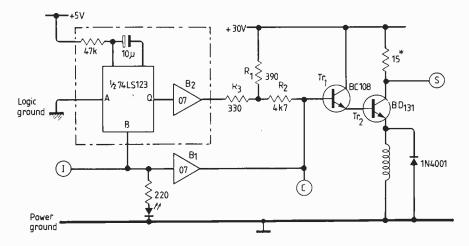
Fig. 2. Motor driver circuit. The enclosed section is required only once for each motor.
