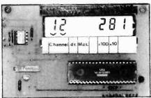
**Fig. 2.** Contents of channel 12: input has spent 281 units of ten seconds in the range of channel 12 – 36,000-38,999 in this case. Channel contents rise from 0 to 99,999, after which 10,000 is displayed, with the arrowed annunciator pointing to ×10, etc.
