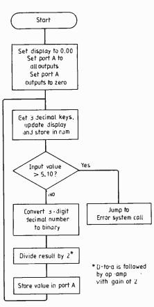
Fig. 3. Picotutor contains a program for converting three decimal digits entered on the keypad to binary form. This binary value is sent to the digital-to-analogue converter board through port A.
