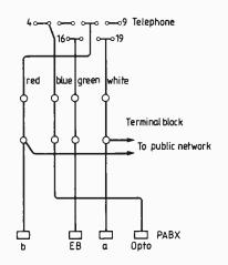
Connection to public network for UK (left) and Continental sets. For UK sets, remove straps 5, 6, 17 and 18 in telephone. Change around green/white strap in terminal block and connect blue wire to tag five in telephone. In Continental telephones, change green wire from the point two to point five and connect 'a' to the socket ground strap.
