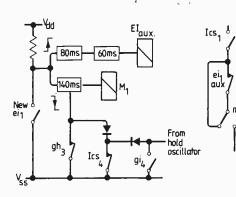
Circuit changes in line interface and timing diagram for delayed dial pulse and muting sequence.
