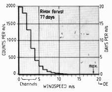
*Fig. 6.* Results from 11 weeks of windspeed measurement at Rivox Forest (see text).
