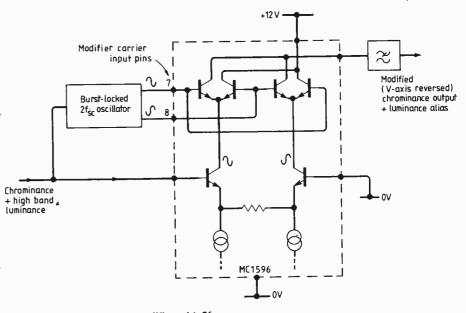
**Fig. 18**. Pal chrominance modifier with 2f<sub>sc</sub> oscillator locked to incoming burst using MC1596 i.c.
