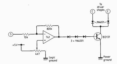
Fig. 4. Driver protection circuitry. RV1 sets maximum output current.
