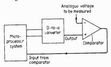
Fig. 4. Most common analogue-to-digital circuits use a digital-to-analogue converter and comparator as shown here.
