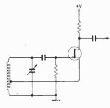
**Fig. 1.** Output level of this simple oscillator varies with frequency and the tapped coil makes range-switching complicated.
