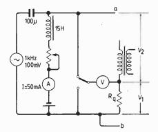
Test circuit for determination of rg value. Connect to line interface and select rg for  $V_1 = V_2$ . Impedance is 600 ohms  $\pm 20\%$ .
