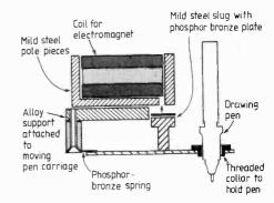
Fig. 14. Cross-section of pen lifting mechanism. More than one can be used to provide different coloured pens.
