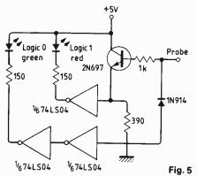
A basic logic probe circuit also could be incorporated into the simulator. A suggested circuit is shown in Fig. 5, the required gates being available in  $IC_8$ .
