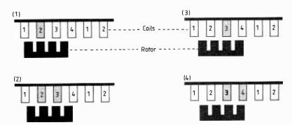
**Fig. 1.** Internal configuration of a typical four-pole stepper motor. The sequence shows how the half stepping is achieved.
