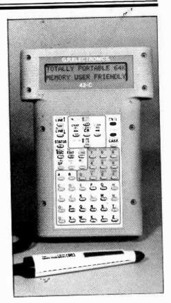
Nominally a hand-held terminal, the 42-C from G.R. Electronics has many inbuilt functions associated with a portable computer. (See News at Compec)
