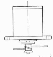
Fig. 13. Shows the pulley and thread arrangement for one of the stepper motors.
