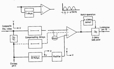
Fig. 20. Combing across adjacent lines with the aid of the PAL decoder (page 54, bottom). Block diagram of the PAL decoder is for Mullard one-chip decoder TDA3561A (or 3560).Components within broken-line area are replaced by diagram on p.54; pin 10 is luminance input, pin 3 chroma input.
