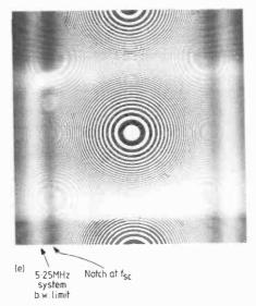
the top two traces of (b) the carrier frequency has been shifted slightly by removing the 25Hz term and changing  $\frac{1}{4}$  to a  $\frac{1}{2}$ in the subcarrier expression, the result being that the subcarrier is now stationary with respect to line timing. You can now see that phase (group delay) in the gaussian chroma bandpass filter and the cheap DL60 chroma delay line, figure (c), reduce the ability to obtain cancellation at the vertical colour transition where the side-
