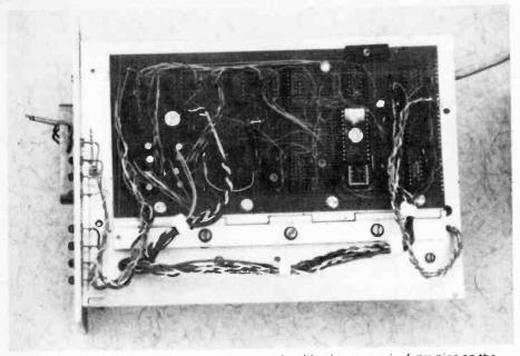
**Fig. 10.** Controller p.c.b. Interconnections are made with wire-wrap wire from pins on the component side.
