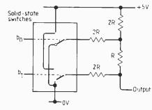
**Fig. 1.** Basic digital-to-analogue converter circuit. Two digital input bits,  $b_0$  and  $b_1$ , are converted to one of four output levels using an R-2R network. Bit  $b_0$  is the least-significant digit of a binary word and  $b_1$  is the most significant.
