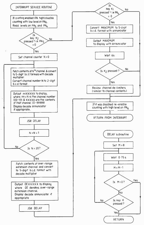
**Fig. 5.** Flow chart of interrogation mode of operation. Key switches K1 and K2 are diode or-ed to the m.p.u. interrupt request line. If K1 is closed, the maximum input value is displayed briefly. Closure of K2 initiates a cycle through all 21 channels, displaying briefly the contents of each. Holding K2 closed accelerates the scan. Note that an interrupt can be pending, even though neither switch is closed.
