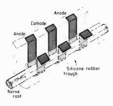
**Fig. 5.** Construction of electrodes for one nerve root. The middle platinum foil electrode is a cathode while the outer ones (connected together) form an anode.
