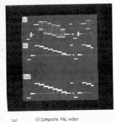
(i) Composite PAL video in 100% colour bars (ii) Luminance output using modifier and one chroma line delay
