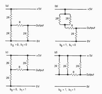
Fig. 2. Equivalent circuits of the network shown in Fig. 1 for the four input permutations.
