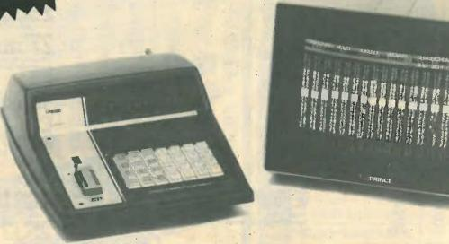
The new microprocessor controlled EP8000 Emulator Programmer will program and emulate all EPROMs up to 8k x 8 sizes, and can be extended to program other devices such as 16k x 8 EPROMs, No personality cards/characterisers required. Bipolar PROMs, single chip microprocessors with external modules.
