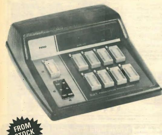
Checks, Programs, Compares up to 8 devices simultaneously Handles all EPROMS up to 128K with no personality modules
