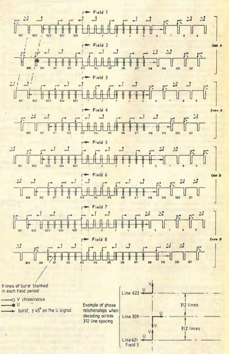
Fig. 13(a). Full eight-field sequence over which the colour subcarrier phase sequence repeats. The pairs of rounded vectors show U/V phases across field and picture intervals. (From EBU statement D22-1979).
