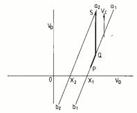
**Fig. 11.** Transfer characteristic of class 3 op-amp comprises a series of parallel lines, two of which are shown, corresponding to the projection of lines such as  $a'_2b'_2$  on the plane
