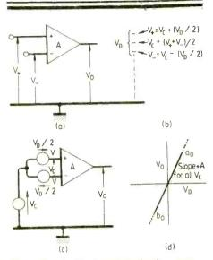
**Fig. 1.** Symbol for 'quasi-perfect' op-amp uses thickened line to denote non-ideal behaviour (a). Signals  $V_+$  and  $V_-$  can be split into common-mode component  $V_C$ and differential component  $V_D$  (b). Redrawn version (c) emphasizes significance of  $V_C$  and  $V_D$ . This class 1 opamp is completely specified by transfer characteristic (d).
