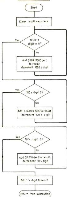
List 9 is a program example for converting 2748 to binary for representation in hexadecimal form. First POINT and POINT+1 are set up with the decimal value then the index register is loaded to point to result location 60. Subroutine BCDBIN is then called to convert the number to decimal and return control to the monitor. Examination of locations 60 and 61 using the memory-open key should Table 1. System calls.
