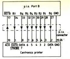
Fig. 5. Program will drive a Centronicscompatible printer to provide hard copy of messages.
