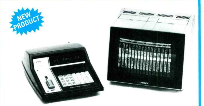
The new microprocessor controlled EP8000 Emulator Programmer will program and emulate all EPROMs up to 8k x 8 sizes, and can be extended to program other devices such as 16k x 8 EPROMs, Bipolar PROMs, single chip microprocessors with external modules.
