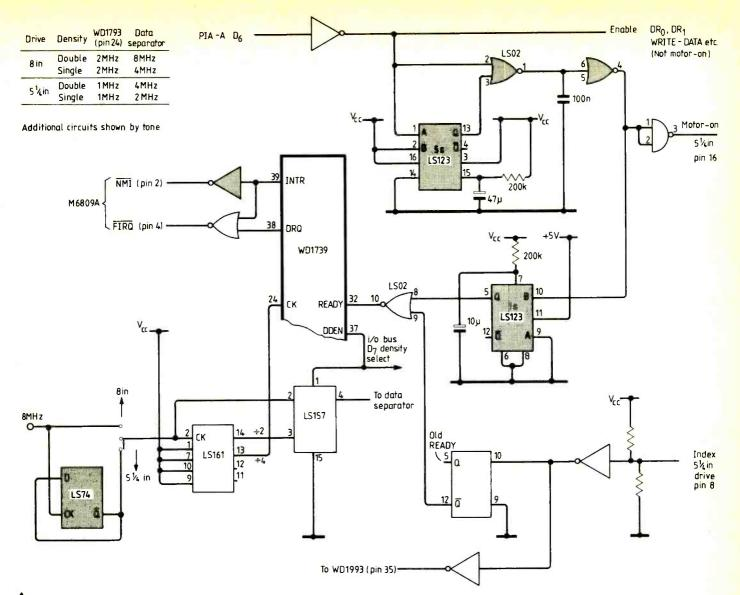
Disc interface modification speeds up overall access time by keeping the drive motor running for five seconds after the computer tells it to switch off. This significantly reduces the effect of a one second delay required for the motor to start up since disc-access operations tend to come in bursts.
