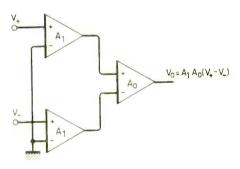
**Fig. 3.** Common-mode signal is rejected due to identical magnifications, though the signal paths are different, as indicated.
