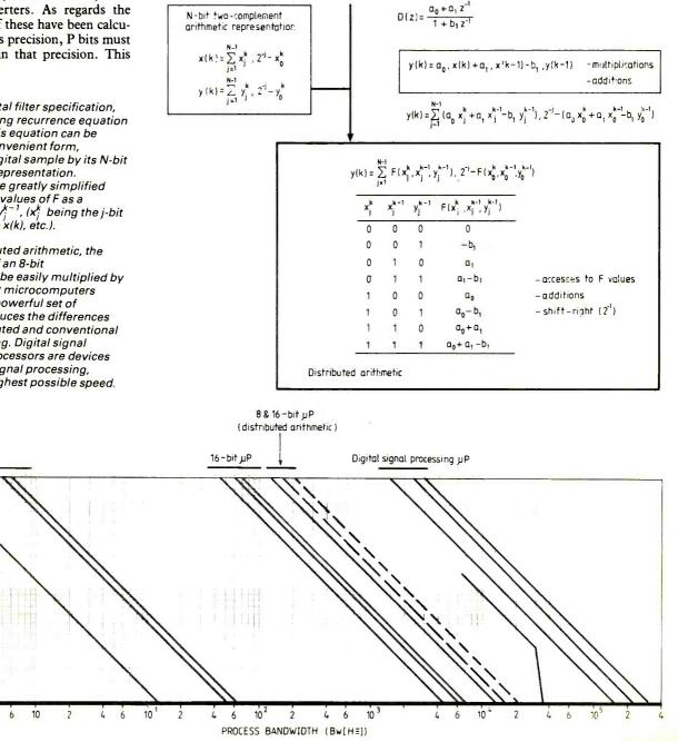
The microcomputer services can be evaluated when implementing a secondorder filter; on the other hand, the microcomputer maximum processing speed for an nth-order filter will result from extrapolation as follows:
