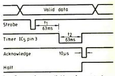
In a Centronics parallel interface a strobe pulse from the computer signals that valid data is available. The computer must receive an acknowledge pulse from the peripheral device before any further data transfer can take place.
