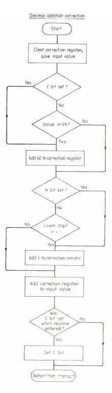
greater than 99 so 60 is added and the halfcarry bit is set so a further six is added. With correction of 66 added, result E2 becomes 148, i.e. 48 with the carry indication set.
