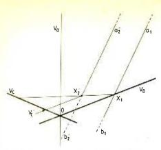
**Fig. 9.** 'Three dimensional' characteristic plane displays functional dependence of  $V_0$  on the two dependent variables  $V_D$  and  $V_C$ . As  $A_D$  and  $A_C$  are constant, equation for  $V_0$  is the plane surface defined by two parallel lines.
