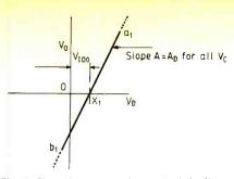
**Fig. 4.** Class 2 op-amps have straight-line transfer characteristic with intercept on the  $V_D$  axis, equal to the input offset voltage,  $V_{100}$ , arising simply from small differences in the active devices.
