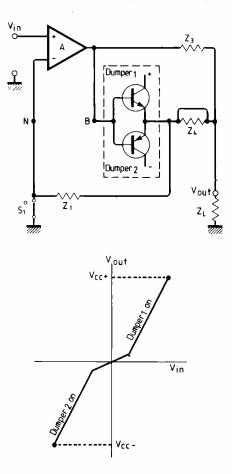
**Figs 2 & 3.** When Z<sub>3</sub> is present in this class B output circuit the output transistors could be called "current dumpers" just as in Fig. 1. Transfer function is shown bottom at Fig. 3 impedance will be very small. In terms of algebra this bridge model is very powerful, and also in terms of intuition. Fig. 5 with an inductor at  $Z_4$  and a capacitor opposite shows that the basic idea is just to balance a traditional LC bridge, according to  $L=R_1R_3C$ .
