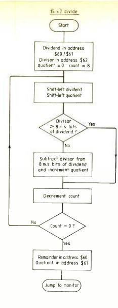
most-significant bits of the dividend without causing a borrow. If the divisor can be subtracted the corresponding bit in the quotient is one, if not, the bit is zero. Dividend and quotient are correctly aligned by shifting them left one bit before each trial subtraction.
