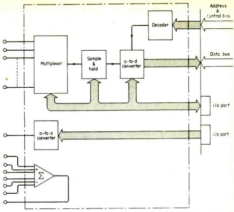
**Figs 1 & 2.** Functional scheme of the analogue interface (above) together with its detailed system performance (below).
