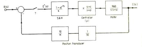
bilinear transformation a lag-lead controller has been programmed in the microcomputer, with the transfer function
