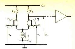
**Fig. 7.** Typical circuit for which commonmode rejection is quantitatively given by the ratio of the mean amplifier gain to the difference in gains.
