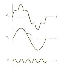
**Fig. 2.** Common-mode gain for class 1 opamp is zero so if  $V_+$  and  $V_-$  have the form indicated,  $V_0$  is an amplified version of  $V_D$ only.
