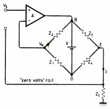
**Fig. 5.** Modelling the dumpers of Fig. 1 as a voltage source V<sub>1</sub> Vanderkooy & Lipshitz redraw the circuit as a bridge.
