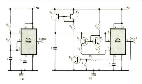
$Tr_1, Tr_2$ . In this case we have to introduce resistors<sup>2</sup> in the emitter circuits of  $Tr_1$  and  $Tr_2$  as in  $Tr_3$  and  $Tr_4$  (the emitter resistor of  $Tr_1$  in this case can be used for frequency control as well). For the current source  $Tr_3, Tr_4$  the resistor  $R_3$  and  $R_4$  are necessary to compensate for the saturation voltage of the 555 inner switch (this voltage can be as large as 0.1V).
