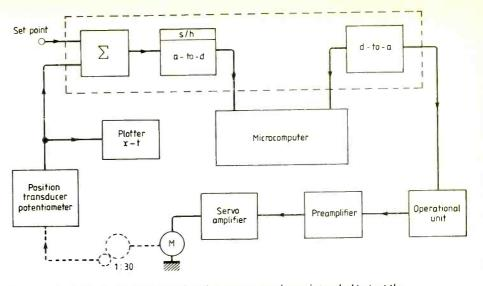
**Fig. 9.** Schematic representation of a laboratory experience intended to test the performance of the equipment described in Fig. 3 in the position control of a d.c. servomotor.
