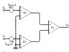
**Fig. 6.** Unequal magnifications of  $V_+$  and  $V_-$  together with offset voltage are taken into account in this class 3 equivalent circuit.
