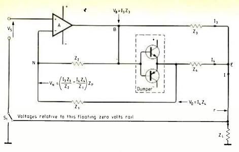
**Fig. 1.** Walker's basic current dumping circuit. It is a standard class B circuit with elaboration of the feedback network, and floating signal source.  $(Z_p \text{ means } Z_1/Z_2)$
