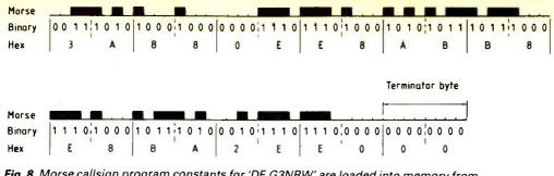
*Fig. 8.* Morse callsign program constants for 'DE G3NRW' are loaded into memory from location 0FD4.
