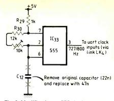
Fig. 2. Modification to 555 clock generator to run the uart at 44.45/50baud. Component numbers refer to those in the Nascom 1 manual.
