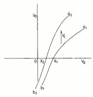
Fig. 14. Family of Class 4 transfer characteristics associated with Fig. 13 obtained by projection onto the plane  $V_C=0$  are now neither straight nor parallel.
