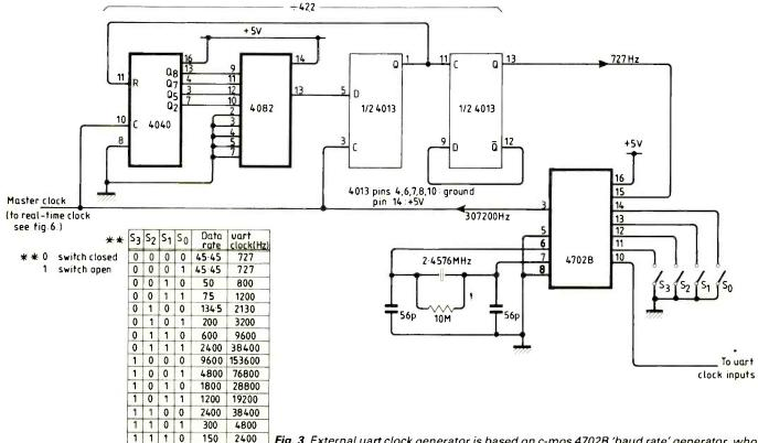
Fig. 3. External uart clock generator is based on c-mos 4702B 'baud rate' generator, whose output frequency is selected by switches  $S_0$  to  $S_3$  – see table.
