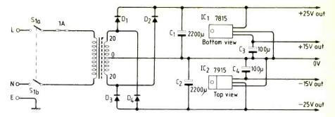
Fig. 2. Circuit diagram of power supply. Toroidal transformer from RS Components.
