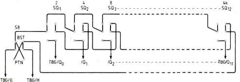
Fig. 5. Switching for tone-burst gating. Circuit connects to G and H in Fig. 4.
