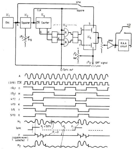
Fig. 3. Basic circuit of tone-burst switching, with waveforms.
