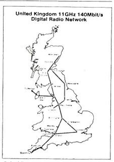
Coinciding with the London to Birmingham Mercury project, BT open 34Mbit/s optical fibre and 140Mbit/s digital microwave links.
