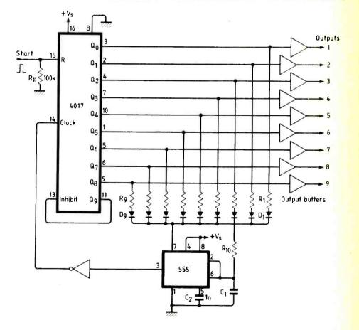
Pin 5 of the timer, shown de-coupled to ground through  $C_2$ , can be used as a modulation input to compress or expand all output times simultaneously, i.e. scale factor. Output buffers can be selected according to requirements or omitted entirely if driving other cmos logic.
