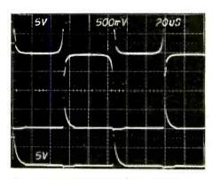
**Fig. 6.** Secondary output  $(S_X - |C1, pin 1 - upper trace)$  and phase sensitive detector's control signals: middle trace:  $|C_1, pin 5$ . lower trace:  $|C_1, pin 6$
