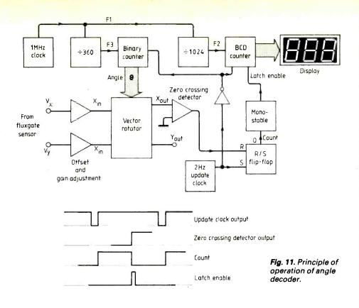
Fig. 13. Angle decoder: control logic and display.
