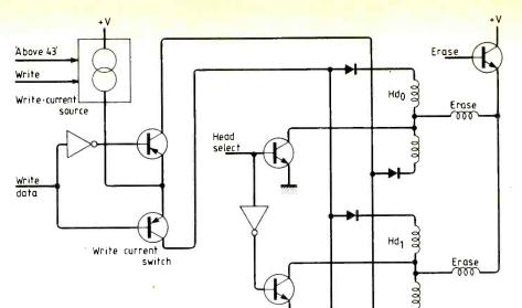
**Fig. 8.** Typical write circuit from a doublesided disc drive with head-select matrix. During writing, the erase poles are energized by switching power to a fourth head connection. 'Above 43' refers to higher cylinder addresses and is a signal used to reduce write current at the inner tracks where the writing density is higher.
