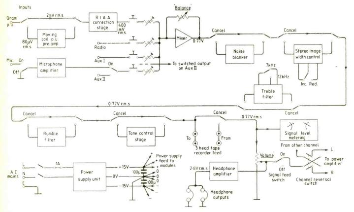
sensible proposition to envisage the preamplifier modules operating at the 0dB level (referred to 0.774V r.m.s. in  $600\Omega$ ), employing this type of op. amp. gain block, to give both an adequate overload margin and a negligible contribution to total circuit noise and distortion. (The gain characteristics of the power amplifier unit were chosen to give maximum output at 0.774 V r.m.s. input).
