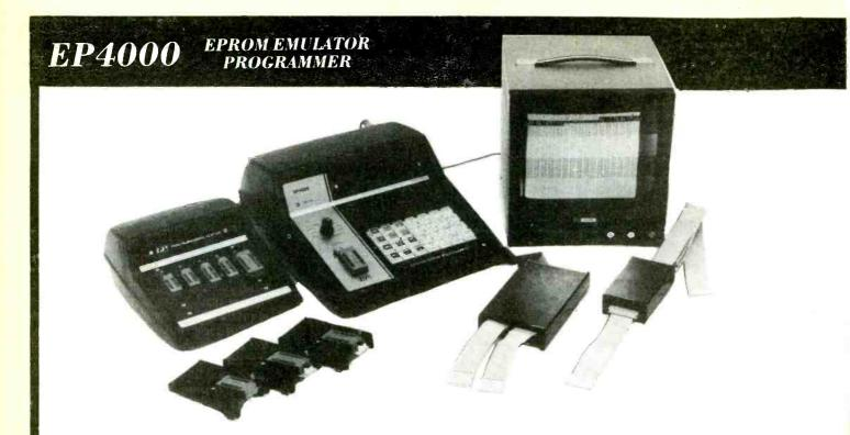
The microprocessor controlled EP4000 will emulate and program all the popular EPROMs including the 2704, 2708, 2716(3), 2508, 2758, 2516, 2716, 2532 and 2732 devices. Personality cards and hardware changes are not required as the machine configures itself for the different devices. Other devices such as bipolar PROMs and 2764 and 2564 EPROMs are programmed with external modules.
