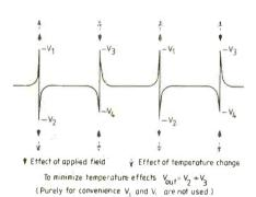
Fig. 5. Effects of temperature versus applied magnetic field on secondary waveform.
