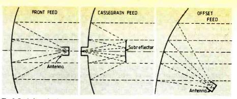
Fig. 3. Basic front-feed parabolic antenna and two variations. Cassegrain feed is used for •antennas with unfavourable f/d ratios, but subreflector obscures part of the dish, causing problems with small antennas. The offset feed gives no blocking problems but is difficult to construct as the dish is neither symmetrical nor parabolic.
