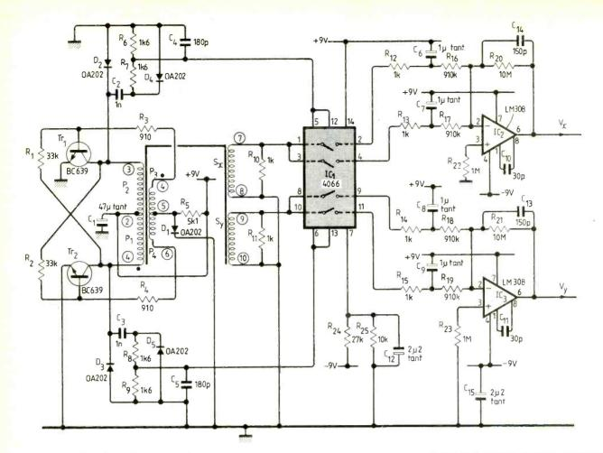
component perpendicular to the plane of the appropriate secondary coil. In practice, the effect of applying an external field is to change the amplitude of the pre-existing secondary voltage spikes. The amplitude of these spikes is also quite strongly temperature dependent. Figure 5 illustrates how the effect of an applied field is separated from the effect of temperature.
