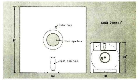
**Fig. 2.** A slot in the disc's protective envelope allows the read/write head to access the disc surface, and a further small aperture lets the photo-electric index sensor detect a small hole in the disc for signalling one revolution. Various types of micro-floppy disc-drives are appearing, one of which has a rotary positioner to keep costs down. Micro-disc shown is for the Sony SMC-70. Relative sizes shown are approximate.
