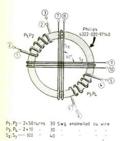
Fig. 3. Toroid windings.
