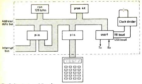
Fig. 7. A test set consisting of a p.c.b. and a control module.
