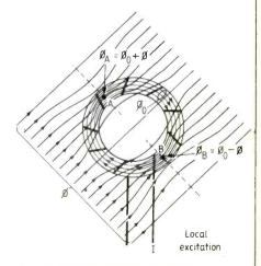
Fig. 1. Flux interference pattern.
