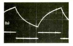
Fig. 8. Response of equalizing circuits to square-wave input. Passive circuit of Fig. 5(a) produces curve (a); curve (b) is output of system when conventional series-feedback equalizer is used; series/shunt circuit chosen and shown in Fig. 6 produces trace at (c).
