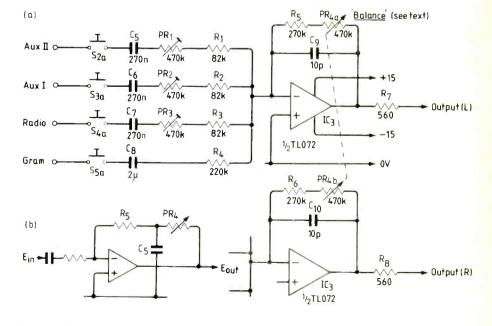
**Fig. 3.** Input mixer and buffer stage is at (a) Careless wiring of balance control could introduce stray capacitance, resulting h.f. lift configuration at (b).
