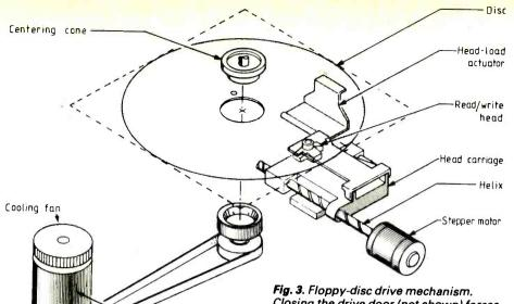
rig. 3. riopp-use arive mechanism. Closing the drive door (not shown) forces the moving disc hub (here the upper hub) toward the fixed driving hub to both grip the disc and centre it by means of a location taper.
