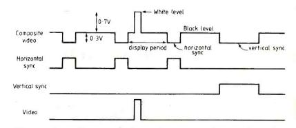
Fig. 1. Video waveforms. Top is compositevideo signal, while other three waveforms,
