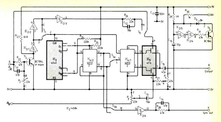
G goes positive it will either set or maintain toggle output J at logic 1. Each positive transition of H will reverse the status of the first toggle, but reset will occur as soon as there is a positive transition at G.
