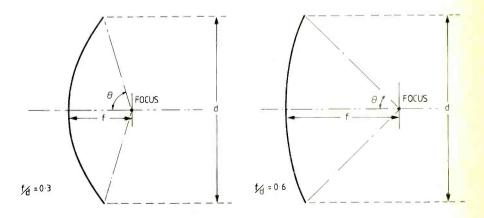
**Fig. 1.** Two dishes with the same diameter but with different focus-to-diameter ratios. Dishes with a low f/d ratio usually give a high degree of side-lobe suppression while those with higher f/d ratios of around 0.5 are designed for optimum forward gain.
