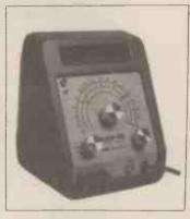
has three ranges covering rates from 0 (off?) to 16000 flashes per minute. When used without external triggering, the flash rate can be set to within 1% at certain points on the continuously-variable scale using a mains-frequency dependent calibration method; a t.t.l. compatible output is provided. Maximum light output of the unit is 10W and mains inputs from 110V to 240V a.c. can be used. Firnor Misilon, Unit 49, The Maltings, Stanstead Abbotts, Herts. WW310
