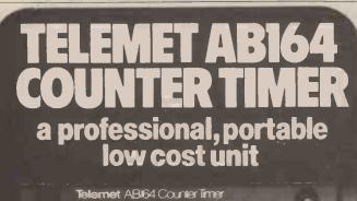
3 frequency ranges DC to 180MHz with 1 Sec gate including phase locked loop 1Hz-1KHz providing 0.01Hz resolution within 10 seconds.
