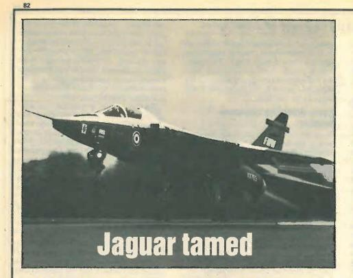
Said to be the first aircraft in the world to fly solely under the direction of all-digital, quadruplex, fly-by-wire controls, the Sepecat Jaguar made its first flight in this form at British Aerospace's Warton aerodrome on October 20, 1981.
