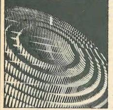
Fig. 1. One of the lens aerials constructed by the new method.
