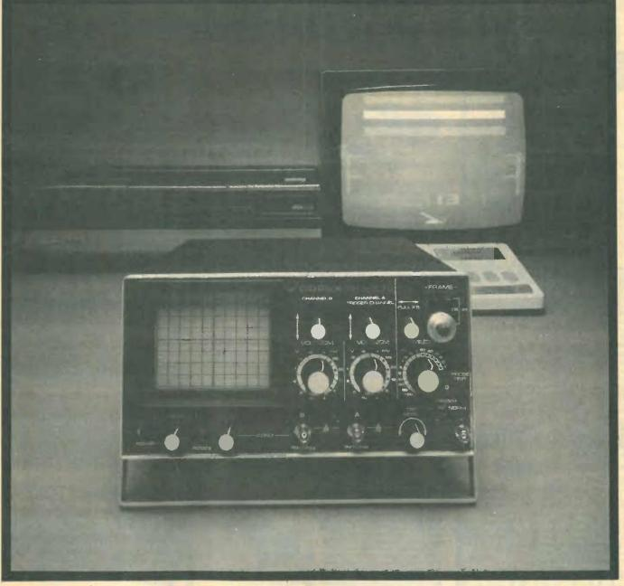
The 14D-10V is a dual trace 10MHz. oscilloscope with active TV sync separator and line selector specifically designed for the servicing and alignment of video cassette and disc recorders, colour television and video games.
