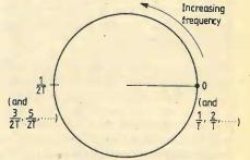
Fig. 3 The circular frequency axis of sampled systems
