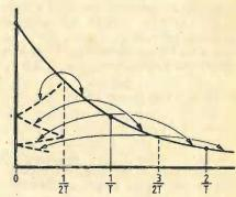
Fig. 2 How sampling "folds" the frequency spectrum
