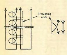
Fig. 6. The idea of a processing node, involving both the slow line (left) and fast line (right) and allowing more advanced operations than simply "read" and "write".
