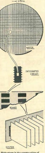
electronic equipment from the conventional silicon chip.
