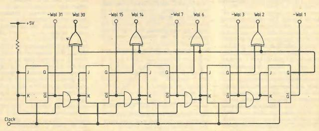
Fig. 4. By adding inverters and four excusive- or gates triangle and sawtooth waveforms can be synthesized.
