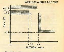
Fig. 8 Specifications of the pre-sampling filter for telephone-quality speech
