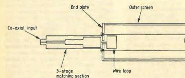
Fig. 4. Cross-section of dipole-mode launcher using magnetic coupling.
