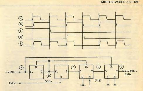
4MHz master clock or a 31250Hz double line frequency is easily produced.
