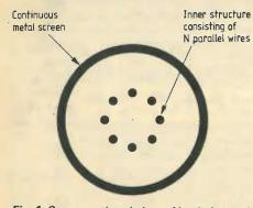
Fig. 1. Cross-sectional view of basic form of dipole-mode cable
