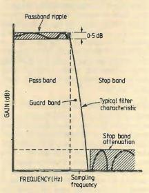
Fig. 7 General characteristics of the presampling filter
