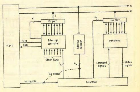
interrupt systems depends only on the peripheral and not on whether vectored or nonvectored interrupts are being used. Furthermore, because the microprocessor response consists of i/o signals, whose nature does not vary greatly from microprocessor to microprocessor, the interface hardware is almost identical for all types of microprocessors.
