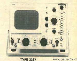
DC-30MHz Bandwidth 11.7 ns Risetime 5mV/div sensitivity Signal Delay Algebraic addition and subtraction
