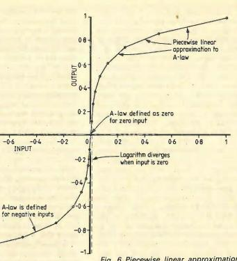
Fig. 6 Piecewise linear approximation to the A-law input/output relationship
