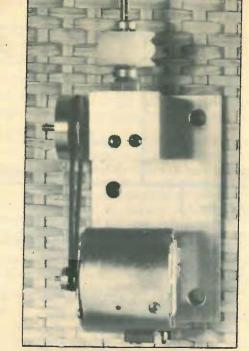
One way of achieving faster traverse is to use a second, inexpensive, motor with slipping clutch.
