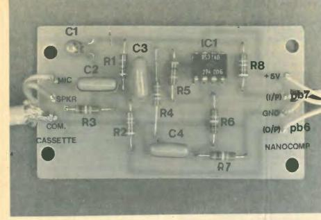
Fig.3. Layout and component placement for the cassette interface.
