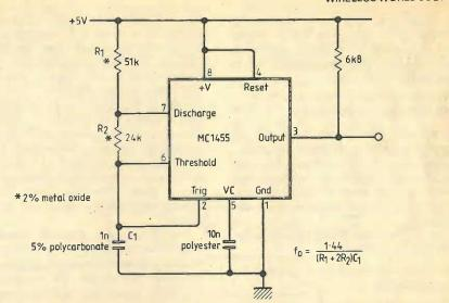
Fig. 6. Clock generator frequency is set to 2<sup>5</sup>f for testing dynamic operation of Fig. 5.
