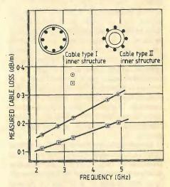
Cable type I in dipole - mode propagation
