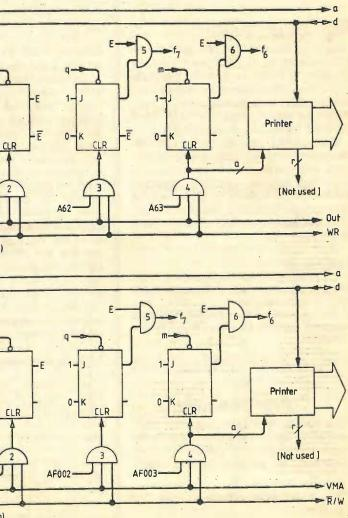
shown in Fig. 6(a). Switch *m* is connected directly to the clock terminal of flip-flop 6, allowing it to be set each time switch m is pushed and released. Similarly the output of the sensor is connected directly to the clock terminal of flip-flop 7, which also allows it to set each time the sensor generates a pulse.
