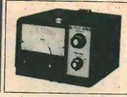
AG203 Low Distortion Oscillator — 10Hz to 1MHz in 5 ranges — < 0.1% distortion — very flat O/P to 7V r.m.s. sinewave from 600 ohms, squarewave 10V pp - Ext. Sync. - > 60dB's of variable
