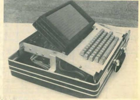
An early prototype of the Microdata model 8400 briefcase computer, now going into production.
