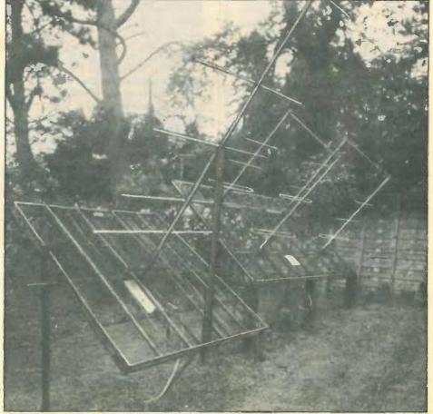
Fig. 2. Four 4-element yagis used to collect radio waves from the sun.
