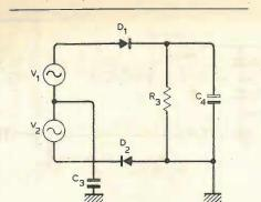
Fig. 12. Equivalent circuit of Fig. 11.
