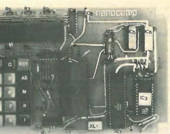
Fig. 4. Assembled printed circuit board and layout details. The board measures 200 x 120mm
