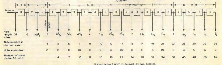
Fig. 6. Shift register can be tapped at necessary increments and simple gating controls appropriate frequencies from generators or pipes. (See part 2, Fig. 7, for simplified control system.)
