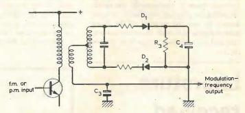
Fig. 11. An unbalanced ratio-detector circuit with a single reservoir capacitor C3.
