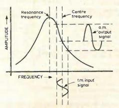
Fig. 2. Simple f.m. slope detector.
