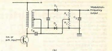
Fig. 8. Two forms of Seeley-Foster circuit using a capacitive link between primary and secondary windings.
