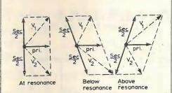
Fig. 6. Vector diagram for the circuit of Fig. 5 showing how the voltages V1 and V<sub>2</sub> applied to the diodes vary with frequency.
