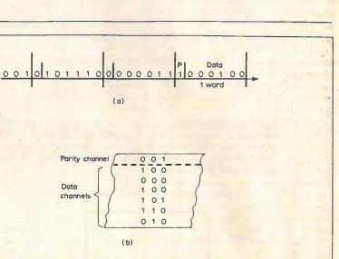
Fig. 1. Parity bits in serial (a) and parallel (b) data channels.
