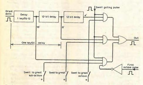
Fig. 4. Coupling between manuals is achieved by lengthening delays so that delayed data occurs at the right place in the scan.
