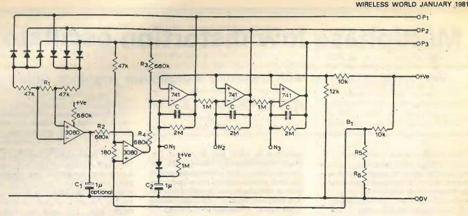
Fig. 4. Three-phase oscillator. f=0.3Hz with C=0.47µF.
