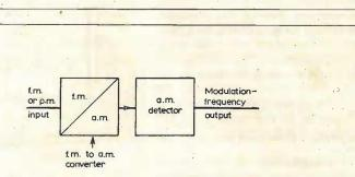
Fig. 1. Block diagram illustrating the form of a number of types of f.m. detector.
