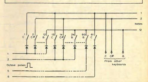
Fig. 2. Identical notes are wired together on one side of matrix, with all 12 notes in each octave wired together via diodes on the other side.
