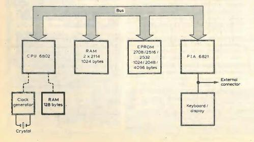
decoding the three most significant address lines. This provides selection of 8 4K address blocks, of which Y1, Y4 and Y7 are used. Note that the most significant address line, A15, from the c.p.u. is not used because sufficient address space is available without it.
