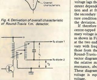
Fig. 5. Method of deriving the two diode inputs in Seeley-Foster and ratio detectors.
