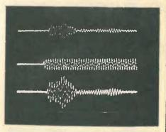
Traces illustrating loudspeaker-room interaction with or without an equaliser. The middle trace is the input tone burst. At the bottom is the room response without an equaliser; at the top the response with an equaliser. Note how the equaliser fails to compensate for envelope distortion and hence timbre and character. (Timebase 20ms/div.)
