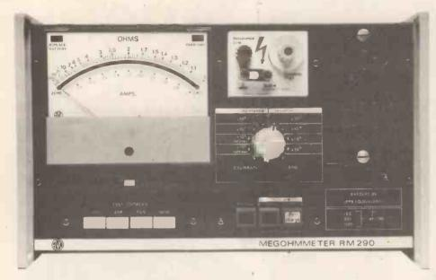
The AVO RM290 is a bench type . megohmmeter with a resistance range that goes up to  $10^{14}~\Omega$  :making it ideal for those applications where there is a need to measure the electrical resistance of non-conducting materials...accurately!
