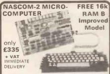
780A 8 bit. This will run at 4 Mhz but is selected between 2/4/Mhz. On-board, addressable memory. 2K 2K Monitor - Nas-sys 1. 1K Video RAM
