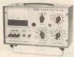
Tests bipolar transistors, diodes and zener diodes. Measures leakage down to 0.5 nA at 2V to 150V. Current gains are checked from 1µA to 100mA. Breakdown voltages up to 100V are measured at 10µA, 100µA and 1mA. Collector toemitter saturation voltage is measured at 1mA, 10mA, 30mA and 100mA for I<sub>C</sub>/I<sub>B</sub> ratios of 10, 20, 30. The instrument is powered by a 9V battery.
