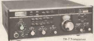
Ham Bands with 1.5-30 MHz receive with built-in 150 MHz frequency counter plus option of 0-1.5 MHz receive and / or any transceiving application 1.8-30 MHz
