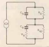
For a long time we have had the original and accurate method of calculation for such an equalization network; here, for example, is one of many possible versions:
