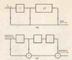
Fig. 2. (a) Encoding a single digit by means of delays T and 2T.
