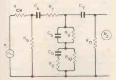
After the usual simplifications we have the equivalent network with a current generator:
