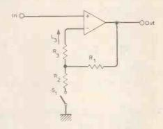
Fig. 3 Basic gain switching circuit.
