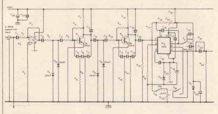
Fig. 3. (top) Clock channel.
