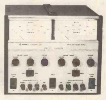
Around 40,000 L series bench power supplies have been sold and the latest units are still uncompromising in performance and reliability. They provide constant voltage or constant current, feature large recessed meters, overload and short-circuit protection, coarse and fine adjustment controls, a separate output switch and LED indicators for mains on and current limit.
