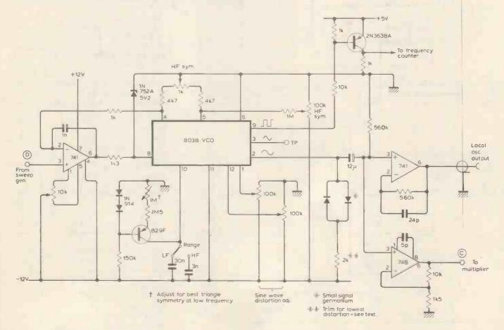
Fig. 11. Local oscillator circuit diagram.
