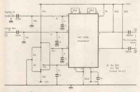
Fig. 9. Multiplier circuit.
