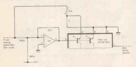
Fig. 17. Modified in this way, the local oscillator of Fig. 11 will provide a logarithmic frequency sweep.
