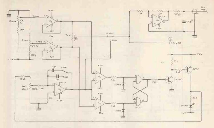
Fig. 12. Sweep control section. Components marked with asterisk are mounted on connector.
