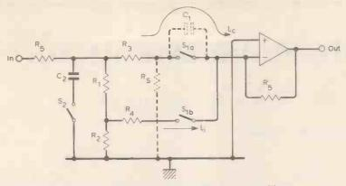
Fig. 7 Internal capacitance effect and compensation low-pass filter.
