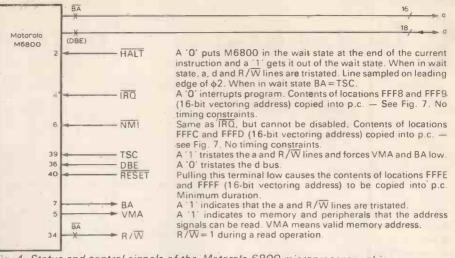
Fig. 4. Status and control signals of the Motorola 6800 microprocessor chip.
