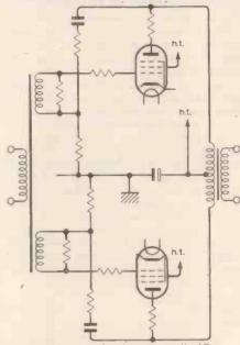
of a well-designed transformer. So there would not in this amplifier be a serious load-sharing problem. The arrangement of the output stage was, as far as I can remember, as shown above: unfortunately my pre-war Wireless Worlds are not to hand. E. F. Good
