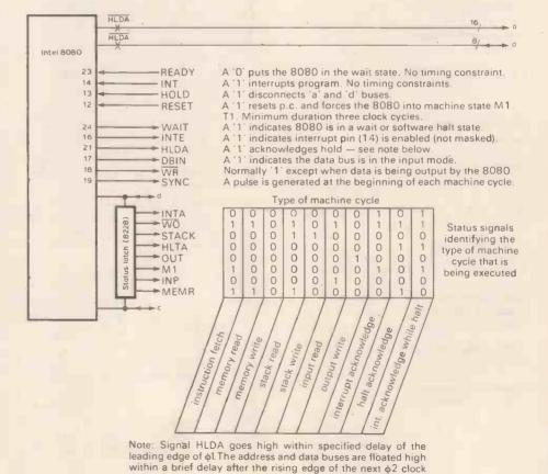
Fig. 3. Status and control signals of the Intel 8080 microprocessor chip.
