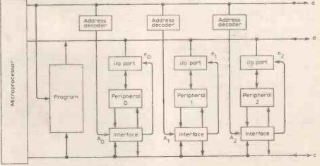
Fig. 6. Basic configuration for single-processor systems.
