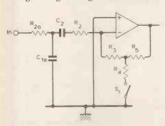
Fig. 10 Inverting input buffer.
