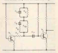
The resistor R<sub>7</sub> is used only for "equalizing" the loading of Tr<sub>1</sub>.
