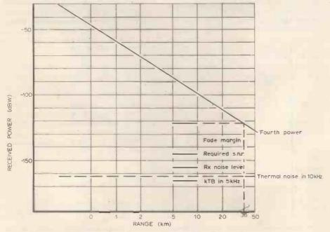
Fig. 3. Estimation of range for s.s.b. system taking into account fading.
