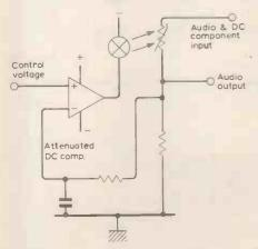
Fig. 2 Closed-loop light dependent resistor attenuator.
