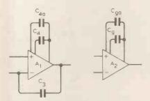
Fig. 11 Alternative compensation networks for other op-amps.
