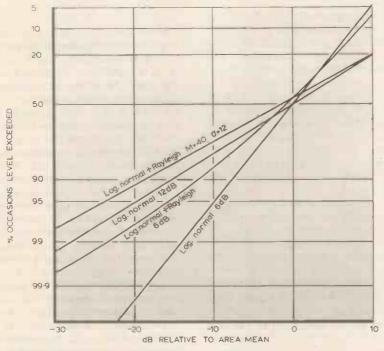
Fig. 2. Fading levels for log-normal shadow fading and long-normal plus Rayleigh fading. Area mean given by fourth power law variation.
