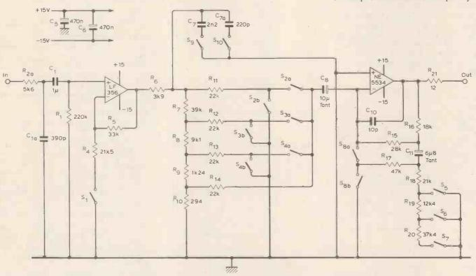
Fig. 8 Complete attenuator circuit for one channel. The switches are grouped in five i.cs as follows;  $S_5 + S_{g'} S_7 + S_{gab'} S_{10} + S_{10} + S_{10} + S_{10}$ . All resistors should be 1%.
