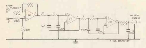
Fig. 10. Low-pass filter. The resistors shown as R are switched, and for bandwidths of 10, 20, 50, 100, 200, 500 Hz should be 72k, 36k, 15k, 7.2k, 3.6k and 1.3k.
