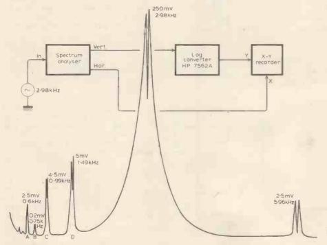
Fig. 6. A typical analysis. The fundamental is at 2.98kHz, its second harmonic being clearly shown at 5.96kHz. The spurious products are all below the frequency of the fundamental.
