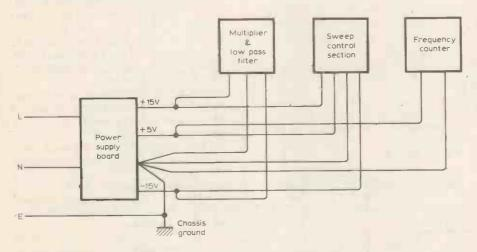
Fig. 16. Wiring should be arranged in this way to avoid common impedances and consequent instability.
