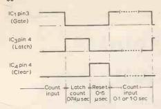
Fig. 14. Timing diagram for counter operation.
