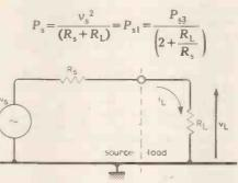
Fig. 1. Simple series circuit with  $\eta = R_{L/}$  $R_1 + R_s$
