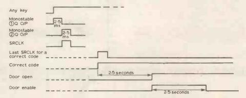
Fig. 3. Timing diagram of logic.
