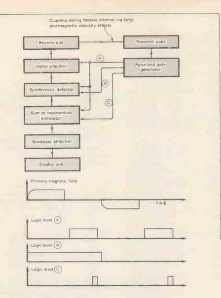
Fig. 6. Circuit block diagram. 🔺
