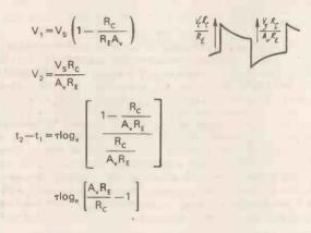
For  $R_{E}$ ,  $R_{C}$  comparable  $A_{V} \gg 1$
