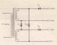
windings alternately and both low current rails are fed on alternate halfcycles. The voltages shown increase when capacitors are connected to provide an adequate margin for the regulators.
