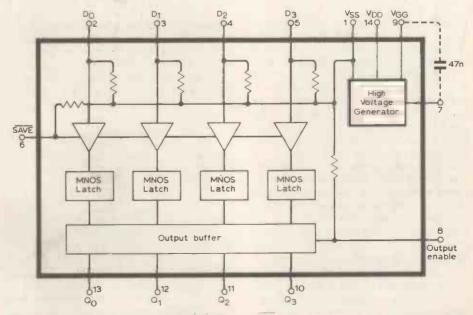
Fig. 1. Internal block diagram of MN9102 quad latch.
