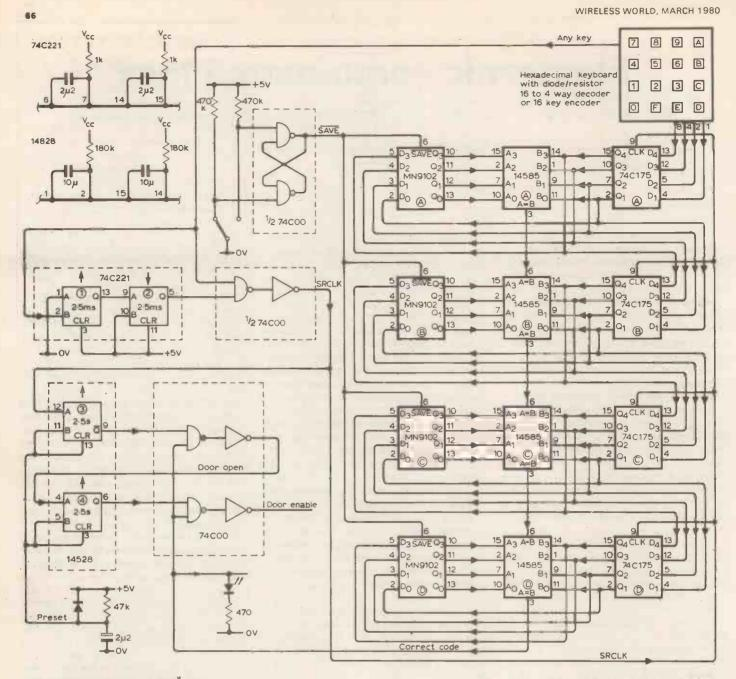
Fig. 2. Circuit diagram of lock logic.
