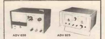
ADV 030 ADV 025 Model No **Output Current** 5 Amp 10 Amn **Output Volts** 2-30 DC 0-25 DC **Input Volts** 115-230-250 A/C 115-230-250 A/C **Tolerated Mains** 15% 15% Variation 05% **Ripple On Load** 05% Load Regulation 5% 5% **Retter Than** Both Models, Internal Fold Back, Overload, Protection Thermal and short circuit Protected. Guarantee Both Models. 2 years Dimensions Height. 130 M/M mm 177 mm Width. 250 M/M mm Depth. 170 M/M mm 335 mm including 294 mm handles
