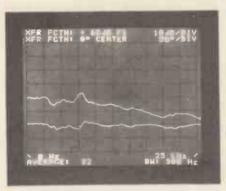
Fig. 4. Comparison of two 1in diameter capacitor microphone capsules in a stereo coincident pair configuration. Lower trace-amplitude. Upper trace-phase.
