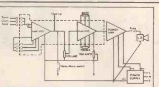
VALUES OF COMPONENTS FOR CONNECTING TO HY5 Volume – 10K n log. Bass/Treble – 100K n linear. Balance – 5K n linear.
