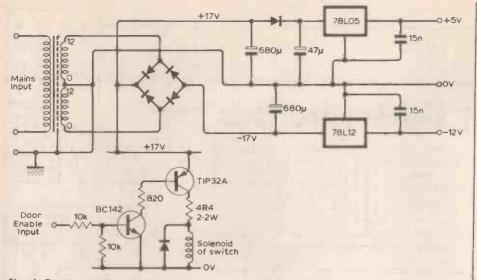
Fig. 4. Power supply and switch driver.
