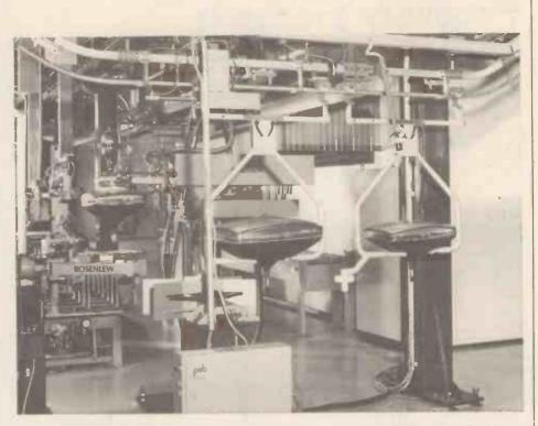
A modern tv tube production line in Finland using 'Japanese'' technology, in this case a Hitachi range of 20in, 22in and 26in tubes of the ''in-line'' variety, featuring quick-start heater, 110° deflection angle, temperature-compensated shadow mask, electrostatic focusing and self-converging integrated neck components. This automated plant, operated by the Automation Group, Valmet Oy, Finland is expected to be producing about 500,000 tubes by the end of 1981.
