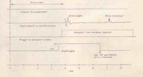
low frequency response is to be examined in detail), an electronic signal gate is needed so that the first directpath signal can be isolated. To do this, and to be able to adjust all the delayscorrectly and generate the test impulse required some auxilliary equipment in addition to the analyser itself. This is unfortunate because it seems that it would have been quite simple to build all the required functions into the analyser in the first instance.\*
