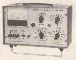
Tests bipolar transistors, diodes and zener diodes. Measures leakage down to 0.5 nA at 2V to 150V. Current gains are checked from 1 $\mu$ A to 100mA. Breakdown voltages up to 100V are measured at 10 $\mu$ A, 100 $\mu$ A and 1mA. Collector to emitter saturation voltage is measured at 1mA, 10mA, 30mA and 100mA for  $I_C/I_B$  ratios of 10, 20, 30. The instrument is powered by a 9V battery.
