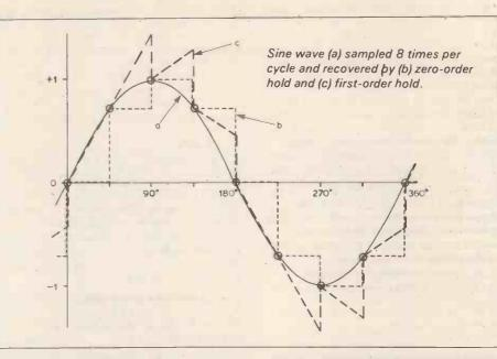
generate a slope which will, one hopes, lead towards the point where the next sample will arrive as shown here. This method effects a significant reduction in the delay terms. A second order hold is also possible and this will generate sections or parabolae. I do not know of any applications in real time where this technique is used, but it is not uncommon for curve generation in the computer numerical control of milling machines, for example.
