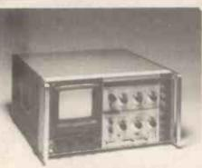
**HEWLETT PACKARD** Spectrum Analyser System 141T Display 8552A IF Section 8554L RF Section 500KHz-1250MHz
