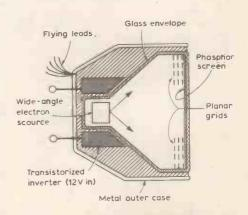
Cross-sectional view of the EEV character display tube. The flying lead grid connections are for multiplexing; the "expected life" of the tube is 40,000 hours or about five years. Clock timer — 2
