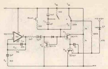
Fig. 11. Noise level monitor uses I.e.d. to indicate when noise level exceeds safe limit as well as simplifying setting-up procedure. Switch is shown in setting-up mode.
