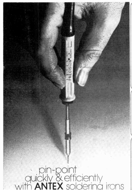
You can now combine fingertip accuracy with strict temperature control (within 2%) at the 0.6mm tip of a miniature soldering iron by using the soldering station shown with one of the 24volt irons.
