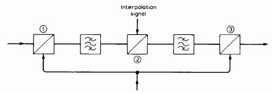
Fig. 17. Triple mixing synthesizer.
