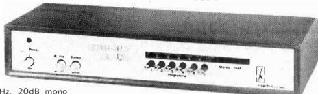
**Brief Spec.** Tuning range 88—104MHz. 20dB mono quieting @ 0.75 µV. Image rejection — 70dB. IF rejection — 85dB. THD typically 0.4%.
