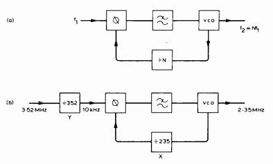
**Fig. 18.** Phase-locked loop multiplier (a) and a p.l.l. multiplier solution to the 2.35/3.52 problem (b).
