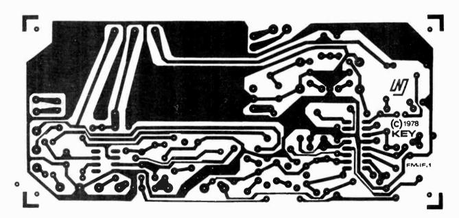
Printed circuit board layout for the i.f. circuit
