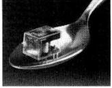
or 1A 24V d.c. Coil ratings range from 1.5 to 24V at currents between 18.8mA and 300mA, while service life is said to be in excess of  $5\times10^6$  operations. Coil resistances range from 5 to 1280 $\Omega$ , and the maximum switching frequency is 1800 operations per hour. Operate and release times are both around 5ms and the insulation resistance is greater than 100M $\Omega$ . IMO Precision Controls Ltd, 349 Edgware Road, London W2 IBS WW 317
