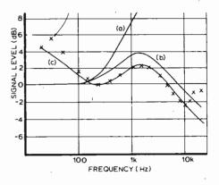
Fig. 2. Effect of noise pumping is reduced by using pre-emphasis (curve a) prior to compression and corresponding de-emphasis on expansion to reduce h.f. noise by 12dB. Possibility of tape saturation is alleviated by adding pre-emphasis in the detector path, as in the dbx system, giving combined result of curve b. Low frequency pre-emphasis, included in curve c helps to reduce audibility of hum signals.
