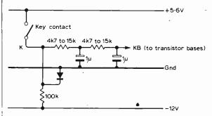
Fig. 14. Keying circuit. The double integrating network is used to control a d.c. output component by shaping the keying envelope.
