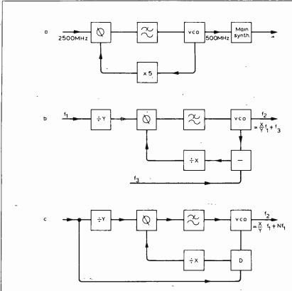
**Fig. 19.** P.l.ls can be used as high-speed dividers by inclusion of a multiplier in the loop. P.l.l. at (a) divides by 5. Mixer at (b) reduces frequency requirements of divider and (c) shows alternative method.
