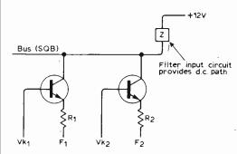
**Fig. 13.** Common-base transistor gates. Input signals  $F_1$  and  $F_2$  are square-wave divider outputs.
