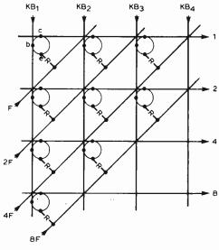
**Fig. 15.** Portion of the three-way matrix. This layout is roughly the same as the p.c.b. viewed from below.
