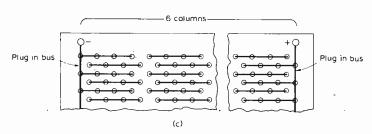
Fig. 1. Breadboard socket systems.
