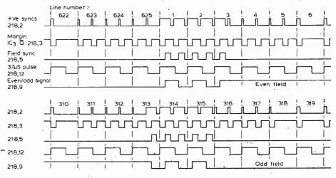
**Fig. 2.** Waveforms in the odd/even field  $\blacktriangleright$  selector, IC<sub>218</sub>
