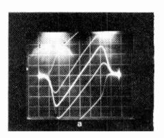
Effect of tuning  $L_2$  (a) and  $L_3$  (b) in double-tuned discriminator circuit, compared with characteristic of single-tuned discriminator (c). Ordinate 0.5V/cm, abscissa 100kHz/cm.
