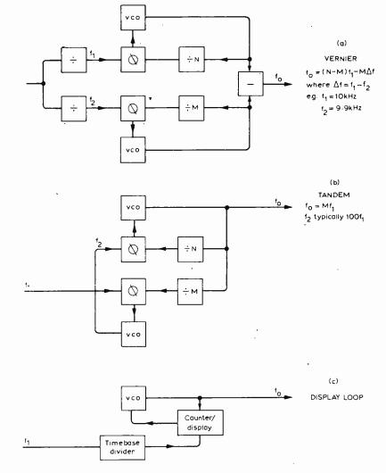
Fig. 20. Methods of achieving wide bandwidth and small increments.
