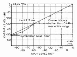
Compressor law with ideal curve and measured values. Measurements made at LM381 input and NE570 output at lkHz.
