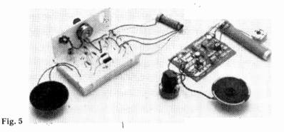
strips of 25 linked sockets, provide eight power supply rails. The double-sided strips of sockets are available in nickel silver or with a gold plated finish. The blocks are supplied with a self adhesive backing compound for instant and semi permanent mounting. This backing can be peeled off to expose the socket strips which can then be removed. However, this is a sticky procedure and
