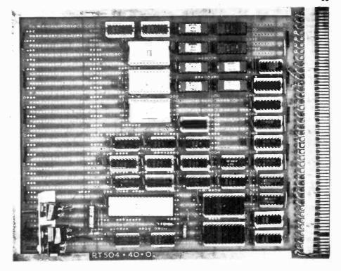
**Fig. 3.** Add-on Telesoftware board to go with the teletext decoder in Fig. 2.
