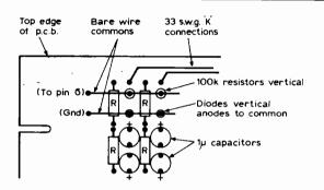
Fig. 17. Keying circuit layout from component side, showing two circuits. Except for the value of R, all of the circuits are identical. The common wire connections bend down to enter the p.c.b. on the left.
