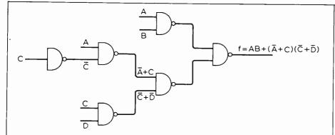
Fig. 11. Minimal circuit for  $f = A B (\overline{A} + C)(\overline{C} + \overline{D})$ , using the merging operation.
