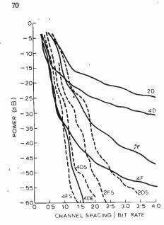
Fig. 2. Adjacent channel rejection ' factor.
