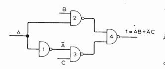
Fig. 7. Mechanism of "spike" generation.
