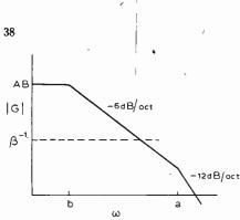
Fig.3. Gain vs frequency plot for the amplifier in Fig.2; both axes logarithmic.
