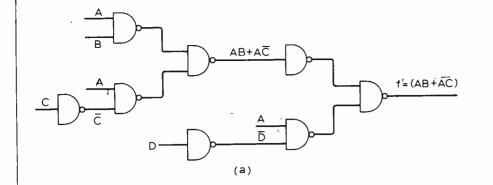
Fig. 9. Bracketing two products in  $f = A B + A \overline{C} + A \overline{D}$  enables use of 2-input gates but requires eight instead of six, as in (a). Removing a common factor again meets fan-in restriction to 2 inputs, with varying savings in number of gates, as seen in (b) and (c).
