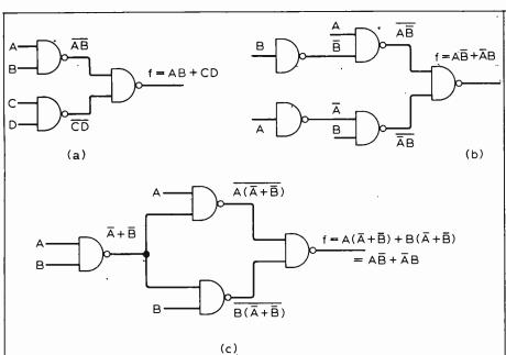
Fig. 3. The use of NAND gates to obtain a sum-of-products function (a). The minimal form of expression need not give a minimal circuit; minimal expression  $f = \overline{A} \overline{B} + \overline{A} B$  in (b) needs one more gate than non-minimal expression  $f = A (\overline{A} + \overline{B}) + B (\overline{A} + \overline{B})$  at (c).
