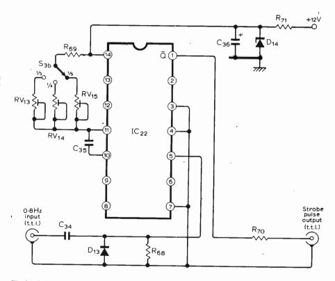
Fig 14. SR strobe-pulse generator
