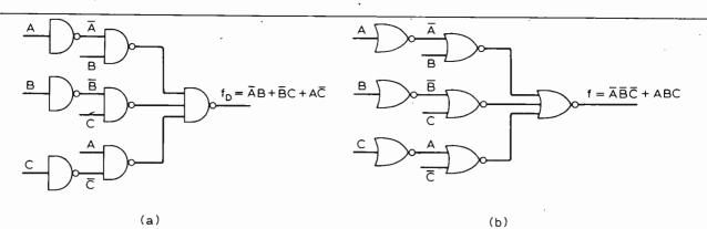
Fig. 6. Generating a function using NOR gates. Function  $f = \overline{A} \ \overline{B} \ \overline{C} + A B$  C is first dualized, minimized and implemented in NAND logic, as at (a). This circuit is then converted to NOR gates to provide the required output.
