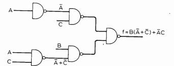
Fig. 12. Two-input NANDS used to realise  $f = B(\overline{A} + \overline{C}) + \overline{A}C$ , which is hazard-free form of  $= \overline{A}C + B\overline{C}$ .
