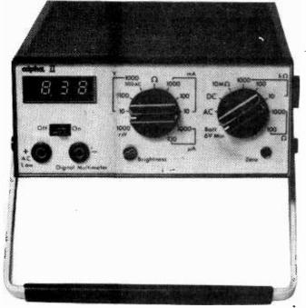
Use the instrument for a little while, and something else will impress you: its accuracy. The Alpha II is accurate to within 0.2% – better than many a more expensive instrument.
