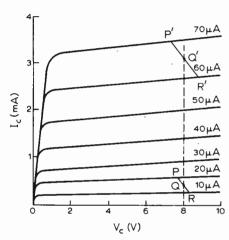
$\dot{F}i\bar{g}$ . 18.  $I_c - V_c$  characteristics and load lines showing the action of reverse a.g.c.
