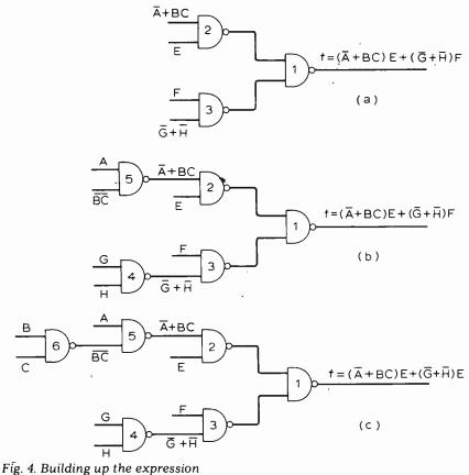
Fig. 4. Building up the expression  $f = \overline{A} + BCE + (\overline{G} + \overline{H})F$  from the output end in three levels.
