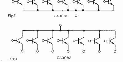
segments to display any number from 0 to 9, the display devices may be filament or l.e.d., and the currents required might be up to 100mA per segment. In addition, the preceding drive circuitry may require common emitter or common-collector configurations. These options are indicated in Figs. 3 and 4 and it is interesting that the transistors can be accommodated in a 16-pin standard package leaving just one spare pin as a separate substrate connection.
