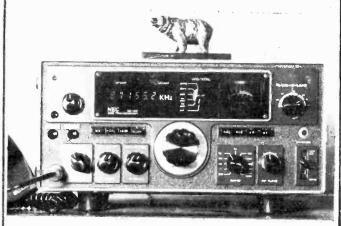
allband, HF, 300 wattstransceiver, 160 / 80 / 40 / 20 / 15 / 11 / 10A / 10B / 10C / 10D / WWV, modes FSK, USB, LSB, CW, AM, with separate 8 pole X-tal lattice filters for each mode fitted. Further features: Side tone at CW, VOX (automatic transmit-receive) by talking into microphone), 11 meter CB band, all channels easily selectable through digital counter, excellent receiver sensitivity at extreme crossmodulation security by application for the 7360 low noise beam, deflection mixer tube.
