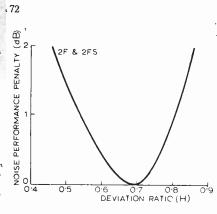
Fig. 8. Effect of f.s.k. deviation ratio on noise performance.
