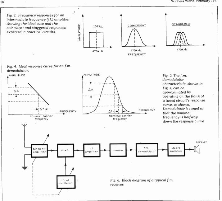
circuits all of which had to track together over the radio spectrum. This combination of amplifiers had a combined frequency response curve which was very sharp and centred on the carrier frequency of the received signal. In the superhet the i.f. amplifiers are all tuned close to a fixed frequency which does not change when the radio is tuned to different transmitters.
