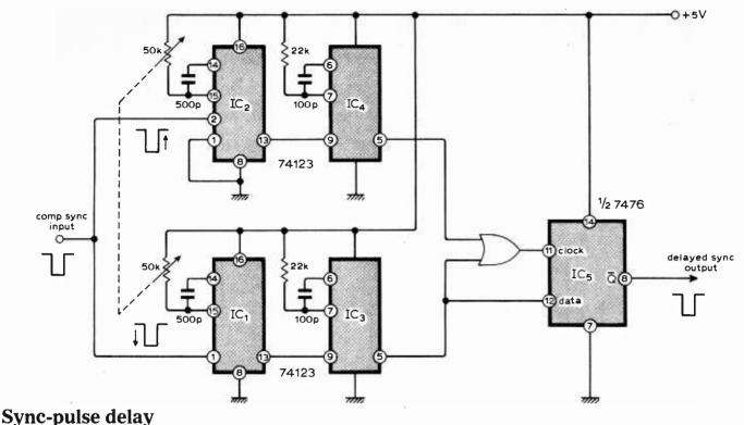
In t.v. broadcasting it is sometimes necessary to delay a composite signal. Passive elements can be used but these only offer delays of a few hundred ns. If a longer delay is required, several of these elements are used. This circuit replaces these passive networks and allows a variable delay up to  $7.0\mu$ s.
