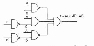
Fig. 8. "Direct" generation of  $f = A B + A \overline{C} + A \overline{D}$  when 3-input gates can be unused.
