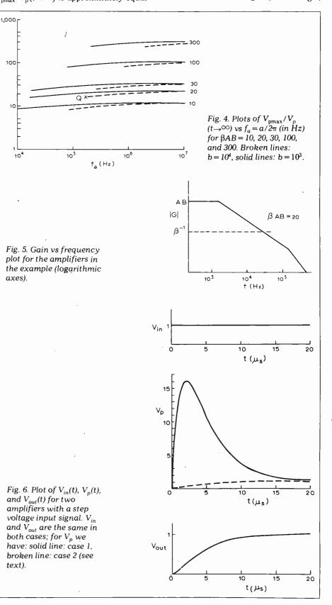
ref.1, for  $\gamma = 0$ ). Thus for  $a \gg b$  we always get, for a step input, a maximum voltage  $V_p$  that is approximately  $(1 + \beta AB)$  times the steady state voltage at infinite time.
