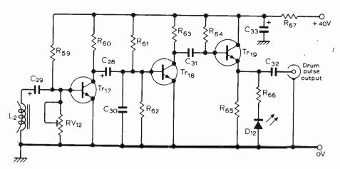
Fig 13. Drum-pulse amplifier
