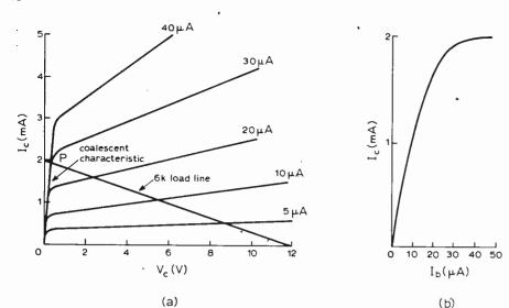
Fig. 17. (a) Load line exhibiting limiting characteristic and (b) the input-output characteristic for the  $6k\Omega$  load line of Fig. 17 (a)
