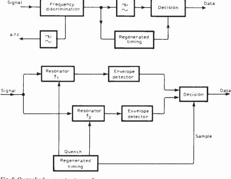
Fig. 8. Quenched-resonator type of f.s.k. demodulator.
