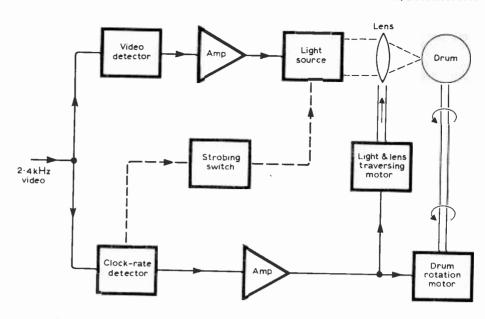
Fig. 2. Basic block diagram of machine.
