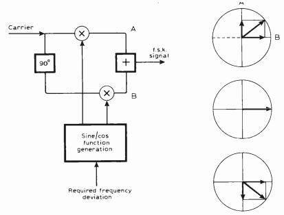
Fig. 4. General form of the modulator shown in Fig. 3.
