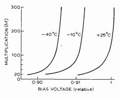
Fig. 7. Avalanche photodiode characteristic allows manual or automatic gain control by bias variation.
