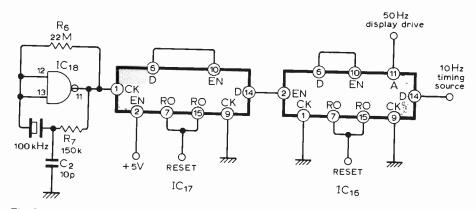
Fig. 2. Crystal oscillator and dividers. A standard Pierce circuit is used with the crystal,  $C_2$ , and input capacitance of the gate acting as the feedback network.
