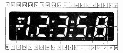
Fig. 6. Liquid crystal display connections.
