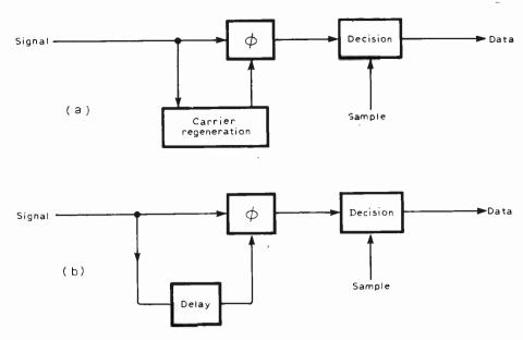
Fig. 9. Coherent (a) and differential (b) binary phase demodulators.
