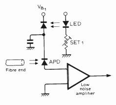
Fig. 9. Novel method of providing current source for biasing uses second photodiode, illuminated with adjustable light source.
