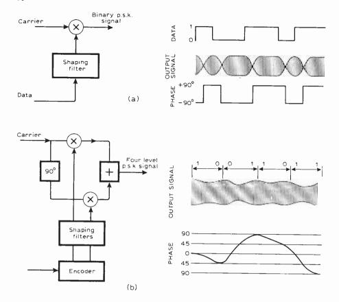
Fig. 6. Binary p.e.k. modulator ▲ producing band-limited output signals is shown at (a) while (b) shows a four-level p.e.k. modulator.
