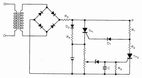
Fig. 7. Automatic charger control. Circuit can be simply set up by using a large capacitor and suitable resistor in place of battery.
