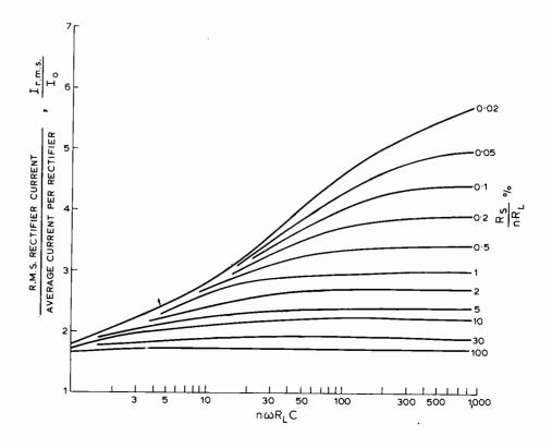
Fig. 4. The ratio repetitive peak current/average current per rectifier, plotted against  $n\omega R_L C$ . C in farads and  $R_L$  in ohms,  $\omega=2\pi f$  and f is line frequency. n=1 for half-wave, n=2 for full-wave and n=0.5 for voltage-doubler.
