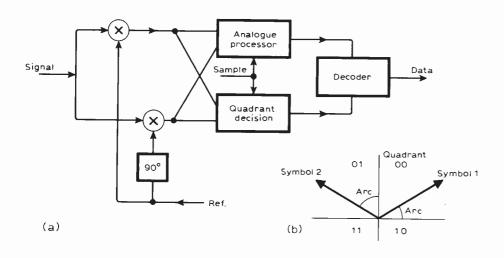
Fig. 11. A further type of demodulator not using a delay line.
