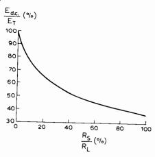
Fig. 2. Characteristics of full-wave rectifier for  $\omega$ CR large, as is the case in battery charging.
