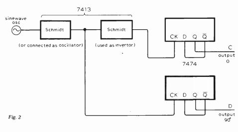
divided by two using the 7474 flip-flop. Output waveforms from the flip-flops are at half the input frequency and in quadrature. This system has only one time sensitive component which makes tuning over a large range possible. High
