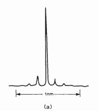
pulses exhibit spectral widths of 3nm or so, whereas biasing above threshold ensures spectral widths of only  $0.5 \text{nm}^{28}$ ; and thus minimizes material dispersion see Fig. 4.
