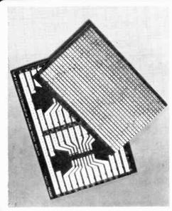
Circuit diagram to circuit board in minutes. Layout circuit plan on .1" graph paper. Select Blob Board, lay components out with leads on copper strip. Blob of solder onto lead and your circuit is complete. Blob Boards normally half price of competitive boards. Roller tinned to solder components directly. No drilling or mounting. Modifications in seconds. Blob Board is re-usable.
