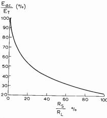
Fig. 6. Characteristics of half-wave rectifier for  $\omega CR$  large.
