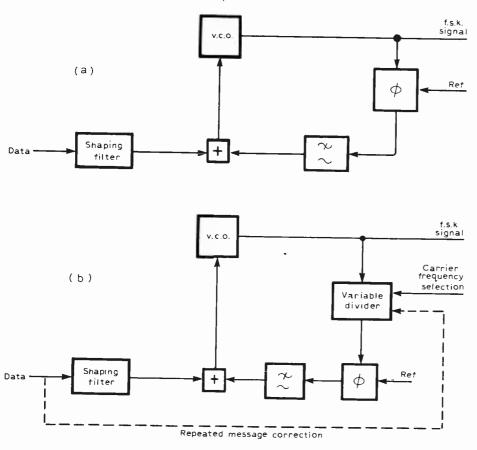
Fig. 2. The v.c.o. of Fig. 1 can be included in a phase-lock loop as in (a) to increase the accuracy of control. In the variation at (b) the variable divider enables the phase comparison to take place at the low reference frequency.
