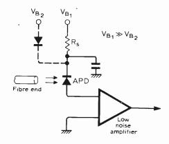
Fig. 8. Gain control of a.p.d. using high source resistance gives flat a.g.c. response.
