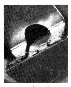
Fig. 10. Hermetic sealing of laser diodes prevents degradation due to contamination. Both stud type (a), above, and planar type (b), right, can also be used for l.e.ds.
