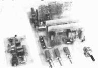
Master Board with one Replay Amp removed
