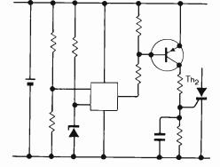
Fig. 8. Use of precision control section is only meaningful if ripple voltage is less than required setting accuracy.
