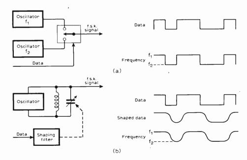
shaping which enables the constantamplitude feature of the modulated signal to be retained. The disadvantage of this method is, however, that strict band limiting of the modulated signal cannot be achieved and finite energy is spread over an infinite frequency band. Some of this energy will therefore fall
