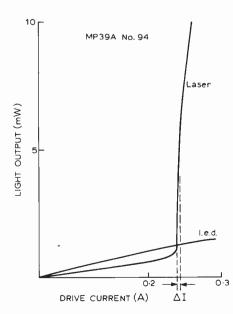
Fig. 3. CW laser output versus drive characteristic shows almost linear relation for an l.e.d. and abrupt threshold for laser.
