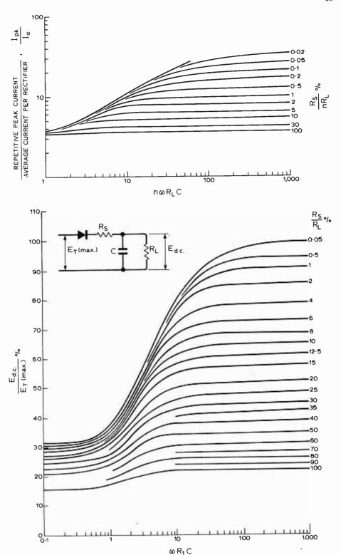
Fig. 5.  $E_{dc}/E_{T(max)}\%$  as a function of  $\omega R_L C$  for half-wave circuits. C in farads, and  $R_L$  in ohms,  $\omega = 2\pi f$ .
