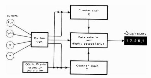
Fig. 1. Block diagram of the stopwatch. Total power consumption for this circuit is between 200 and  $300\mu A.\,$
