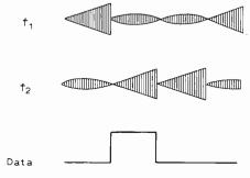
slowly and take about one digit period to change from 0 to 1 or vice-versa. As a result of this, the output amplitude of the balanced modulator will vary as shown. It can be seen that in this case bandlimiting the signal results in abrupt phase transitions occurring when the signal amplitude is zero.
