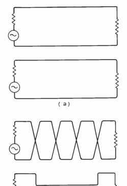
linking the receiving loop. This can be done by careful layout particularly of printed circuit boards, by avoiding ground returns and by twisting together go and return conductors<sup>15</sup> see Fig. 8(b).
