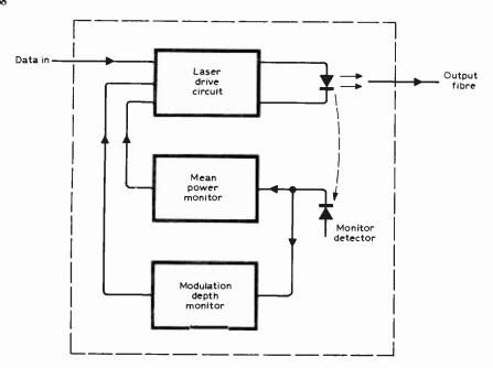
Fig. 5. Feedback from laser output ensures correct laser bias despite variations in threshold due to temperature effects and ageing.
