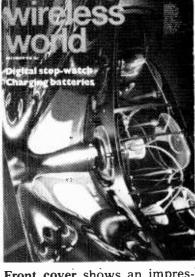
Front cover shows an impression of the CV3 Superscreen colour television projector marketed by Speywood Communications. The three separate Schmidt optical systems are mounted in line and use 75mm tubes.
