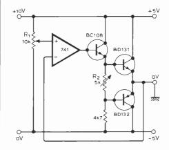
When working with i.cs it is often necessary to have positive and negative supplies, and it is desirable that each supply remains steady with changes in load current. This circuit has been a useful addition to an adjustable 0 to 15V stabilized supply. For +5 and -5V, potentiometer  $R_1$  is set to the mid position and the current through the output transistors is set to 20mA by  $R_2$ .
