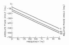
Fig. 1. Absolute phase-frequency response curve of all-pass networks used for phase shift experiments.
