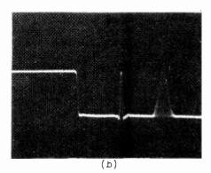
Fig. 24. Distorted 2T and 10T pulses mainly corrected by tuner group-delay equalizer but comparing remaining distortion caused by different transmitter characteristics.
