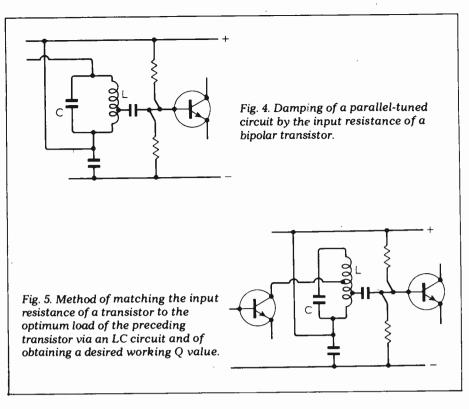
tapping point must be such that the turns ratio between the winding presented to the collector circuit and that presented to the base circuit of the following transistor is n:1 where
