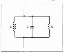
Fig. 3. A parallel-tuned circuit damped by a parallel resistor R.
