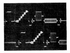
Fig. 22. Insertion test signal (i.t.s.) waveforms as generated (top), and as received showing added distortion (bottom).
