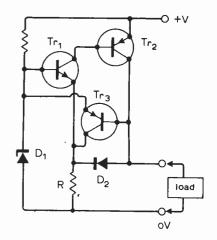
normally-closed push button switch in the collector of  $Tr_3$  may be used, with the advantage that fold-back limiting. remains in action through the  $Tr_3$  base-emitter diode during the switch on process.
