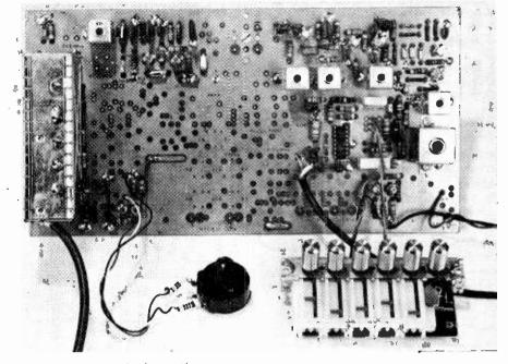
Sound-only tuner with alternative push-button tuning control.
