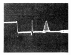
Fig. 23. Detail of 2T and 10T i.t.s. pulses showing effect of gain and delay inequality distortion.
