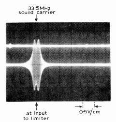
Fig. 20. Sweep response of Tr<sub>9</sub> output showing sound i.f. band.
