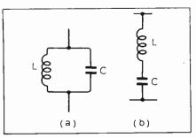
Fig. 1. For given values of L and C<sup>1</sup> parallel-connected circuits (a) and series-connected circuits (b) have the same resonance freqency. the square root of inductance and to the square root of capacitance: thus the required value of  $f_o$  is given by
