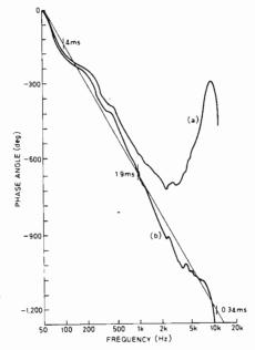
Fig. 3 (a) Phase-frequency response curve of monitoring loudspeaker type LS5/5 (b) Phase response plus 4ms time delay.
