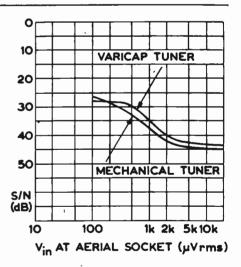
Fig. 26. Curves show satisfactory noise performance (on a "just perceptible" basis at 38dB) is obtained for inputs as low as  $700\mu V$  at the aerial socket. Sound signal-to-noise ratio is better than 50dB over the whole range.
