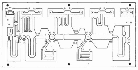
x = 0.8mm holes for components = 3 5mm holes for p.c b, mounting
