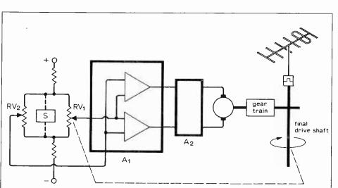
Fig. 1. Block schematic diagram of the proportional control system.
