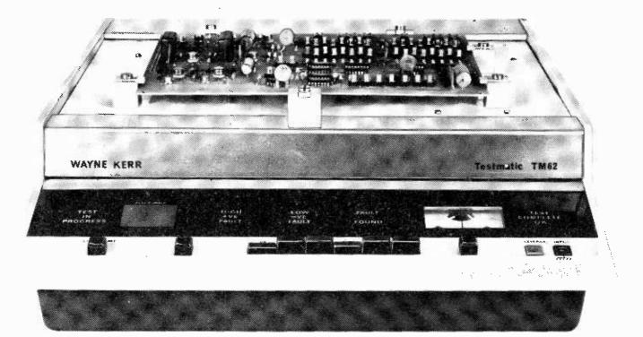
Testmatic TM62, designed as a selfcontained on-line test station, is a new addition to the Wayne Kerr range of lowcost automatic test equipment. Plug-in test panels can be changed-over in 5 seconds to suit different production lines. Operation is simple: assembly staff can check circuit boards as soon as éach one is completed.
