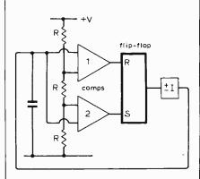
Fig. 12. Triangular wave generator using technique of Fig. 11. Comparator reference inputs are set to 2V/3 and V/3, the capacitor voltage ranging between these limits.
