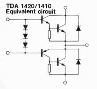
The TDA 1420 integrates a quasi-complementary (NPN/PNP) darlington pair and biasing diodes for perfect electrothermal matching. Applications for this versatile power IC include DC or stepping motor drivers, op amp power boosters, audio output stages, etc. All this in Pentawatt<sup>®</sup>, the rugged 5-pin plastic pack. For lower voltages try the TDA 1410.
