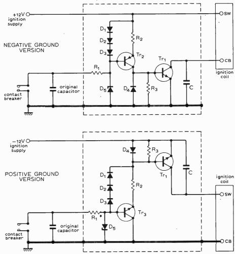
Complete circuit diagrams for positive- and negative-ground systems.
