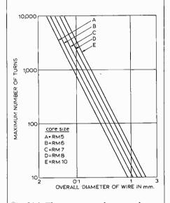
Fig. 5(a). These curves apply to round cores conforming to B.S.4061 range 2 or I.E.C. Pub.133.
