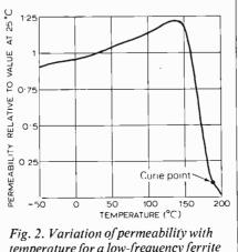
temperature for a low-frequency ferrite material.
