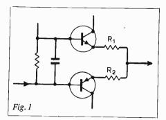
the quiescent current is dependent on the temperature; and (c) too much quiescent current results in a kind of "take over distortion". This kind of distortion is due to a signal current flowing through the resistors  $R_1$  or  $R_2$  (Fig. 1), cutting off the quiescent current of the other stage, which results in a voltage shift at the input necessary to keep the output following the signal.
