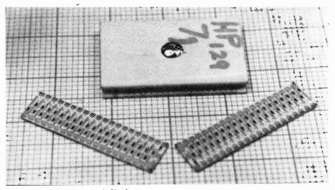
Fig. 4. Two of the new thick-film logic circuits compared in size with the hermetically sealed logic package (above) used in the second implant.
