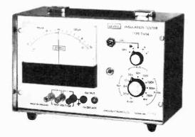
A logarithmic scale covering 6 decades is used to display either insulation resistance or leakage current at a fixed stabilised test voltage. The current available is limited to a maximum value of 3mA for safety and capacitors are automatically discharged when the instrument is switched off or to the CAL condition. The instrument operates from a 9V internal battery.
