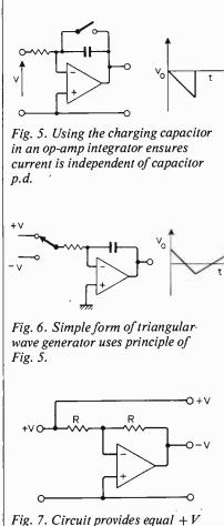
Fig. 7. Circuit provides equal +Vand -V inputs for Fig. 6 with an op-amp of -1 gain.
