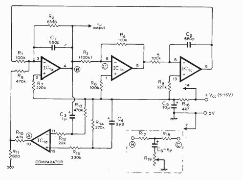
is fed back into the loop to sustain oscillation. Sinewave amplitude is stabilized by virtue of the constant square wave input and is typically  $0.25V_{cc}$  pk-pk, its purity being proportional to filter Q.
