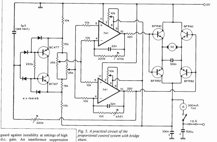
d.c. gain. An interference suppression capacitor is also connected across the motor terminals. Inclusion of offset null controls (the  $10k\Omega$  potentiometers) is recommended. Adjustments are carried out with the wiper arms of the bridge potentiometers brought to the centre of their tracks and then short circuited together. The offset null potentiometers are then set to give an output of exactly half h.t. potential at each operational amplifier.
