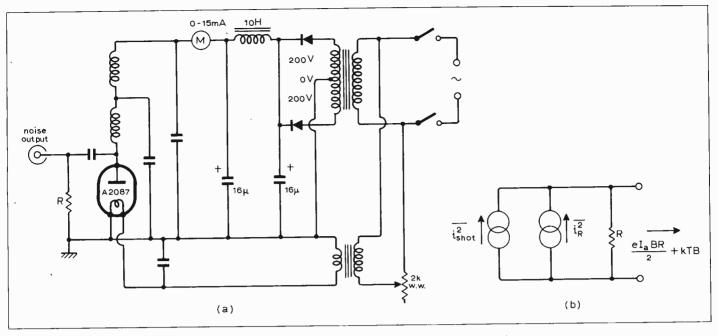
Fig. 8. Still an extremely useful noise source for measurement purposes, the saturated thermionic diode is an absolute noise generator. (a) shows a typical circuit using an A2087, (b) is the equivalentcircuit for calculation purposes.
