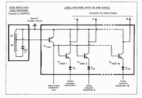
$25 \text{mm} \times 6 \text{mm}$  ceramic substrate and the thick film parts of the circuit are successive layers of resistor material, palladium silver conducting pads and cross-overs, glass for insulation, and gold for transistor connecting pads and the two bus-bars shown in Fig. 3. The transistors and diodes attached to this thick film circuit are beam lead devices, and have a silicon nitride impermeable skin put over them.
