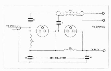
The above power separating filter is only one example of the sort of work that our engineers do in the design and development laboratories of the Submarine Systems Division of S.T.C.
