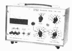
Tests bipolar transistors, diodes and zener diodes. Measures leakage down to 0.5 nA at 2V to 150V. Current gains are checked from 1µA to 100mA. Breakdown voltages up to 100V are measured at 10µA, 100µA and 1mA. Collector to emitter saturation voltage is measured at 1mA, 10mA, 30mA and 100mA for  $I_C/I_B$  ratios of 10, 20, 30. The instrument is powered by a 9V battery.
