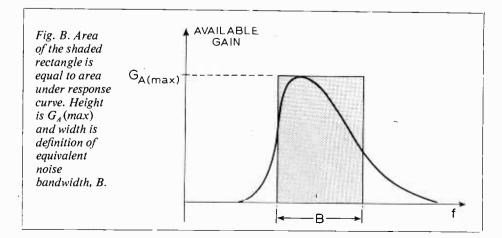
$$G_{A} = \frac{K'R_{in}^{2}R_{g}n^{2}}{(n^{2}R_{g} + R_{in})^{2} + \left(\omega L - \frac{l}{\omega C}\right)^{2}}$$
