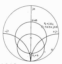
Basically we rely on the fact that a circle centred on the Smith Chart real axis can be transformed by a change of normalizing impedance to a circle anywhere on the chart axis. So to match 5+j5 to 50 ohms, as in the example, a possible procedure is as follows.
