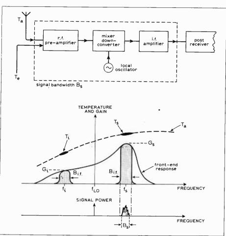
final parameter in any data link or communications system. The effect of the noise power is as though all of it is concentrated into the signal bandwidth  $B_s$ . Therefore we define another temperature; the operating noise temperature,  $T_{op}$  as  $P_{NO}/kB_sG_s$ .
