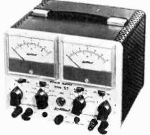
Set by switches and fine control. Meters switchable for volts, 0 to 100mA and 0 to 1A. entrant protection. Pilot
