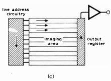
Fig. 8. Design choices—(a) frame transfer, (b) interline transfer, (c) line transfer (ref. 7).
