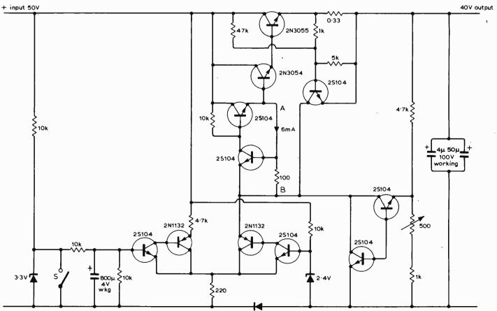
Fig. 5. Complete regulated power pack with current switching control.
