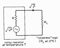
Fig. 2.  $R_L$  is absorbing power from R. Maximum power is absorbed when  $R = R_L$ , according to the well-known matching theorem.
