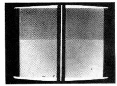
Fig. 10. Same signal as in Fig. 9, but applied to a receiver with a faster flywheel circuit.
