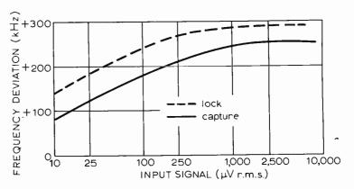
Fig. 4. Variation of the capture and lock ranges with the signal input level.
