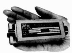
SE40 DC/DC variable reluctance transducer. High level output ± 5V d.c. Pressure range 5 to 5000 p.s.i. gauge, differential or absolute. Temperature range -45 to + 150°C. Total error band less than 1.5%.
