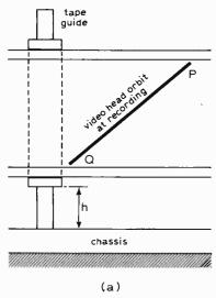
Fig. 5. Effects of tape guiding errors.
