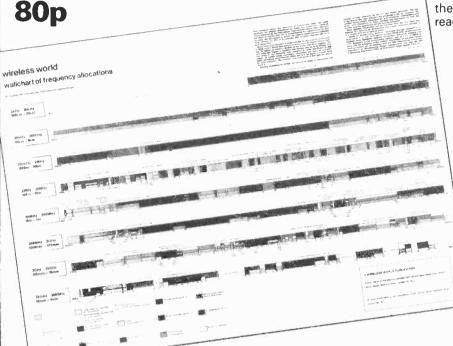
The wallchart shows the allocation of frequencies within the radio spectrum ranging from 3 kHz to 300 GHz and is scaled on eight logarithmic bands contriving 15 main categories of transmissions which are identified by colours. All the important spot frequencies and 'special interest' frequencies are marked. The information is taken from the ITU and has been condensed into easily read chart form. Measures 2' 11"  $\times$  1' 11"
