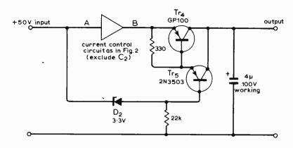
Fig. 3. Practical tandem current control circuit for several parallel loads.
