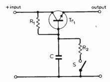
Fig. 1. Basic voltage control circuit.
