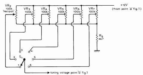
Fig. 2. The preset and continuous tuning unit.
