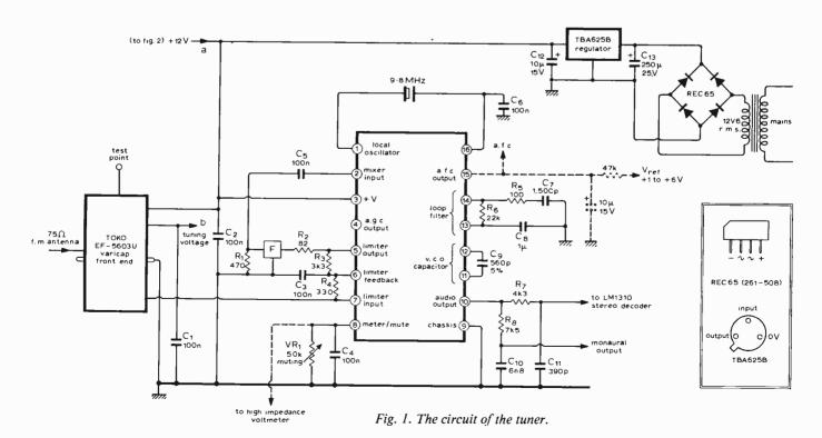
The output filter  $R_7$ — $C_{II}$  attenuates radio frequencies, whilst  $R_8$ — $C_{I0}$  provides the normal 50µs de-emphasis for the monaural output. The effective resistance between pin 10 and ground should not be less than 2k $\Omega$ . A series capacitor (not shown in Fig. 1) will be required in each output circuit to prevent the steady component of the voltage at pin 10 from reaching the following audio amplifier or decoder.
