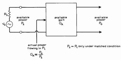
Fig. 3. Available power gain has no direct connection with matching, but maximum available power gain is only obtained when  $R_s$  matches the input resistance of the amplifier.
