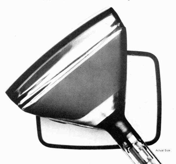
The new Brimar M14-100 is the smallest U.K. – made magnetic focus tube available with special phosphors. Although its maximum overall length is, in fact, only 184 mm., it has a minimum useful screen area of 110 mm. x 83 mm. Particularly suitable for data display and monitoring devices where a bright image with crisp display is required. (A typical linewidth is 0.23 mm. at a beam current of 30 µA.)
