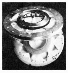
New flexible loudspeaker diaphragm material (see news item). Damping material is attached at the circumference and centre to prevent wave reflections within the material. Also attached to the diaphragm is the voice coil assembly. The chassis is shown at the top of the picture separately from the diaphragm.
