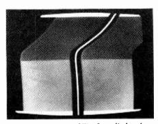
Fig. 9. Test pattern of Fig. 8 applied to the same receiver. In this case the video signal is affected by  $a + 16 \mu s$  phase jump.
