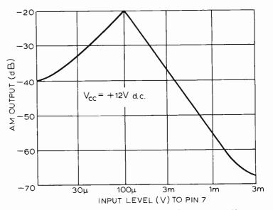
Fig. 3. A.m. rejection plotted against the signal input level to the NE563.
