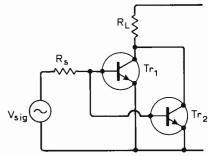
Fig. 1. Two transistors in parallel.
