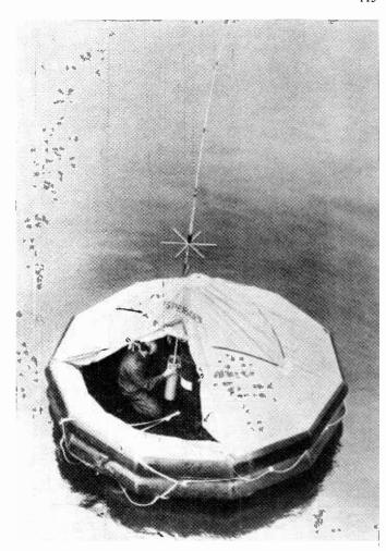
Specialized aerial which radiates both 243MHz and 2.182MHz simultaneously is part of Ultra's new distress beacon which provides transmission on both the marine and aircraft distress frequencies.
