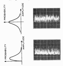
Fig. 1. White noise has a Gaussian distribution (upper oscillogram). After band limiting, white noise typically shows a Rayleigh distribution (lower oscillogram).
