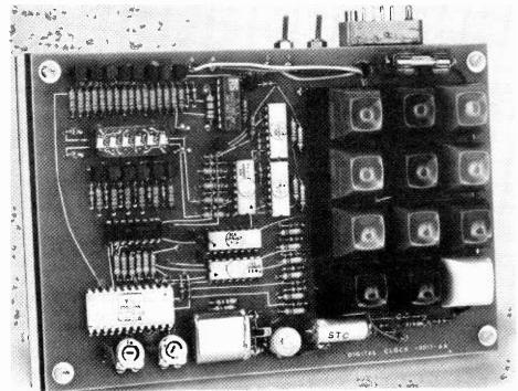
Fig. 10. The complete unit, assembled in a "tray" with the alarm speaker and batteries underneath the board.
