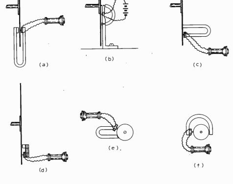
Fig. 1. The magnetic replay system patented by Edison's assistant, Sumner Tainter.
