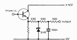
Fig. 3. Circuit used to protect output of tone generator from damage arising from uniselector voltages.
