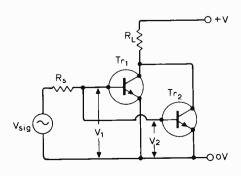
$Tr_1$  and  $Tr_2$  are identical transistors with the same input resistance, current gain and noise generators.
