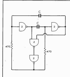
Fig. 1. Oscillator circuit assembled from t.t.l. NAND gates. For capacitor values for the three frequencies
