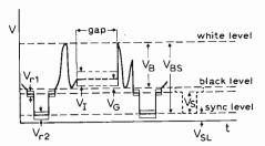
Fig. 7. Signal parameters used for defining errors of the video signal.
