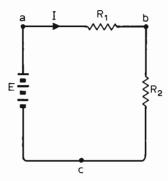
Fig. 1 Simple d.c. circuit for illustrating Kirchhoff's voltage law.
