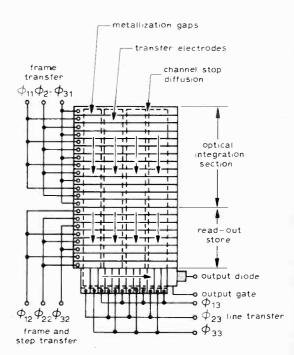
of the array is called the optical integration section; the area of the device upon which the image of the scene falls.
