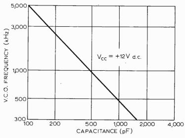
Fig. 5. Free running frequency of the v.c.o. plotted against the capacitance connected between pins 11 and 12.
