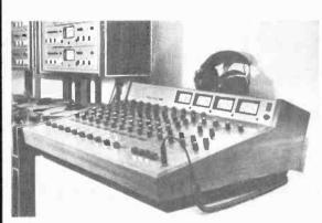
Ten inputs. Four output groups. Four limiters. Base, mid, treble EQ. Balanced inputs. Modular construction. Heacphone monitoring.
