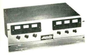
The Mavis 3 way electronic cross-over is intended for use primarily with music and speech amplifying systems. It enables the bass range, mid-range and treble range to be separately controlled. The cross-over frequency for each range can be specified if required but will be, in the standard unit, as follows: Bass roll-off 45 c.p.s.
