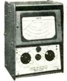
TF 1400S DOUBLE PULSE GENERATOR WITH TM 6600/S SECONDARY PULSE UNIT. For testing radar, nucleonics, 'scopes, counters, filters elc. SPEC. TF 1400S. Rec. frequ. 10Hz to 100 kHz, pulse width 0'1 to 100µ sec., delsy -15 to +3000µ sec., fras time < 30N sec. SPEC. TM 6600/S. As for TF1400S except pulse width 0'5 to 25µ sec, delay 0 to + 300µ sec. £230.
