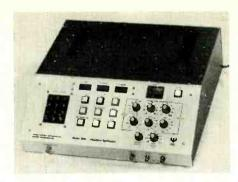
Prosser Scientific Instruments digital waveform synthesizer with keyboard data input.
