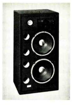
pression driver loaded by an exponential horn with an acoustic lens to give a dispersion pattern  $40^{\circ}$  by  $110^{\circ}$ . All frequencies above the 7000Hz point are fed to a horn loaded ring radiator with a -5dBpoint at 21kHz. Crossover is effected by a 12dB/octave constant impedance passive circuit. The enclosures themselves are a 9 cubic ft distributed port reflex which, it is claimed, gives an improved linearity at low frequencies.
