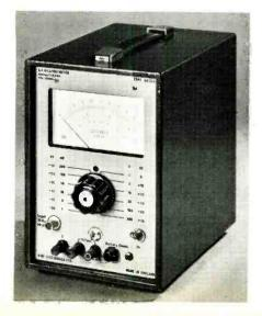
earth link is removed. Under these conditions the amplifier output will also be floating. The use of batteries as a power source greatly reduces the problems of "hum" and earth loop currents which may invalidate readings when very small voltages are being measured. A battery check facility is incorporated. For routine laboratory/bench use a regulated mains power unit is available as an optional extra.
