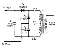
Fig. 7. Alternative high voltage supply circuit.
