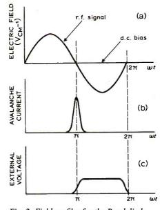
Fig. 2. Field profiles for the Read diode. Note the narrow avalanche region with peak current delayed 90° on peak voltage.
