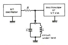
Fig. 6. Resonance testing circuit.
