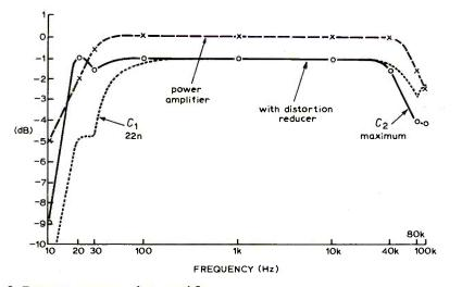
Fig. 8. Frequency response of test amplifier.
