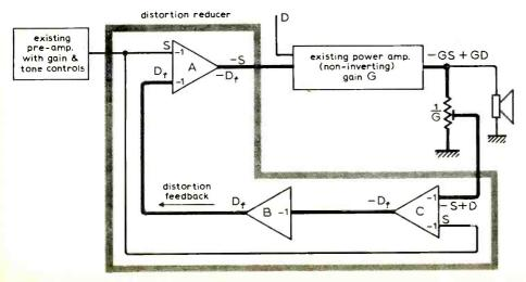
Fig. 2. Distortion reducer with non-inverting power amplifier.
