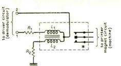
Fig. 5. Typical electrically biased keying relay (Carpenter type 3SE1, 250 $\Omega$  coils or similar).
