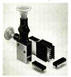
The "Clip-a-Dip" extraction tool has jaws which clamp under the pins of an i.c. and ensure a positive grip on the device during de-soldering operations. Both "Dip-a-Dip" and "Clip-a-Dip" are also available for d.i.l. i.cs with up to forty pins. Industrial Electronic Components Division, Guest International Ltd., Nicholas House, Brigstock Road, Thornton Heath, Surrey, CR4 7JA. **WW 329 for further details**
