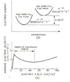
Fig. 5. (a) Energy band diagram for GaAs. The 0.36-eV level represents the quantum energy step between the two levels. (b) Velocity versus electric field for GaAs. Peak indicates the stage at which electrons jump from one level to the other and start to slow down.
