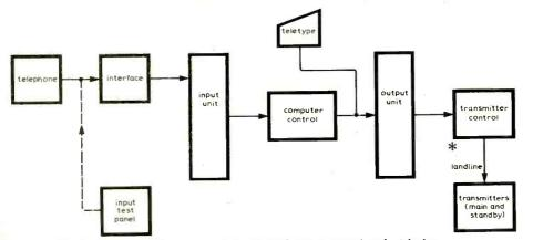
Simple block diagram of the computer and interfacing system'used with the **Post Office's new telephone radio-paging system (Also standby units up to\*)**.
