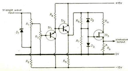
Fig. 7. A sine wave shaping circuit.
