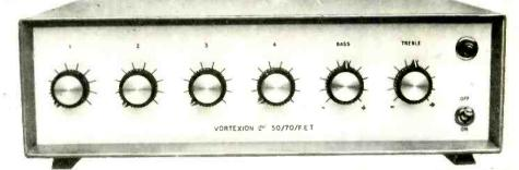
The mixer is arranged for 2-30/60  $\Omega$  balanced line microphones, 1-HiZ gram input and 1-auxiliary input followed by bass and treble controls. 100 volt balanced line output or 5/15  $\Omega$  and 100 volt line.
