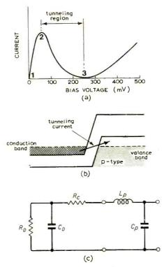
Fig. 6. (a) Typical I-V curve for the tunnel diode. (b) Valence and conduction bands for a p-n junction. Tunnelling current is a function of the amount of overlap of these bands. (c) Equivalent circuit of a packaged tunnel diode.
