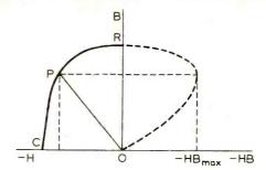
Fig. 6. The left-hand half is a "load-line" diagram for a permanent magnet material in series with an air gap, analogous to Fig. 4; the dotted lines are a construction for finding the best working point, P.
