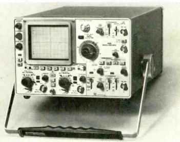
reference. Alternate sweep switching, to view intensified waveforms and delayed waveforms at the same time. When you move the intensified zone you always know precisely where you are, and still see the delayed waveform. It saves time and adds operation convenience. The price of the  $_{485}$  is  $f_{,2,051}$ .
