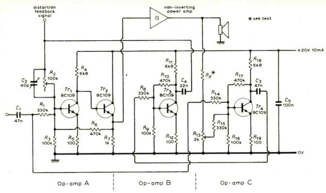
Fig. 5. Circuit of distortion reducer, for use with non-inverting power amplifiers.
