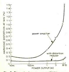
Fig. 7. Distortion/power curves of test amplifier.
