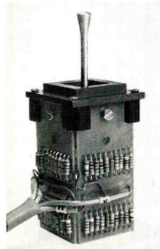
customer specification to meet a particular requirement. Specifications for standard versions are as follows:  $Z_i$  = output impedance of preceding stages is not to exceed 100 $\Omega$ .  $Z_o$  = load impedance of following stages is not to be less than 15,000 $\Omega$ . Insertion loss with joystick in centre (input to any output) = 2 × element value. Audiotek, Farringdon House, St. Albans Road East, Hatfield, Herts. WW 304 for further details.
