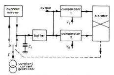
Fig. 1. A block diagram of the oscillator.
