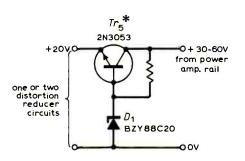
\*fitted with push fit 50°C/W heat sink
