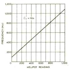
Fig. 4. The oscillator performance using the current generator shown in Fig. 4(a) demonstrating a linear frequency calibration.
