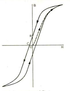
Fig. 3. For comparison with Fig. 1, a typical magnetization curve of transformer core material, taken from zero to maximum (dotted) and then over a complete cycle.
