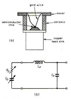
Fig. 3. (a) Typical package used up to 20GHz,  $10 \times full$  size. (b) Simplified equivalent circuit: overall effect of  $L_p$ and  $C_p$  degrades performance of the chip semiconductor
