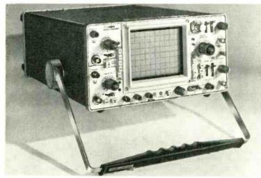
the Tektronix 453A and 454A. They have significantly more bandwidth, twice the sweep speed, a bright 25% larger (full  $8 \times 10$  cm) display and additional user conveniences, and all of this in a shorter, thinner, lighter and much lower-priced package.
