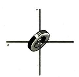
Fig. 8. One of the many ferrite ring cores in a computer magnetic store, encircling one each of the network of X and Y magnetizing wires. A third wire (not shown) is used to sense changes in the core magnetization.
