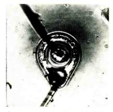
Silicon mesa transistor designed for high speed switching applications, with a current rating of 200mA and a maximum dissipation of 1W. The chip is 0.4mm square.
