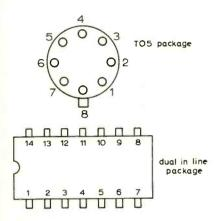
Fig. 3. Pin connections (top view).
