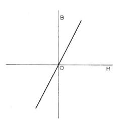
Fig. 1. Ideal magnetization curve for transformer core material, one of its advantages being complete absence of permanent magnetism.
