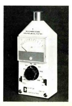
the connection of recorders and oscilloscopes or even a noise dosemeter. The meter can make measurements from 24dB to 140dB s.p.l. using the same microphone type as is fitted to most British units and thus microphone accessories are interchangeable. The CS17A is priced at £68 complete. Custom Electronic Associates Ltd, Castle Associates Division, Redbourne House, North Street, Scarborough, Yorks. YO11 1DE.
