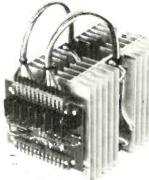
CONTROL AMPLIFIER TYPE EM73 Differential input. Automatic current limiting Automatic dynamic braking Uses linear devices throughout. 220V or 240V input.
