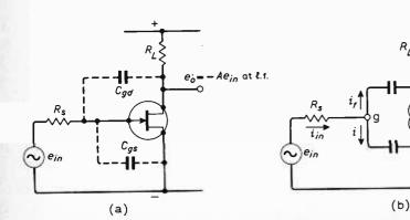
Fig. 8. The junction capacitances  $C_{gal}$  and  $C_{gs}$  limit the frequency response of the device.
