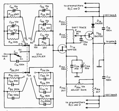
Fig. 6. One of the four input pre-amplifiers.
