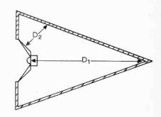
Fig. 4. Triangular cabinet showing different reflecting path lengths.
