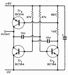
opposite base. The method of improving rise-time by using a diode to isolate the output from the coupling capacitor has the disadvantage that the rise-time is degraded by capacitive loads.
