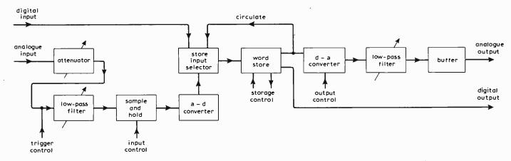
In this transient-event recorder, an analogue waveform is sampled, converted into digital form and successive numbers clocked through a store. After the event, the stored data are circulated and read out in digital or analogue form.
