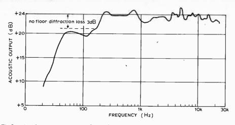
Fig.8. Anechoic response curve of complete loudspeaker system.
