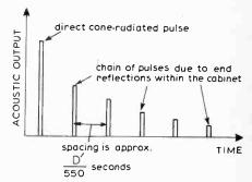
Fig. 3. Pulse-response (idealized) of cabinet shown in Fig.2.
