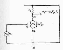
Fig. 6. (a) Common source amplifier and (b) its equivalent circuit.
