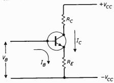
Fig. 1. Basic circuit of common-emitter stage.
