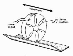
Linear motion is achieved by coupling surface wave energy of a piezoelectric disc to another surface.
