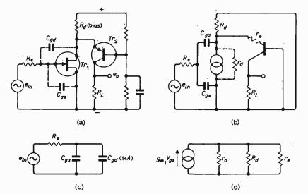
Fig. 11. Adding a bipolar transistor to reduce the term  $(1+A)C_{ad}$ . (a) The circuit; (b) equivalent circuit; (c) the input circuit and (d) the output circuit.
