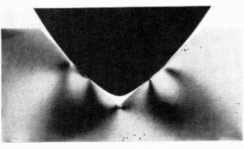
New Shibata stylus (top) developed by JVC claims to reduce record wear by reducing pressure to one-quarter of that with an elliptical stylus (bottom) and to improve phase and amplitude response. Stress patterns shown are for equal downward force.
