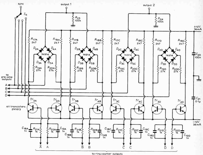
Fig. 7. The four linear transmission gates with the components for interfacing with the counter.
