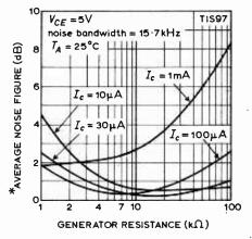
Fig. 6. Broadband noise figure is less than 2dB at  $I_C$  of  $100\mu A$  for a mean source resistance of  $5k\Omega$ .
