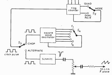
Fig. 2. Block diagram of the quadrupler in the quad mode.
