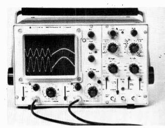
A dual-trace oscilloscope type OS3000 made by A dvance Instruments is a 40MHz unit having a 5mV/cm sensitivity at full bandwidth.
