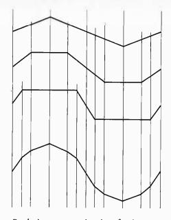
Producing an approximation of a sinewave by adding a triangular wave to clipped versions of the triangular wave.
