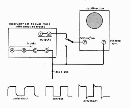
Fig. 9. Quadrupler alignment test circuit. Waveforms show the effect of attenuator trimming capacitor adjustment.
