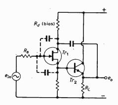
Fig. 13. Improved circuit using bootstrapped drain.
