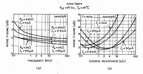
Fig. 4. Noise performance of a p-n-p transistor giving 2-dB noise figure at 1kHz with  $R_5 = 200\Omega$ .
