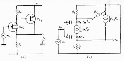
Fig. 16. Another circuit which shows how a bipolar transistor can be used to improve the basic f.e.t. circuit.
