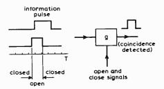
Fig. 3. Example of 'gating' a number of pulses (c) from a train of short pulses (a).
