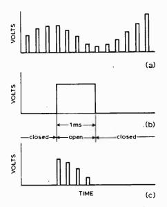
Fig. 4. Gate acting as a coincidence detector: (a) non-coincidence of pulses; (b) coincidence of pulses.
