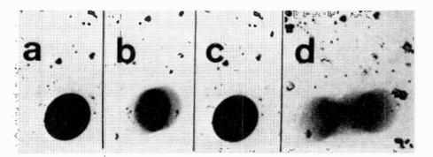
Cylindrical magnetic domain (a) can be displaced by application of a gradient fieldsinsusoidally varying in this case — to give a lateral force, on the bubble (b). Sensitivity can be increased (d) by addition of an auxiliary field of higher frequency. Photographs are taken by shining polarized light through a thin slice of material and then through an analyser, the plane being rotated according to direction of magnetization (Faraday effect).
