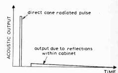
Fig. 5. Approximated output for triangular cabinet excited with impulse from loudspeaker. 215
