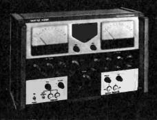
Autobalance Universal Bridge gives four-figure readout on all ten ranges covering every practical value of L, C, R & G. Sensitivity increases automatically when decade back-off controls are used but can be selected manually. External Standards sockets permit comparative measurements and increase discrimination to 5 or 6 figures. Accuracy 0.1%.
