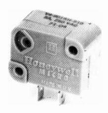
Both s.p.c.o. and s.p.d.t. versions are available with 0.187in quick-connect or solder termination. They are rated at 5A and 125 or 250V a.c. Inrush current values should not exceed 10A. Operating temperature range extends from -40 to +100°C. Honeywell Ltd. Charles Square, Bracknell, Berkshire.
