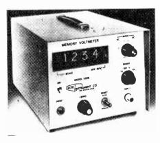
four-figure digital readout and an accuracy of 1% of full scale. There are four switched ranges with full-scale values ranging from 10mV to 19V. The input impedance is  $1\text{M}\Omega$ . The peak value is held in store until reset. Automatic reset for driving a printer or recorder is provided. The input is floating and is double screened to reject radiated transients. Other models in this range include instruments capable of measuring
