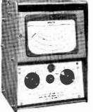
TF1041C VTVM A.C. voltage range 300 MV to 300V in 7 ranges. 20 Hz-1500 MHz. D.C. voltage ranges 300 MV-1000V in 8 ranges. D.C. resistance 50 ohms to 500 Mohms. Price £62.50.
