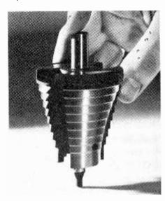
The bit is made of cobalt 'high speed' steel and has a 12.5mm diameter shank. Price £23 plus 35p postage and packing. West Hyde Developments Ltd. Ryefield Crescent, Northwood Hills, Northwood,
