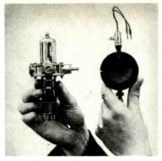
Examples of early klystron and magnetron tubes.
