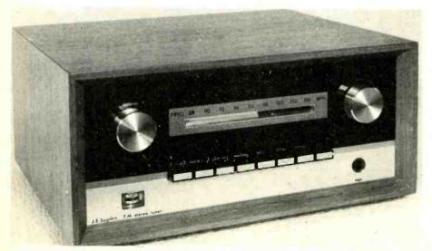
An f.m. tuner from J. E. Sugden employs a varicap tuned front end and a four stage i.f. section with double tuned couplings. A switchable filter permits reduction of L-R information thus allowing separation to be traded for reduced noise on weak signals.
