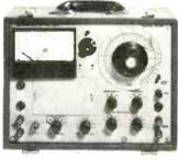
Transmission Measuring Set — portable equipment for checking a.f. lines and equipments from 20Hz to 120kHz. Suits 75, 140 and 600-ohm circuits, balanced or unbalanced, terminated or unterminated. Details on application, quoting 44C.
