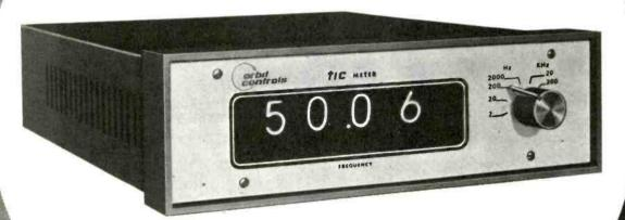
Long gate times at low frequencies are OUTI TIC Meters measure the inter-pulse period, t, of the input frequency, compute its reciprocal, and display the result as frequency to a high accuracy. Basic Sampling time is t+1 seconds. In the higher ranges, t is averaged over 10 or 100 periods.
