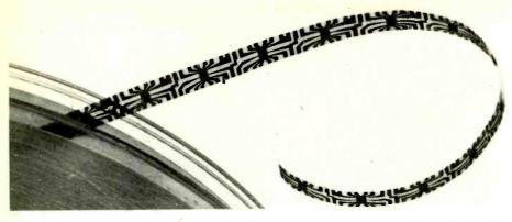
The metalization pattern on the Polymide film can be clearly seen. Integrated circuit chips mounted in this way could easily be used in automatic assembly machines.
