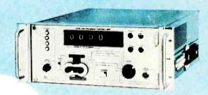
The Type 240 Programme Control Unit, in conjunction with a disc memory, can programme the 568/230 at speeds up to 100 measurements per second.
