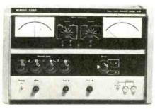
Capacitor Test Set – direct readout of percentage deviation from a pre-set value, and of dissipation, with automatic limit circuits showing pass/hign/low. Also 4-figure capacitance measurement. Ask for B700 Data Sheet.
