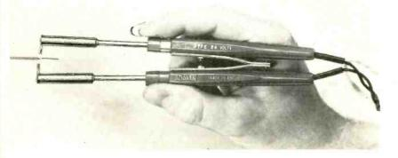
The ADAMIN thermal wire strippers allow one-handed operation, using a simple tweezer action.
