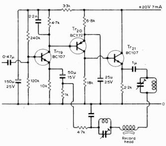
Fig. 29. A feedback recording output stage.
