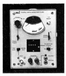
errors in 24- and 32-channel equipment at bit rates of 1.536 and 2.048 Mbits/sec. A meter indicates presence of a signal and errors. A totalizer displays total errors over any period of time. It has an internal 9V battery. Marconi Instruments Ltd, St. Albans, Herts.
