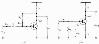
Fig. 5. A single-stage amplifier with (a) parallel-derived, parallel-injected feedback and (b) series-derived, scries-injected feedback.
