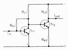
Fig. 8. Skeleton form of two-stage current amplifier.
