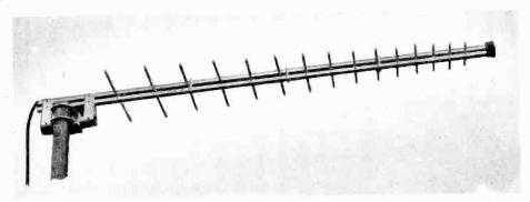
Fig. 3. Aerial and mount adjustable for either horizontal or vertical polarization.
