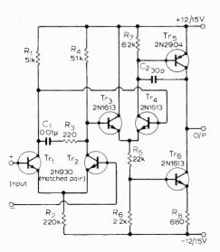
Fig. 1. Discrete component operational amplifier.
