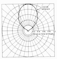
Fig. 5. Radiation pattern at 650MHz for vertical polarization.
