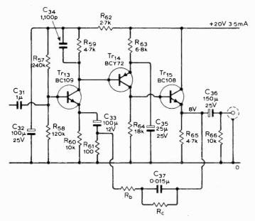
Fig. 27. A discrete-component replay amplifier.
