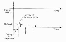
Fig. 5. Circulating pulse in feedback amplifier.
