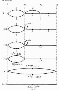
Fig. 6. Rules for feedback loops, self-loops and node elimination.
