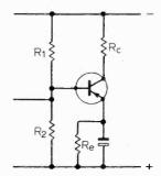
Fig. 6. Mean collector current stabilization by means of a potential divider and emitter
