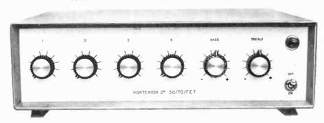
**100 WATT ALL SILICON AMPLIFIER.** A high quality amplifier with 8 ohms—15 ohms or 100 volt line output for A.C. Mains. Protection is given for short and open circuit output over driving and over temperature. Input 0.4 V on 100K ohms.
