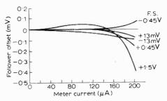
Fig. 4. Plot of offset voltage vs meter current for five scales ( $\pm 15 \text{mV}$ ,  $\pm 0.5 \text{V}$  and  $\pm 1.5 \text{V}$ ) by changing  $R_s$  shows total variation in offset is within 0.1 mV on  $\pm 15 \text{mV}$  scales. This shows feasibility of a + 5 mV scale at  $\pm 1\%$  error.
