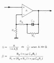
Fig. 31. Replay amplifier equivalent circuit.
