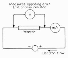
Fig. 2. Simple circuit illustrating work done by an e.m.f. source in moving electrons against resistance. The e.m.f. could be varied to form a signal.
