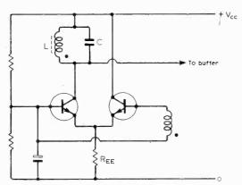
Fig. 25. A current-switching oscillator.
