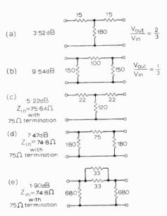
one should select the resistors using a bridge, and not merely pick  $\pm 20\%$  components at random from the spares box.
