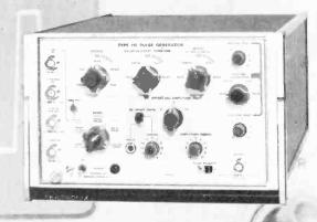
The Type 2101 is a compact, 25-MHz, 10-volt, general purpose generator with SIMULTANEOUS positive and negative going pulse outputs. Switch positions are provided for selection of a specific pulse period, duration and delay, within the calibrated range of the respective control. Weighs only  $8\frac{3}{4}$  lb. Price £334 plus £47 cuty
