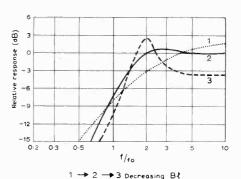
Fig. 5. Effect of Bl on response of small closed box.
