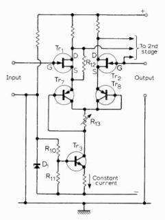
Fig. 2. Circuit compensates for bias differences by using diodes  $(Tr_{\gamma} \& Tr_{s})$  to approximate constant voltage devices.
