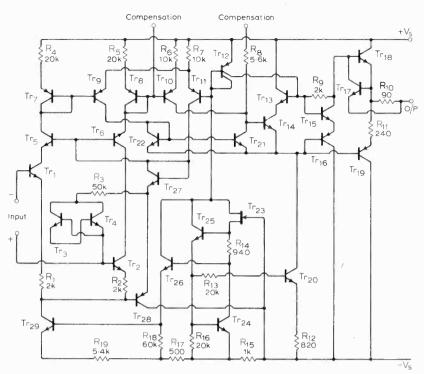
Fig. 6. Third generation example, the LM108. Tr, and Tr, are 'super-gain' or 'punch-through' transistors which operate at very low voltages.
