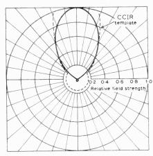
Fig. 4. Radiation pattern at 650MHz for horizontal polarization
