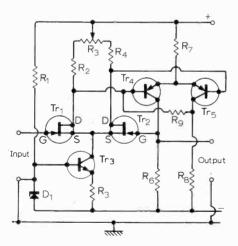
Fig. 1. Basic voltage follower circuit. Field-effect-transistor differential amplifier gives high input impedance with low offset voltage. Low output impedance is achieved by both negative feedback from  $Tr_4$  collector and positive feedback from  $Tr_5$  collector.
