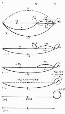
Fig. 7. Solution of the signal-flow graph of Fig. 1 by successive node elimination.
