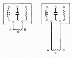
Fig. 2. We can move R away from the system on the end of a line of characteristic impedance R.
