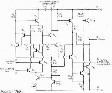
possible to include capacitors and so terminals 1, 8 and 5 were provided to enable separate external compensation capacitors to be connected. The  $220 \mathrm{k}\, \Omega$  resistor  $R_2$  in Fig. 1 also could not be provided in the monolithic version, and was replaced by the constant current transistor,  $Tr_{11}$ , in Fig. 2.
