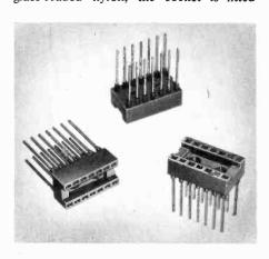
with pre-tensioned double wiper blade contacts. These have a life expectancy of up to 10,000 insertions with a typical contact resistance of 7 to  $10 \text{m}\Omega$ . Jermyn Industries, Vestry Estate, Sevenoaks, Kent.
