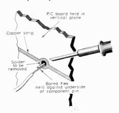
The wire "brush" used should be of reasonably new and clean multi-strand flex, such as  $23 \times$  No. 36 s.w.g. A 1 to  $1\frac{1}{2}$ in. end should be stripped, gently twisted, and liberally treated with flux. The tip of the iron should be clean with, obviously, a minimum of solder on its surface. More than one application, using a fresh brush each time, may be needed if there is much
