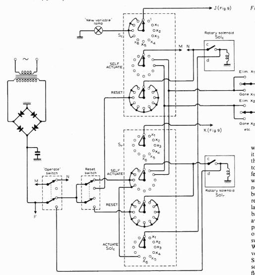
$S_r$  and  $S_c$  in the control box are replaced by switches operated by rotary solenoids designated  $Sol_r$  and  $Sol_c$  in Fig. 11.  $Sol_c$  operates three banks of contacts;  $Sol_r$  operates four banks. Each bank is a one-pole 11-way switch. In the twelfth position the moving contacts are connected to themselves. The banks  $S_r$  and  $S_c$  are connected to the display board exactly as shown before in Fig. 9.
