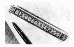
claimed to be more reliable than separate tubes. It uses a mixture of gases to give a luminance of 600cd/m². Coincident pulses of greater than 150µs are used to illuminate digits. Separate cathodes are provided for decimal points. Flicker can be eliminated by using an alternating supply of over 70Hz. Mullard Ltd, Torrington Place, London WC1E 7HD.
