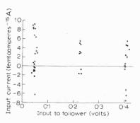
Fig. 7. Measurements of follower input current over two-week periods show input current is within  $\pm 10^{-14}A$  and that compensation reduces input current by 200.
