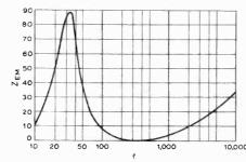
Fig. 3. Motional impedance circuit of moving coil loudspeaker in free air.
