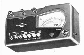
A portable lightweight insulation test set suitable for measuring the insulation resistance of all components, installations, etc. Cranking is obviated by the utilisation of a transistor converter; the power supply being two  $4\frac{1}{2}\text{-volt}$  dry batteries. The test voltage and range are selected by push buttons which facilitate quick and easy reading of the resistance value.
