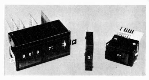
binary, and binary with complement. Multi-pole switching is achieved by coupling together a switch and up to four slave modules. Terminations are for direct wiring or for edge connectors and are numbered. Contact rating is 100mA at 50V d.c. Life is specified as being not less than 10<sup>6</sup> operations. Dimensions of the switches are height 33mm, width 8mm. Professional Component Division, Plessey Components Group, Abbey Works, Titchfield, Fareham, Hants.
