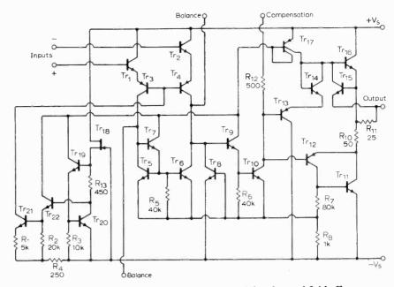
Fig. 5. Second generation example, the LM101A. Both bipolar and field effect transistors are used.
