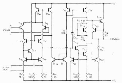
Fig. 4. The µA741. Note the diffused compensation capacitor.
