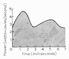
Fig.3. Graph of a signal in which information is represented by a variation of power with time.
