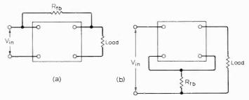
Fig. 4. General circuits for (a) parallel-derived, parallel-injected feedback and (b) series-derived, series-injected feedback.
