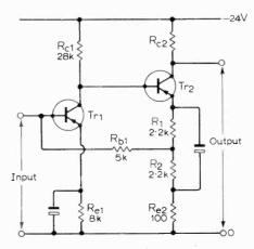
Fig. 9. More detailed version of the circuit in Fig. 8, designed for a current gain of 50.
