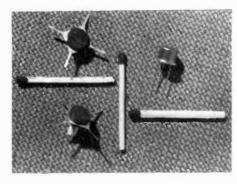
housed in a TO-39 package. The first two give an output of 3 watts at 470MHz from a drive of 350mW and a power supply at 13.8V. Output is limited to 2 watts in the
