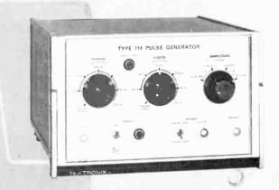
The Type 115 is a 10-MHz, 10-volt, general-purpose pulse generator with separately variable risetime, falltime, width, delay, period, amplitude and baseline offset. It is intended for use in applications where a variety of pulse amplitudes, polarities, shapes and other characteristics are required.
