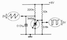
The s.c.s. has been in use for many years, why give it a new name? The circuit shown above, using a General Electric 3N58, produces much the same result as Fig. 14 in Mr. Greiter's article.
