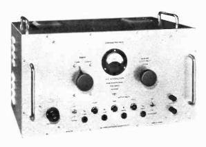
This instrument has been designed to fill the need for a very stable supply with a high purity of waveform for precision A.C. measurements. The uhit is extremely simple in operation and is fitted with protective devices and alarms which automatically prevent any possibility of damage it does not require any adjustments in setting up other than the output voltage selection. Output current:— 1 ampere maximum for stabilisation range of  $\pm~7\%$  change of input voltage
