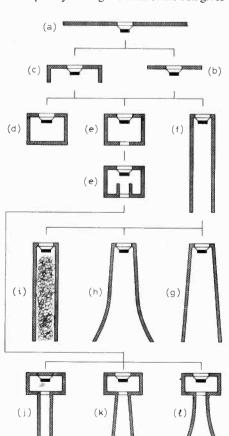
Fig. 1. The lineage of loudspeaker baffles.
