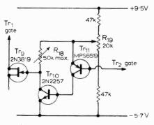
Fig. 6. Feedback circuit for raising input impedance. With this circuit voltmeter reading changed by only 1% of full scale in 30 min with a 0.01µF input capacitor (self time constant 400 days).
