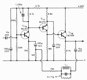
Fig. 28. Recording equalized amplifier.
