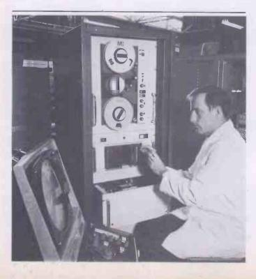
Designed primarily for air traffic control use by Solartron the interface equipment shown allows a standard television tape recorder to be used to record radar data for subsequent analysis on a radar display.
