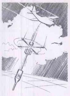
The sketch shows a device called EROWS (Expendable Remote Operating Weather Station). The eight-foot arrow-like structure implants itself in the ground after being dropped from an aircraft. The device is turned on remotely and it begins to transmit information on wind speed and direction, atmospheric pressure, temperature, humidity, precipitation and cloud cover. EROWS is being developed by Honeywell for the U.S. Air Force.
