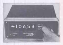
Weston standard cell. Zero offset current and voltage are automatically corrected between each reading. Series-mode rejection at mains supply frequency and its harmonics is greater than 85dB, and common-mode rejection 100dB at mains frequency and d.c. with  $1k\Omega$  imbalance in the input leads. The price is £25. International Electronics Ltd, Ewood Bridge, Haslingden, Lancs. WW303 for further details
