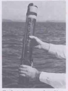
This floating beacon manufactured by Burndept, which has already captured orders worth £50,000 from Norway, operates on a primary battery and transmits on both the civil and military aviation distress frequencies (121.5 and 243MHz) for a minimum of 48hrs at 0°C. It measures 670 × 85mm and weighs 2.89kg.
