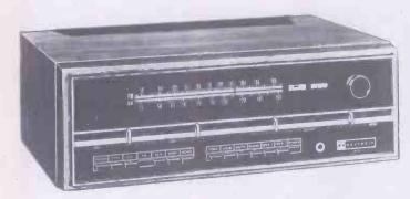
Model AR-19. AM-FM multiplex stereo Tuner/Amplifier. 30 watts (IHF) power output each channel, with less than 0.25% THD (8 ohm load). Can be used with all types of pick-ups. Linear motion controls Tuner sensitivity 2.0 uV (IHF). FM stereo separation 35dB at midfrequencies. New FET front end. Four I/C stages. Electronically regulated power supplies. Choice of Walnut or Teak cabinet. KIT PRICE £118. 0. 0.
