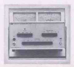
Meter, type TF2337, is complementary to the more elaborate Marconi Instruments TF2331 announced in 1964 and intended for development work. Level is set to give adequate meter deflection at either 400Hz or 1kHz and distortion factor read directly from the other meter. Provision is made for injection of external fundamental frequency in the range 30Hz-7kHz.
