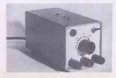
than 5000 to 1. On full load the ripple and noise do not exceed  $500\mu V$ , reducing to less than  $30\mu V$  for load currents below 50mA. A.D.M. Electronics, P.O. Box 3, Merthyr Tydfil, Glamorgan. WW310 for further details
