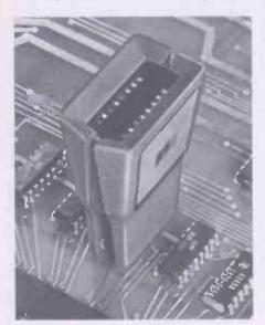
logic states of all 14 or 16 pins. The clip has 16 light-emitting diodes, each of which follows voltage-level changes on one pin.
