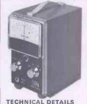
Input sensitivity 100MV MAX. INPUT 50 Volts Input Imput Sensitivity 100MV MAX. INPUT 50 Volts Input Impudence 10K, Zero Fraguency 3KHZ + or -0.1 percent
