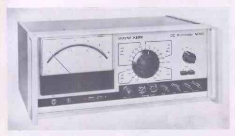
Wayne Kerr stand during the I.E.A. exhibition earlier this year, also measures direct voltage and resistance. Amplifier uses photochopper stabilization with 40-Hz switching to avoid beats with the 50-Hz supply. Instrument also features a small reverse scale for null detection, overload protection, one set-zero control for all ranges, a recorder output of 0-1mA at  $1k\Omega$ , and a hum rejection filter which rejects hum equivalent to  $50 \times f.s.d.$
