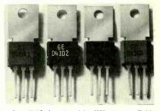
pairs: D40 brown, 1A 6W, n-p-n; D41 black, 1A 6W, p-n-p; D42 red, 3A 12W, n-p-n; D43 green, 3A 12W, p-n-p. Each type is available with 30, 45 or 60V continuous rating, with a wide range of gains up to 30. The flat pins are easily formed to TO5 or TO66 configurations. 100 up prices range from 7s 8d to 21s. Jermyn Industries, Vestry Estate, Sevenoaks, Kent.
