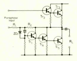
Fig. 1. Symmetrical output stage using only n-p-n transistors.
