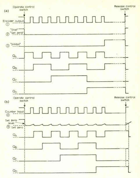
Fig. 4. (a) Coder and (b) decoder waveforms.
