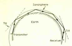
Fig. 6 Chordal hop. At the first and last reflection points, the ionosphere behaves as if tilted slightly towards the terminals. For tangential radiation (i.e. zero deg.), and tilt, however small, prevents a return to earth until a tilt of opposite sign occurs. (Ionosphere not to scale.)
