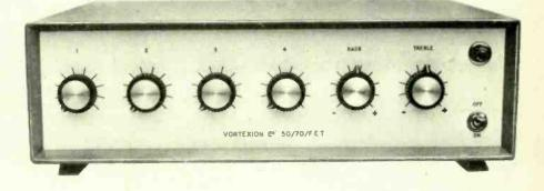
100 WATT ALL SILICON AMPLIFIER. A high quality amplifier with 8 ohms-15 ohms or 100 volt line output for A.C. Mains. Protection is given for short and open circuit output over driving and over temperature. Imput 0.4 V on 100K ohms.
