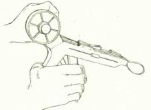
The first is called Tyton – an 'off-thereel' system that binds 50% faster than any other comparable system. The second is Kabelrap – a heavy duty version using 'one-piece' ties.
