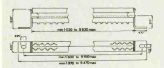
5 to 85 way single sided with solder and printed wiring tails. 10 to 170 way double sided with solder and printed wiring tails. Wire Wrap and Crimp tails will shortly be available.
