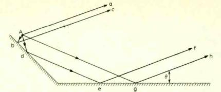
Fig. 3 Ground sloping down into the sea. The direct wave Aa, foreground reflection Abc, distant reflection Agh, and double reflection Adef add in phase if  $\theta$  is small, hg  $\approx \lambda/(4 \sin \theta)$ , h<sub>5</sub>,  $\approx \lambda/(4 \sin \theta)$ , these being the heights of A above ground and sea respectively.
