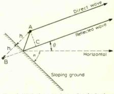
Fig. 2 With the aerial at a height h above ground sloping at an angle  $\infty$ , the direct and reflected waves are in phase when 2h sin ( $\alpha + \theta$ ) =  $\gamma \lambda/2$ . For small values of  $\theta$  this becomes 2h sin  $\infty \approx \lambda/2$ . This diagram is identical with Fig. 1 except for rotation through the angle  $\alpha$ , and the increased ground angle.
