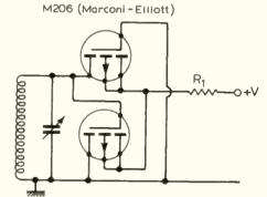
Fig. 2. Arrangement for operation between 50 kHz and 350MHz.
