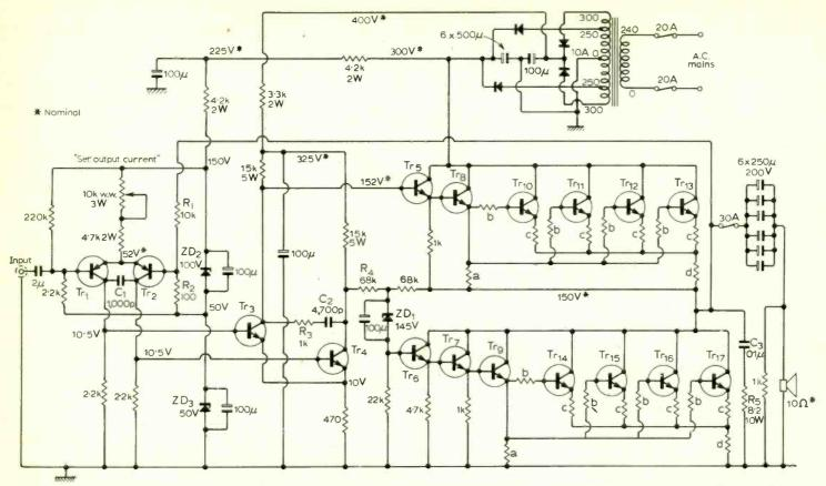
Fig. 2. Expanded version of Fig. 1 employing a Darlington triple as the output device.  $Tr_1$ ,  $Tr_2$ —R.C.A. 38496;  $Tr_3$  to  $Tr_7$ —MJE340;  $Tr_8$  to  $Tr_{17}$ —MJ413. Lettered resistor values:  $a = 22\Omega$ , 2W;  $b = 10\Omega$ , 2W;  $c = 0.5\Omega$ , 5W; and  $d = 0.1\Omega$ , 5W.
