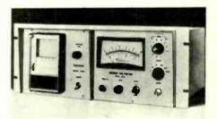
low frequency and where unwanted highfrequency noise is present. Voltage ranges are 0-3, 30, 100, 1000V to 30kV with optional probes. Input impedance is 10MQto 30kQ depending on the range and accuracy  $\pm 3\%$  of full scale. Sintrom Electronics Ltd, 2 Castle Hill Terrace, Maidenhead, Berks.
