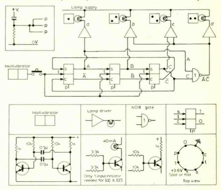
Fig. 2. The suggested circuit for a digital dice, the method of display is left to the reader, almost any general-purpose silicon transistors may be used.
