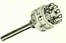
standard torque setting is 200 gm/cm; 400 and 600 gm/cm can be supplied to order. A ceramic wafer and gold-plated stud contacts are used. Contact resistance is better than  $5m\Omega$  and wafer insulation better than  $10^{12}\Omega$ . Switching capacity is up to 1A. Radiation Components Ltd, 76 Crown Road, Twickenham, Middlesex. WW 309 for further details
