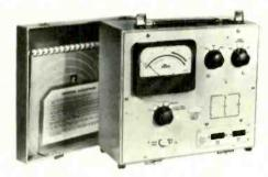
1MHz. The instrument is protected against overloads of up to +25dBm on all inputs and the measurement range of -1 to +1dBm is displayed over the full 4-in scale of the meter. The accuracy of the standard version is  $\pm 0.05$ dB on all inputs. However, it is now available as option 1 with special calibration charts guaranteeing an accuracy of 0.02dB on all three inputs. Hatfield Instruments Ltd, Burrington Way, Plymouth PLS 3LZ, Devon.
