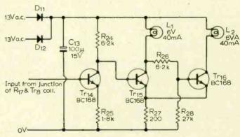
Fig. 7. Overload indicator circuit.
