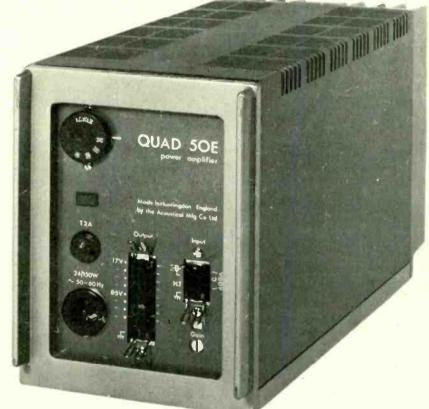
**INPUTS** – 0.5 Vrms unbalanced with provision for an optional plug-in transformer for bridging 600 ohms lines. **OUTPUTS** – isolated providing 50 watts into almost any impedance from 4 to 200 ohms. **DIMENSIONS** –  $12\frac{3}{4}$ " x  $6\frac{1}{4}$ " x  $4\frac{1}{2}$ "
