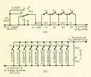
Fig. 9. (a) Construction of  $R_V$ ; (b) Contruction of  $R_c$ .
