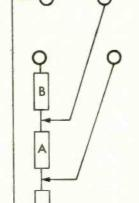
4-terminal connections minimise lead and contact resistance errors. Bridge measures A, ignoring B & C.
