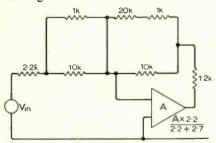
Fig. 2. High-frequency equivalent circuit.
