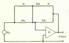
Fig. 3. Unity-gain version of Fig. 2 omitting  $R_1$ ,  $R_2$  and  $R_3$ .
