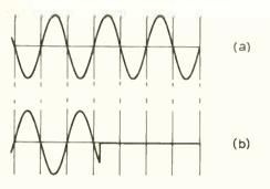
Fig. 6. Instead of switching on, as shown in Fig. 5, one signal is switched off.
