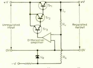
Regulated output voltage  $V_0 = R_v \frac{V_R}{R_k}$   $V_0 \propto R_v$  if  $\frac{V_R}{R_k}$  is constant
