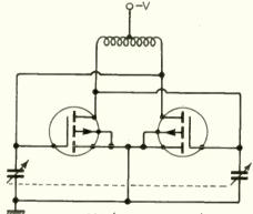
M206 (Marconi-Elliott) Fig. 1. Oscillator operating up to 300MHz.
