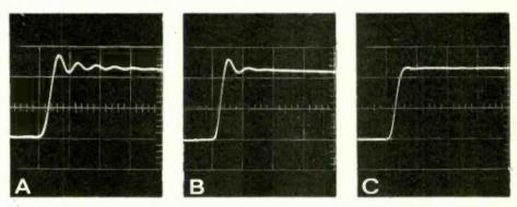
Fig. 16. Step responses of three filters: (a) a 5th-order Darlington, (b) a 5th-order Butterworth, (c) an approximate linear-phase filter.
