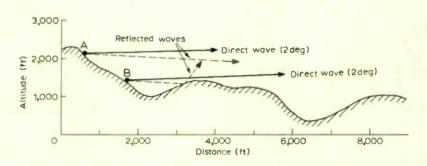
Fig. 4 Typical ground profile for mountainous country. Distant low-angle reflections are non-existent for transmitter at B, and probably unimportant (due to break up of Fresnel zones) for transmitter at A. In both cases low-angle reflections (not shown) are obtained from the foreground. (Isle of Mull, grid ref. NM 568332 bearing 104 deg.)
