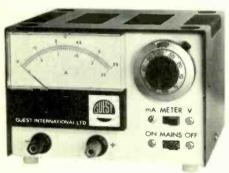
ability. A built-in meter enables the output voltage or current to be monitored. Ripple noise is less than 0.5mV pk-pk and overload protection limits the output current to 110% of maximum. Reset is automatic. The model 606 is available in current ranges from 0-500mA up to 0-2.5A. Dimensions are  $156 \times 152 \times 102$ mm and prices from £34 15s to £42 15s. Guest International Ltd, Nicholas House, Brigstock Road, Thornton Heath, Surrey. WW318 for further details.
