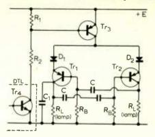
suitable are: diode IN4148 (G.E.); transistors (Ferranti plastic 'E' line) ZTX 500. B. L. HART,
