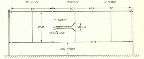
Fig. 7 Low-angle aerial for 7MHz. Height not critical. Reflector and director tunable, by adjusting length of verticals or of the lower horizontal wires. Dimensions approximate.
