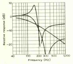
Fig. 5. Measured responses of the individual stages of a filter as Fig. 4, scaled to give -3 dB at 159 Hz.
