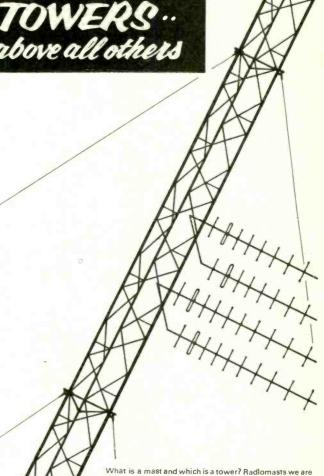
called, but that does not mean we only build masts. This is a mast, on this occasion: a slim structure supported by stay-wires. A tower is generally wider and tapered, and supports itself without stays. They both have their separate advantages.
