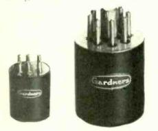
to the existing types, now have a 20,000V capability to meet the Post Office requirement. They are protected mechanically by a new filling of closed-cell epoxide resin foam compound (the smaller types are vacuum-impregnated with a microcrystalline wax). Advanced technical data sheets AT15, AT16 and AT17 are available from the makers. Gardners Transformers Ltd, Christchurch, Hants., BH23 3PN.
