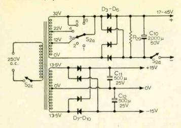
Fig. 8. The d.c. supply circuits.
