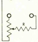
Potentiometer ratios can be related to angular rotation. Bridge reads  $R \times (1/ratio)$ .
