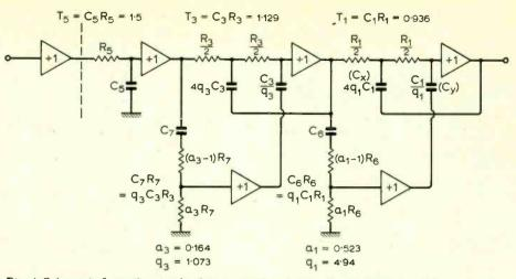
Fig. 4. Schematic for realization by factors of 5th-order Darlington response with 0.1 dB ripple in the pass band, 40 dB minimum attenuation in the stop band, and cut off at 1 radian/second.
