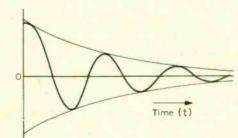
Fig. 1. The shape of  $exp(-\alpha t) cos(\omega t)$ enclosed in the decay curve  $exp(-\alpha t)$ .
