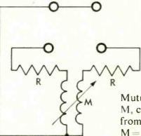
Mutual Inductance, M, can be derived from bridge C reading:  $M = R^2.C.$
