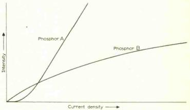
Fig. 5. Current density versus intensity plot of a single gun, dual-phosphor c.r.t. for producing multicoloured displays.
