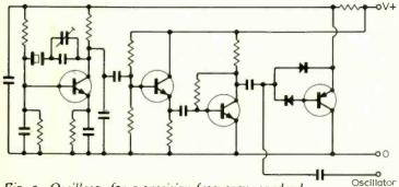
Fig. 5. Oscillator for a precision frequency standard incorporating buffered output and level control.
