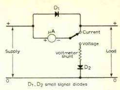
In situ current and voltage metering circuit.
