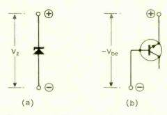
Fig. 1. (a) Ordinary zener diode, and (b) a "zener transistor".
