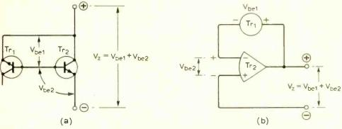
Fig. 2. Circuit configuration of an active zener (a) and its equivalent circuit (b).
