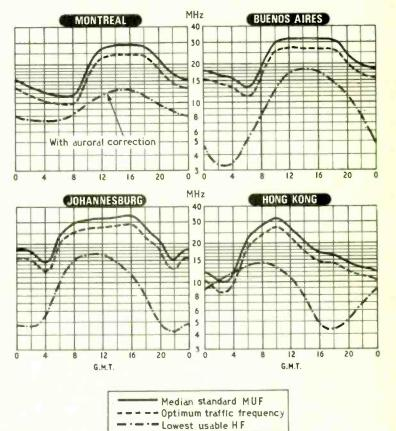
The prediction curves show the median standard MUF, optimum traffic frequency and lowest usable frequency (LUF) for reception in this country. Unlike the standard MUF, the LUF is closely dependent upon such factors as transmitter power, aerials, and type of modulation. The LUF curves shown are those drawn by Cable & Wireless Ltd, for commercial telegraphy and assume the use of transmitter power of several kilowatts and rhombic aerials.
