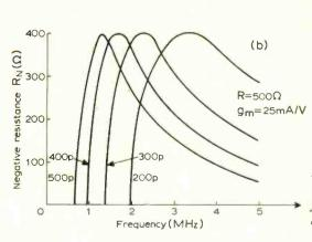
Fig. 3. Negative resistance  $R_N$  as a function of frequency (a) for  $R=700 \Omega$  and (b) for  $R=500 \Omega$ .
