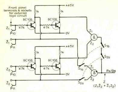
Fig. 79. Circuit that enables the instrument to display the output from one or other of two external logic circuits or to display the difference between the two circuits.
