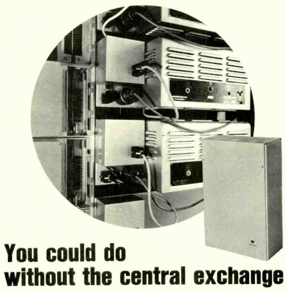
So we designed the Philips Intercom M 100 system, the first all-electronic decentralized duplex intercom on the market. The M 100 system eliminates the usual complicated central exchange with its dustproof and climatized room. Instead there's a small supply unit (76 x 50 x 20 cm) that plugs in anywhere along the cable.
