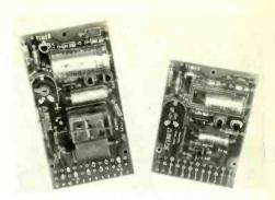
cally for driving external relays, reed switches or thyristors. Connection of all types is either by permanently wired solder tags or, to provide easy interchangeability, by means of a 12-way plug-in edge connector. Screw fixing holes are also provided so that the module may be rigidly attached to a suitable mounting face if desired. Deltic Automation Ltd. Tillys Lane, Staines, Middlesex.
