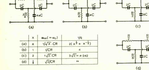
The frequency of the null is found by equating the numerator of the frequency-response function to zero,  $I - \omega^2 T_1 T_2 = 0$ , which gives  $\omega_{\infty} = I/\sqrt{(T_1 T_2)}$ ; and it can be seen from the denominator that this is also the undamped natural frequency of the network,  $\omega_0$ . Hence
