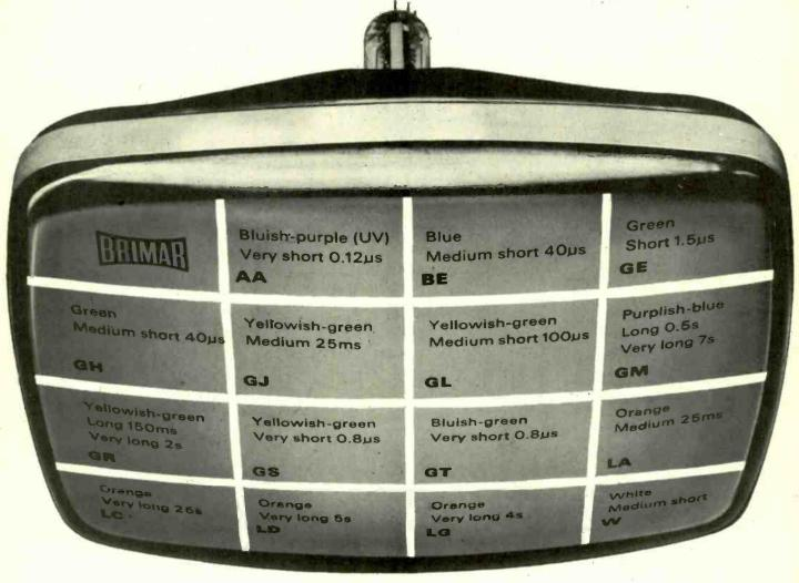
Fifteen different phosphors, from a very short persistence blue-purple (0.12µs) to a very long persistence orange (25s), together with optional extras such as internal and external graticules, are offered by Brimar to users of cathode ray tubes.
