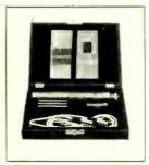
B.M.5. Studio quality Stereo ribbon microphone. Figure of 8 response: Sections may be swivilled up to 90° relative to each other for the desired stereo effect. Fitted with music/ speech switch. Response 30 - 13,000 Hz ±2.5 dB . Sensitivity 85 dB below 1 volt/µbar. Hum sensitivity - 146 dB. Output 200 ohms at 1 KHz. via 9 ft lead, 5 pin DIN plug. Supplied in rosewood
