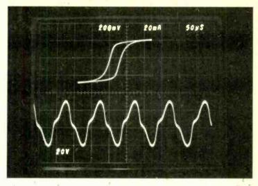
Fig. 4. A polaroid photograph of the screen of the Tektronix 7704 oscilloscope showing the automatic scale factor readout produced by a built-in character generator.
