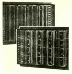
holes or local copper pads will take Vero terminal pins for inter-connections. Location patterns can be screen printed on the component side. The new design permits cooling by natural convection as the dual-in-line packages are mounted in the vertical plane and so allows maximum airflow between rows. These boards are available on epoxy glass or s.r.b.p. base material. Vero Electronics Ltd, Industrial Estate, Chandler's Ford, Hampshire.
