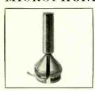
Beomic 1000 Omni-directional moving coil microphone. Response  $50 - 17,000 \text{ Hz} \pm 2.5 \text{ dB}$ . Sensitivity 0.1 mV/µbar. Hum sensitivity - 139 dB. Output: 200 ohms at 1 KHz. via 9ft lead, 5 pin DIN plug. Supplied with frequency response chart, lavalier cord, anti microphonic base, and packed in a futuristic container. Price \*£9.9.0d.
