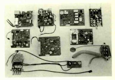
Replaceable modules constituting the circuitry of the British Radio Corporation's new single-standard colour television receiver (chassis type 3000).
