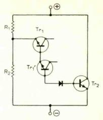
Fig. 4(a and b). Possible alternatives for current boosting without an undue increase in stand-by current.
