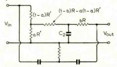
Fig. 19. High-pass unsymmetrical notch network-reduced input to l.p. path obtained by potential divider.
