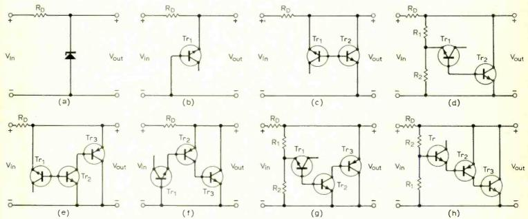
Fig. 6. (a) Zener diode shunt regulator, (b) "zener transistor" shunt regulator, (c) "active zener" shunt regulator, (d) "active variable zener" shunt regulator, (e and f) alternative "active zener" shunt regulators with boosted output current, (g and h) "active variable zener" shunt regulators with boosted output current.
