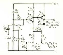
flow through the feedback resistor  $R_8$ , and thus the output stage unbalance, is only  $1.5-2\mathrm{mA}$ . Even this can be reduced by the addition of  $R_D$ , (shown dotted). In my own amplifiers, this has reduced the d.c. in  $R_8$  to  $50\mu\mathrm{A}$ . The values of  $C_A$  and  $C_B$  may seem excessively large, but this has been done deliberately to maintain the amplitude and phase of the a.c. feedback at the extreme low-frequency end of the audio spectrum.
