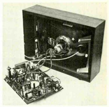
Monochrome single-standard receiver by B.R.C. with almost all electronic circuitry on a single printed-circuit board (chassis type 1500).
