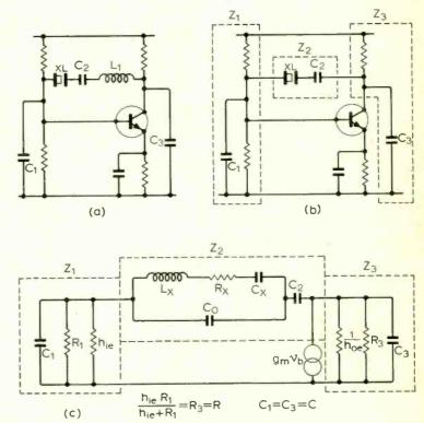
Fig. 1. Common crystal oscillator circuit (a) and with  $L_1$  removed (b). The equivalent circuit of (b) is given at (c).
