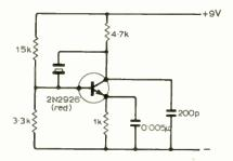
less than 18 crystals duly showed life: there was one non-oscillator, an old regrind of an ex-service FT243 (8012 kHz), presumably not etched. Most of these crystals were over 20 years old. The oscillation frequencies did not differ greatly from the marked values: they depend, of course, on the oscillator actually used.
