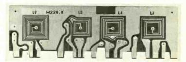
Printed-circuit coils used in the i.f. section of the type 1500 B.R.C. single-standard monochrome receiver.
