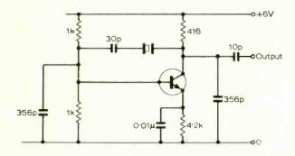
Fig. 4. 2.5-MHz oscillator incorporating calculated values.
