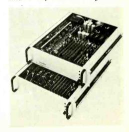
synchronous and asynchronous gating, double pulse operation, square wave modes, and external trigger. The dual timing unit is offered for applications requiring two independently controlled pulses, both from a common clock source. It contains a single repetition rate circuit, two delay circuits and two width circuits, with two independent outputs. One model 145 may be a complete dual pulse system. Aveley Electric Ltd, Arisdale Avenue, South Ockendon, Essex, RM15 5SR.
