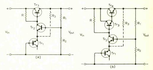
Fig. 7. (a) A simple "zener transistor" (Tr<sub>1</sub>) series regulator, and (b) with boosted output current.
