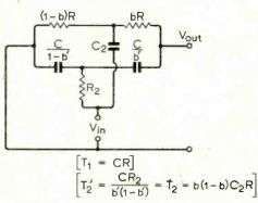
Fig. 20. Balanced parallel-tee network with output taken for "tuned-circuit" or band-pass response with | Vout/Vin | (max)
