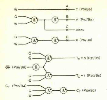
Fig. 83. Logic circuit needed to provide simultaneous display of a Venn diagram, Karnaugh map and Truth table
