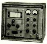
SIGNAL GENERATOR TYPE TF 937 (CT 218). Frequency range:—35 kHz-30mHz. 50 ft. Frequency scale. 200 kHz to 2MHz. Built-in Crystal calibrator Sinewave A.M. V.F.M. Output:—D.19V-IV £95. Carriage 30/-.
