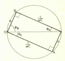
Fig. 13. Showing the 90° phase difference between the voltages at A and B when  $T_2' = T_2 = CR$ .
