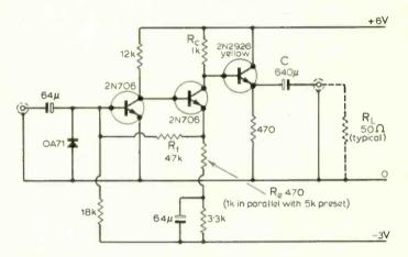
Circuit diagram of direct-coupled wideband amplifier
