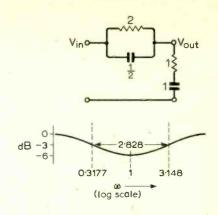
Fig. 10. Inverted Wien-bridge network showing relative component values for minimum bandwidth when maximum attenuation is 6dB.
