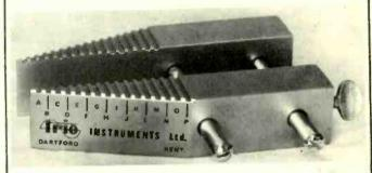
An easily adjusted hand tool for the accurate bending of resistor, capacitor, diode leads, etc., for printed circuits. Will bend leads to within  $\frac{1}{16}$ " of ends of components and up to  $3\frac{1}{4}$ " centres.
