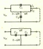
Fig. 11. Network of Figs. 9 (a) and (b) redrawn to show the two paths between input and output.
