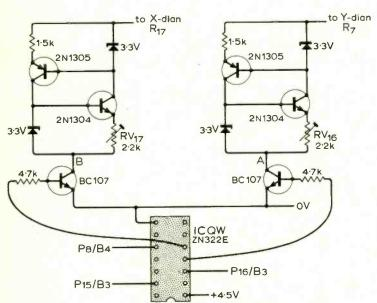
Fig. 81. Details of the circuitry needed to provide four display areas
