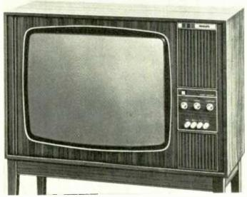
The Philips 511 single-standard colour receiver, which has a 22in screen.
