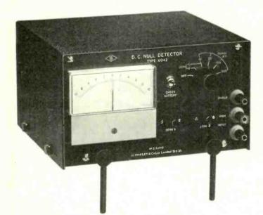
TYPE 6042 uses an F.E.T. Chopper followed by a solid state a.c. amplifier with large open scale output meter.
