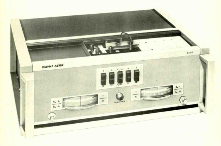
DIRECT READOUT of immittance at frequencies from 100kHz to 10MHz, with real and quadrature terms shown simultaneously, in equivalent series or parallel form as appropriate.
