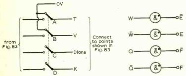
Fig. 84. Circuit which can be added to Fig. 83 to provide a six-variable Karnaugh map facility
