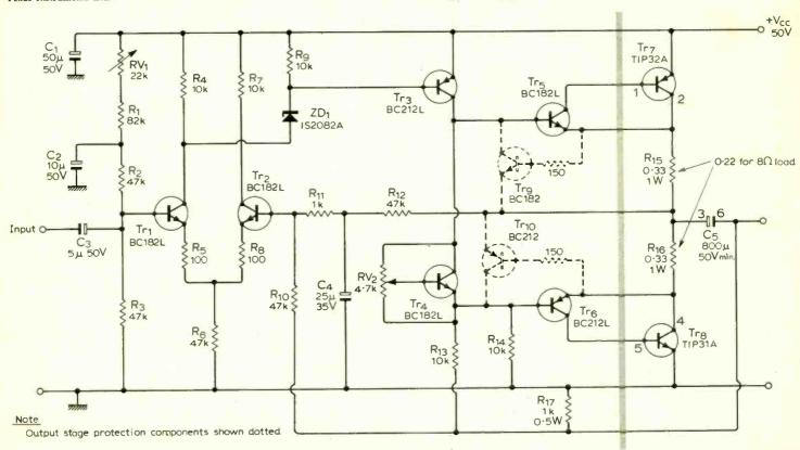
Fig.1 Amplifier circuit for driving resistive and inductive loads of 15  $\Omega$  or  $8\Omega$
