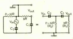
Fig. 7. Here the basic 2nd-order CR network is connected to give high-pass response.
