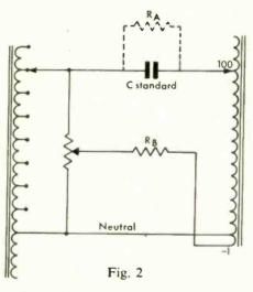
RA is the resistive term associated with the power factor of the standard capacitor. A fixed resistor RB is connected to balance the current produced in the right hand transformer by RA and an exact balance can be made by means of the potentiometer connected across the left hand transformer winding forming a potential divider.
