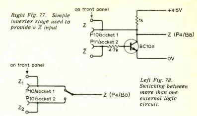
will then have the output  $Z_1$ . In other words the display will show the function external circuit one performs.  $S_1$  (b) has no effect because it is in series with  $S_2$  (b) which is open.
