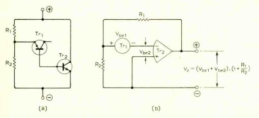
Fig. 3. Active zener with multiplied Vz and the equivalent circuit (b).
