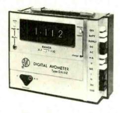
tinuous operation. The meter may also be operated from a 12V car battery. The measured value is presented on a 3½ digit display with automatic decimal point and over-range indication. A print-out socket (parallel BCD 1248 code) is available as an optional extra. Avo Ltd, Avocet House, Dover, Kent.
