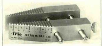
An easily adjusted hand tool for the accurate bending of resistor, capacitor, diode leads, etc., for printed circuits. Will bend leads to within  $\frac{1}{16}$ " of ends of components and
