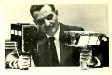
The two television cameras used on the mission: left, the colour camera carried in the command module to televise activities in flight; right, the black-and-white camera carried in the lunar module and used to televise scenes on the surface of the moon.
