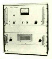
input levels. The units may be operated either locally, with or without extended control; or remotely controlled without switching. Illustrated is the 125ZA 50W output unit with receiver and remote control panel fitted to the same cabinet. The equipment panels fit standard 483mm (19 inch) racks, if required. Park Air Electronics Ltd, Red Lion Square, Stamford, Lincs.
