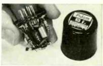
£20/19/0 (normally E1 (Bistable) module shows B9A base for ease of connection. Pins 7, 8, 9 are always power connections.
